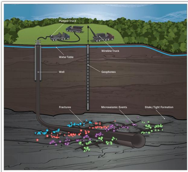
Figure 2: Hydraulic fracture schematic overview [1].
