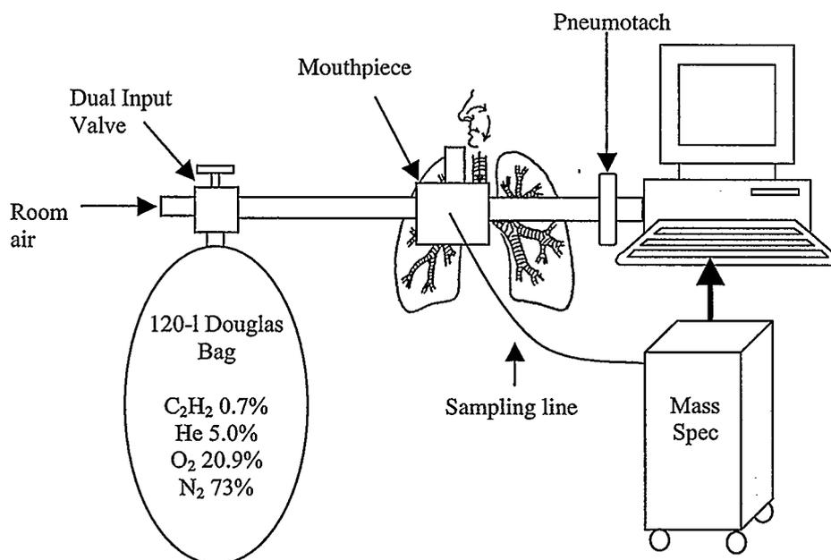
**Figure 9.** Setup for open-circuit acetylene uptake.
