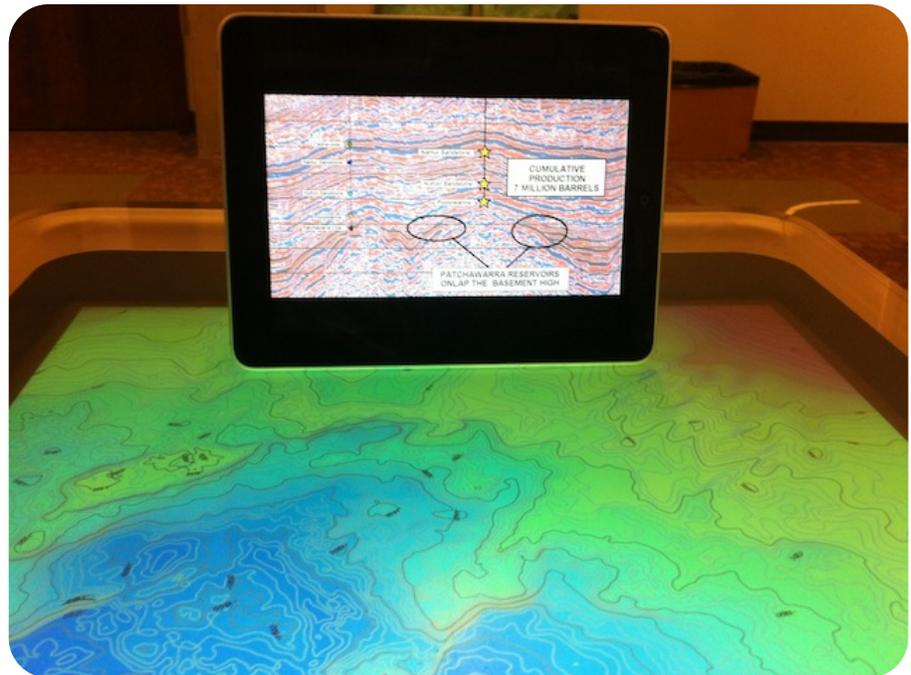
based maps with multi-touch tabletops. This allows a user to pan and zoom through the microseep data and make choices about what types of data to visualize. In addition, we employ a consumer tablet to visualize seismic data in a manner such that the vertical orientation of the data is preserved. When a user places the tablet down on
