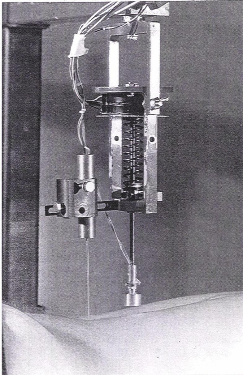
All of the electronic components of the TSM are housed in a rigid support framework that suspends the components over the tissue to be tested. This framework has been designed to allow the spindle to be easily positioned in three dimensional space, allowing for stiffness measurements to be taken at any spindle/tissue contact angle.
