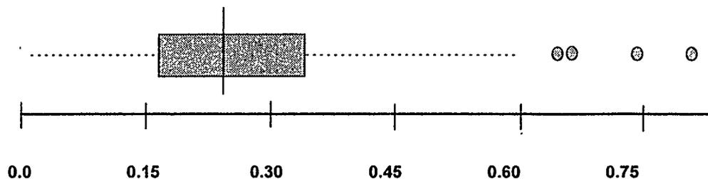
Figure 2. Boxplot distribution of the ICCs generated for 20 surface force groups. The shaded box represents the range of the data's second and third quartiles (interquartile range, IQR) which is transected by a vertical line representing the median of the data. Dashed lines represent the IQR multiplied by 1.5. Values falling outside the range of the dashed lines are considered to be outliers and are represented by circles.
