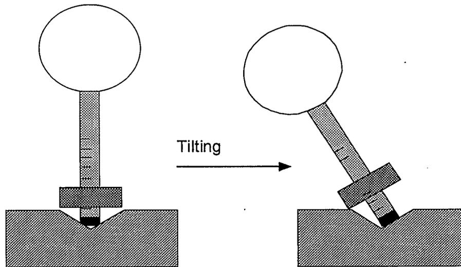
Figure 5. Under-estimation of tissue deformation caused by “submarining”.
