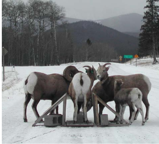
Figure 2. A photograph of sheep gathering around the freestanding platform scale. One sheep is standing between the barriers, with all four feet on the scale.
