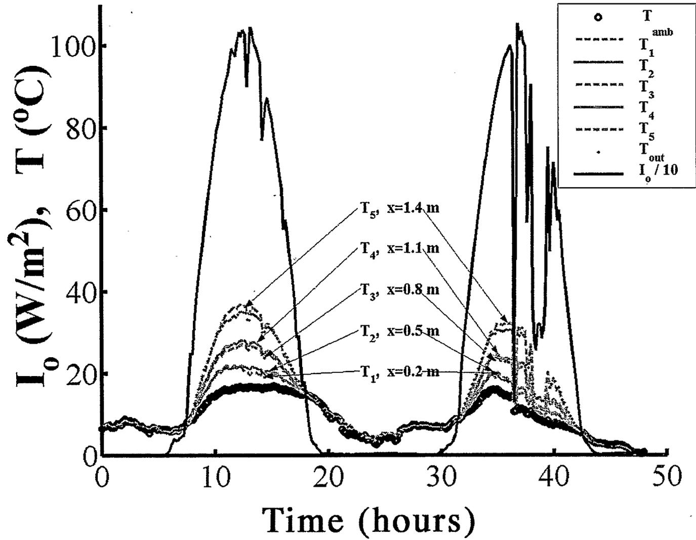
Figure 5.4 Porous Bed Temperature Distribution with 73.78 L/s Airflow
