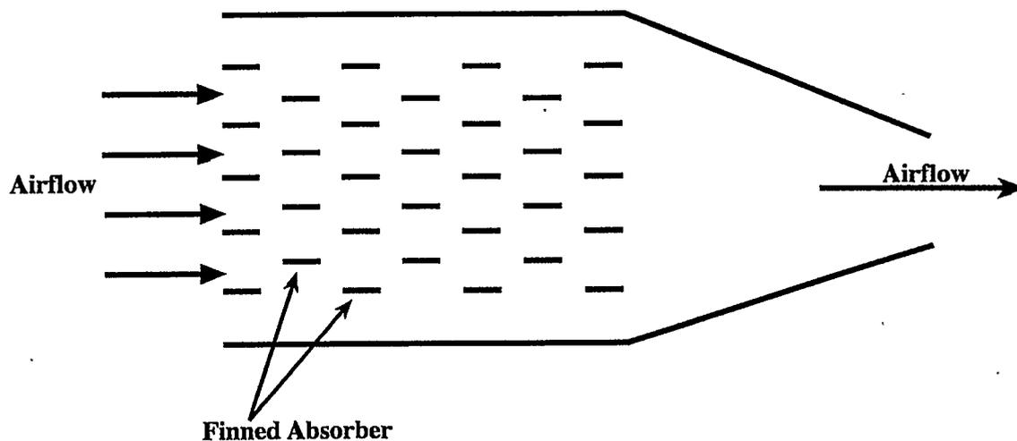
Figure 2.2 Staggered Parallel Flow Fins (top view)
