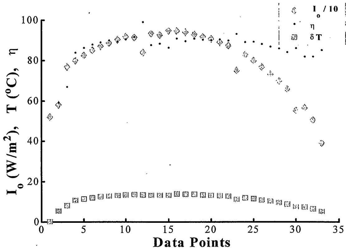
Figure 5.22 Collector Efficiency: One Glass Cover & Porous Media, with airflow rate of 73.78 L/s
