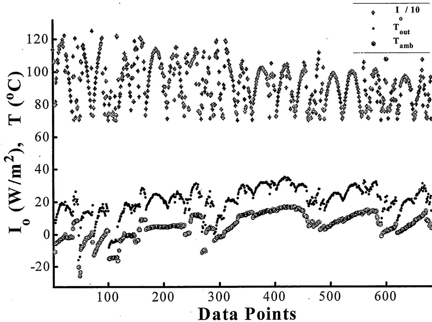
Figure 5.15 Collector Outlet Air Temperature compared to Ambient Air Temperature with Solar Intensity  $> 700 W/m^2$ , for airflow rate of 73.78 L/s
