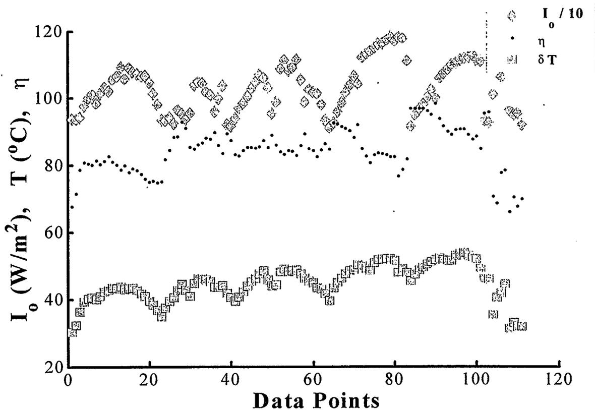
Figure 5.12 Collector Thermal Efficiency with Solar Intensity  $> 900 \text{ W/m}^2$ , with 31.21 L/s Airflow
