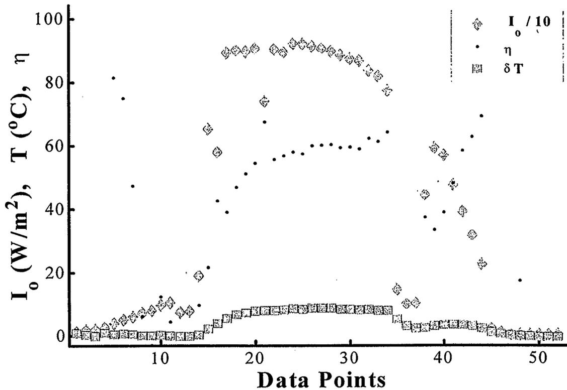
**Figure 5.24 Conventional Collector Efficiency: One Glass Cover & No Porous Media, with airflow rate of 73.78 L/s**
