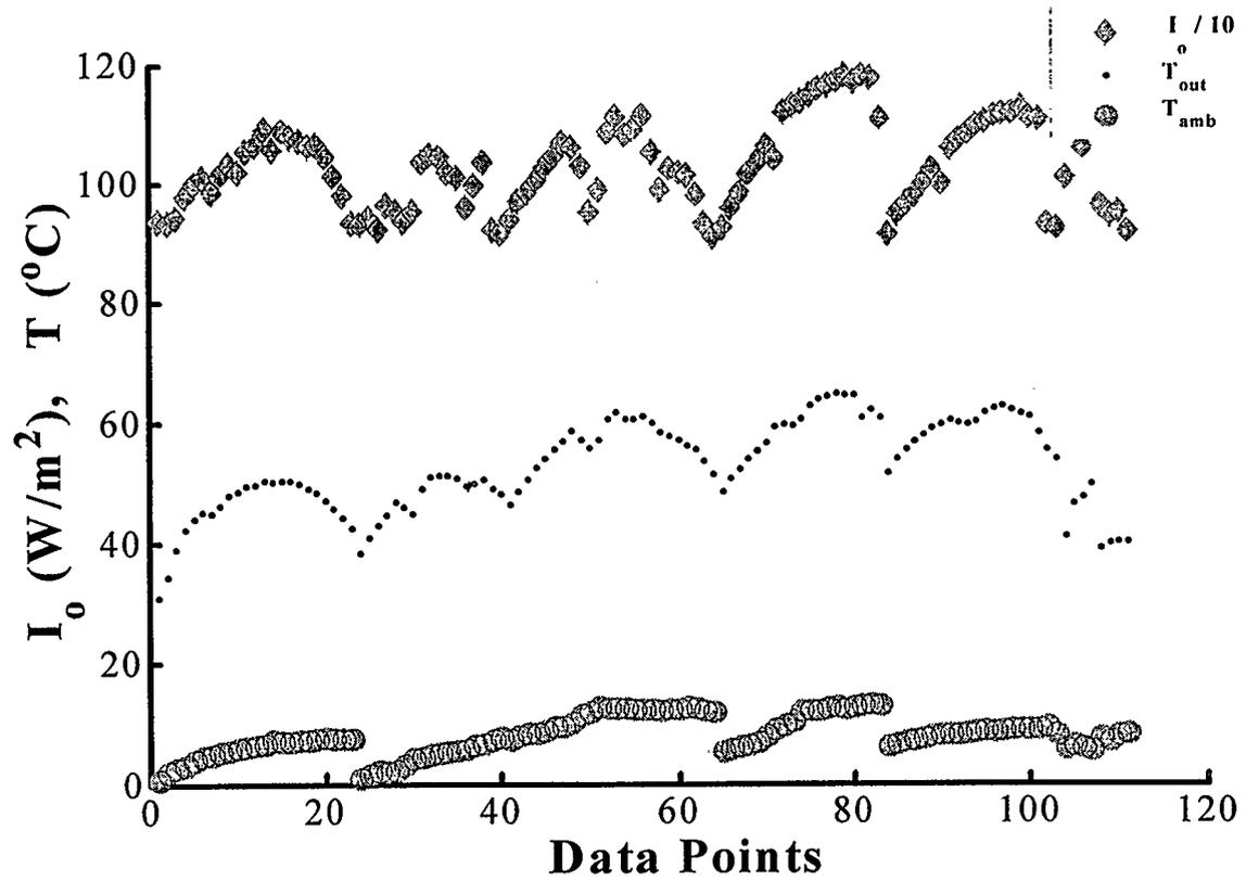
**Figure 5.8 Collector Outlet Air Temperature compared to Ambient Air Temperature with Solar**
