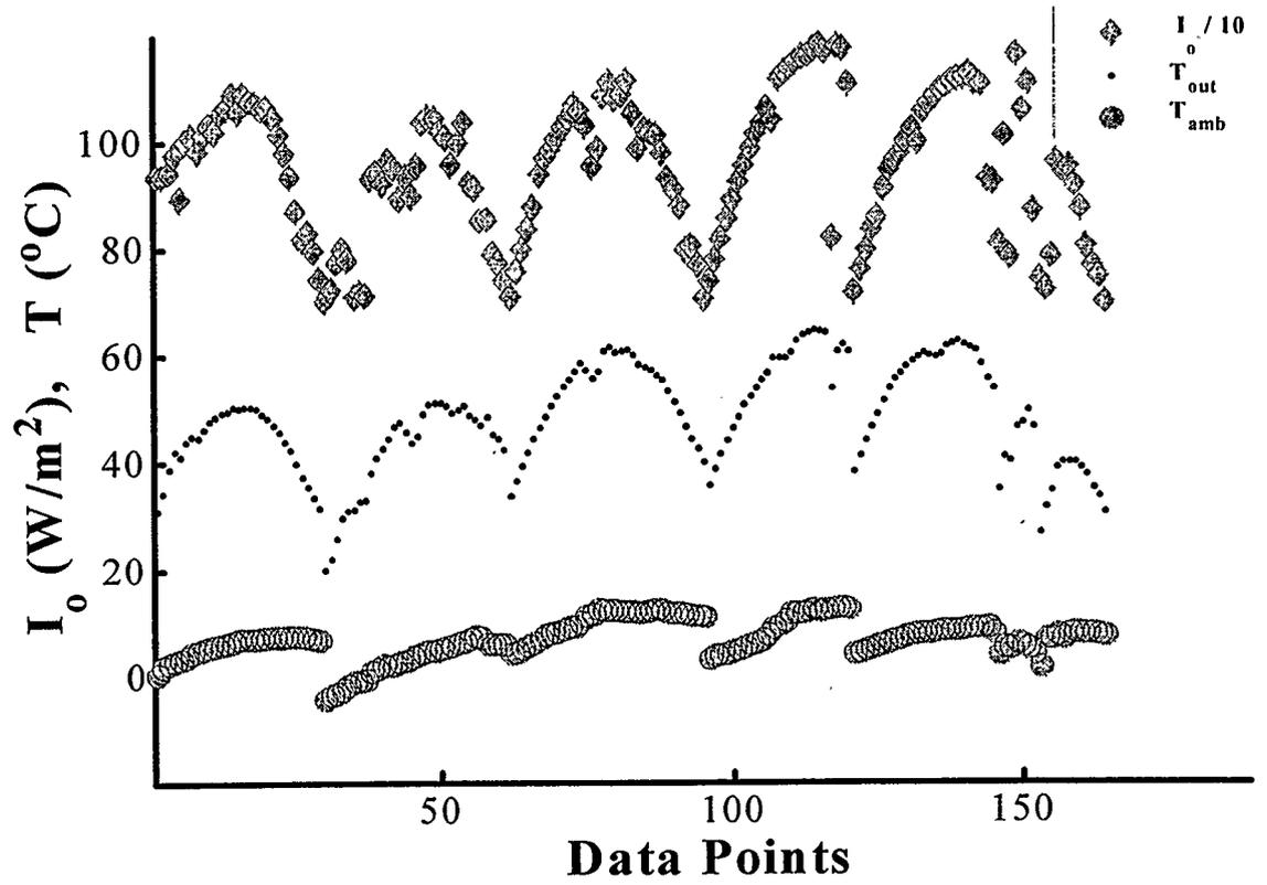
Figure 5.7 Collector Outlet Air Temperature compared to Ambient Air Temperature with Solar Intensity  $> 700 \text{ W}/\text{m}^2$ , for airflow rate of  $31.21 \text{ L}/\text{s}$
