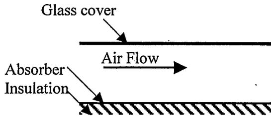
**A. Conventional Collector, with air flowing over absorber**
