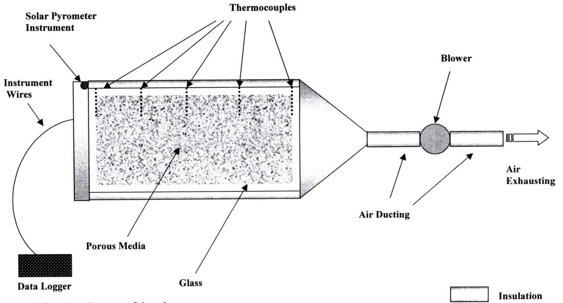
Figure 3.2 Experimental Apparatus Schematic
