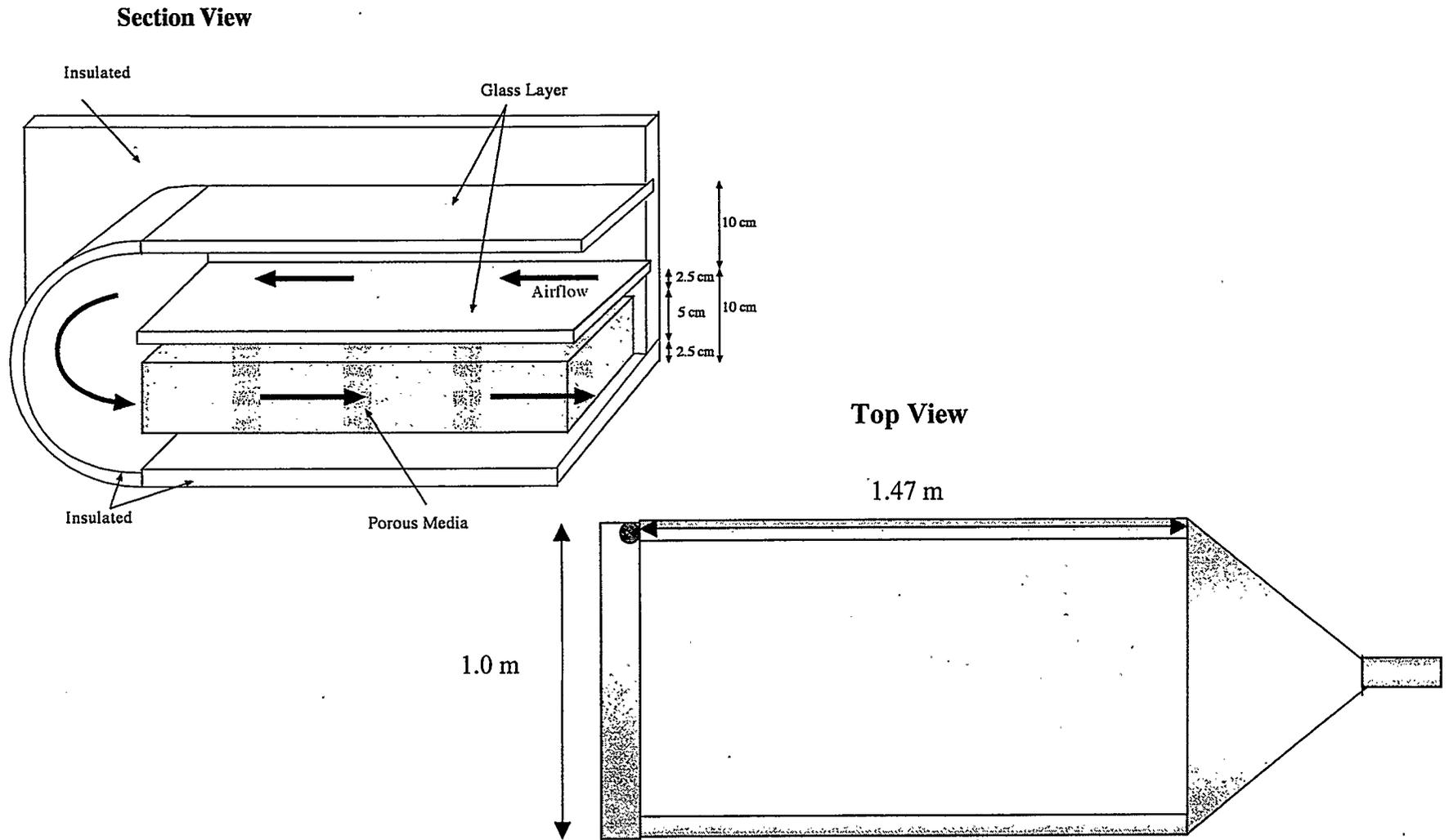
Figure 3.1 Schematic of Present Solar Air Heating Collector
