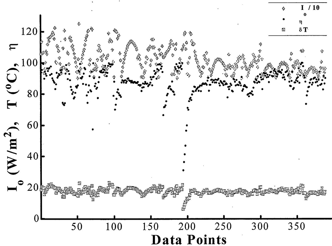
Figure 5.20 Collector Thermal Efficiency with Solar Intensity  $> 900 W/m^2$ , for airflow rate of 73.78 L/s
