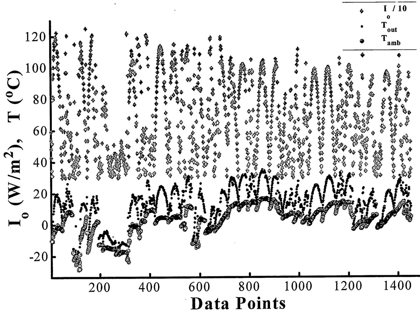
Figure 5.13 Collector Outlet Air Temperature compared to Ambient Air Temperature with Solar Intensity > 300 W/m<sup>2</sup>, for airflow rate of 73.78 L/s
