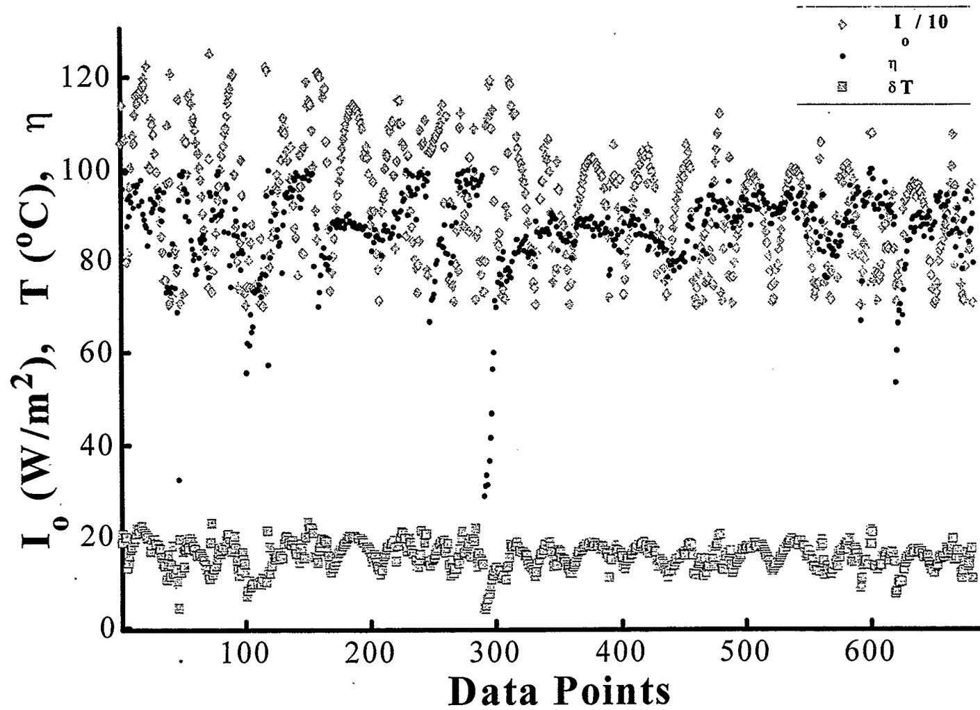
Figure 5.19 Collector Thermal Efficiency with Solar Intensity  $> 700 W/m^2$ , for airflow rate of 73.78 L/s
