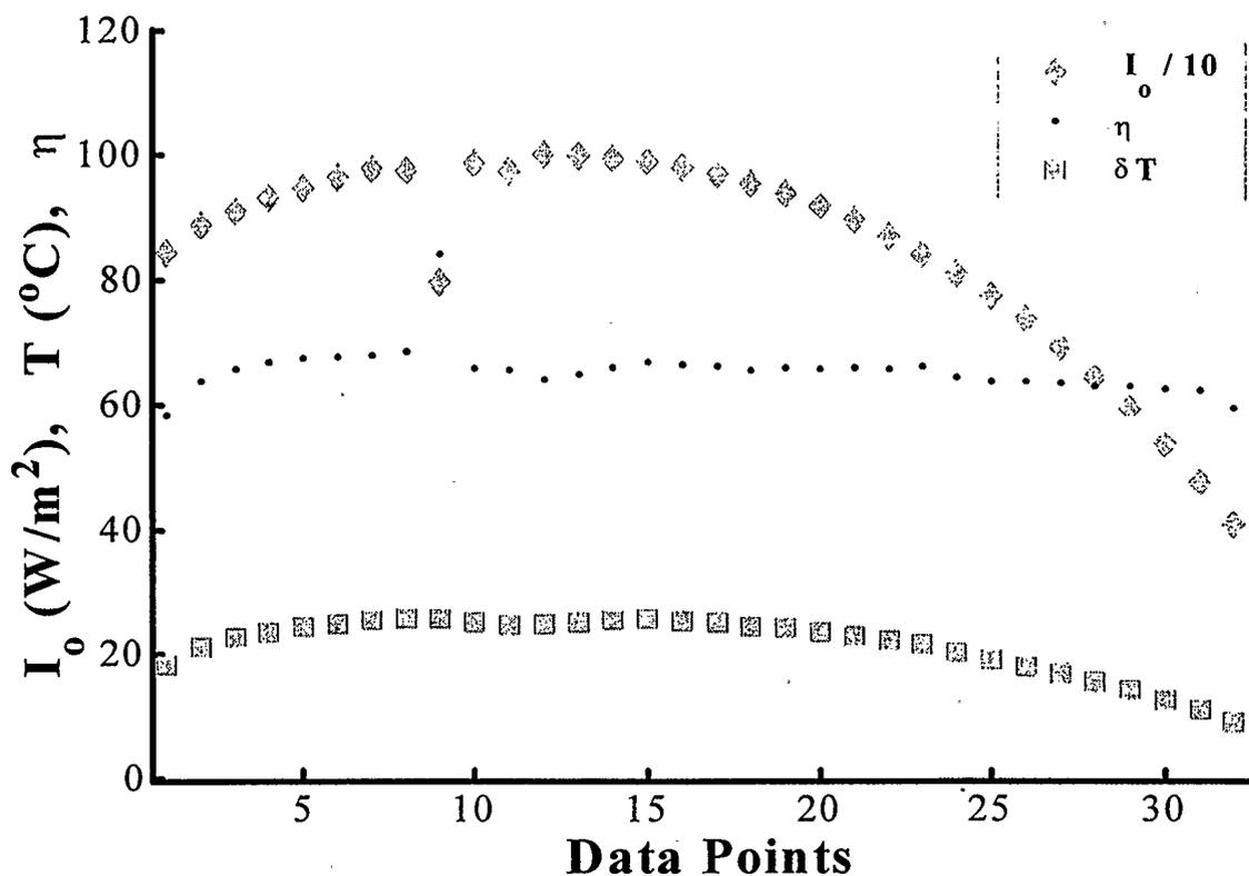
Figure 5.21 Collector Efficiency: One Glass Cover & Porous Media, with airflow rate of 31.21 L/s
