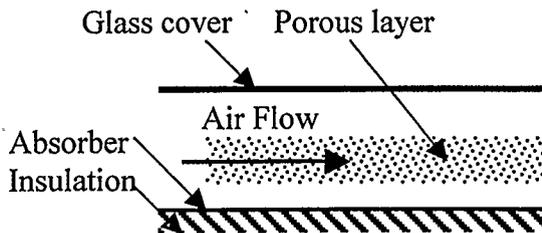
**E. Porous Matrix Absorber Collector**
