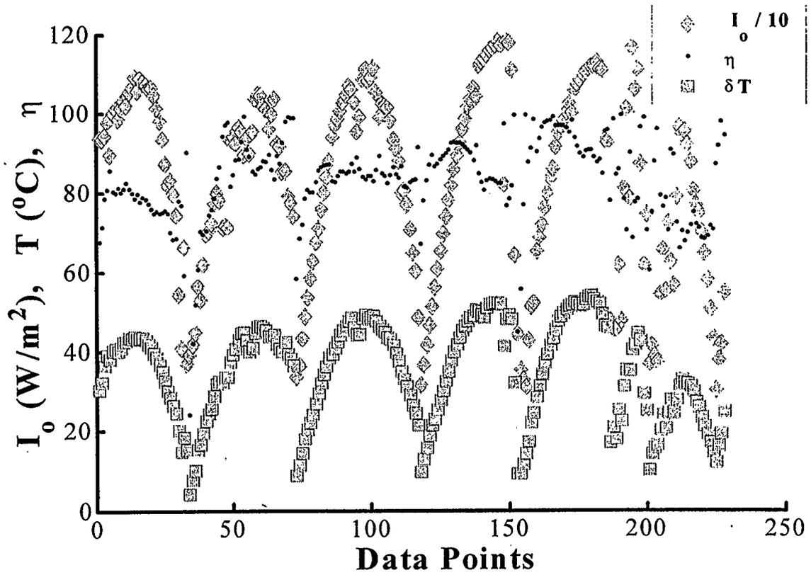
Figure 5.9 Collector Thermal Efficiency with Solar Intensity  $> 300 W/m^2$ , with 31.21 L/s Airflow
