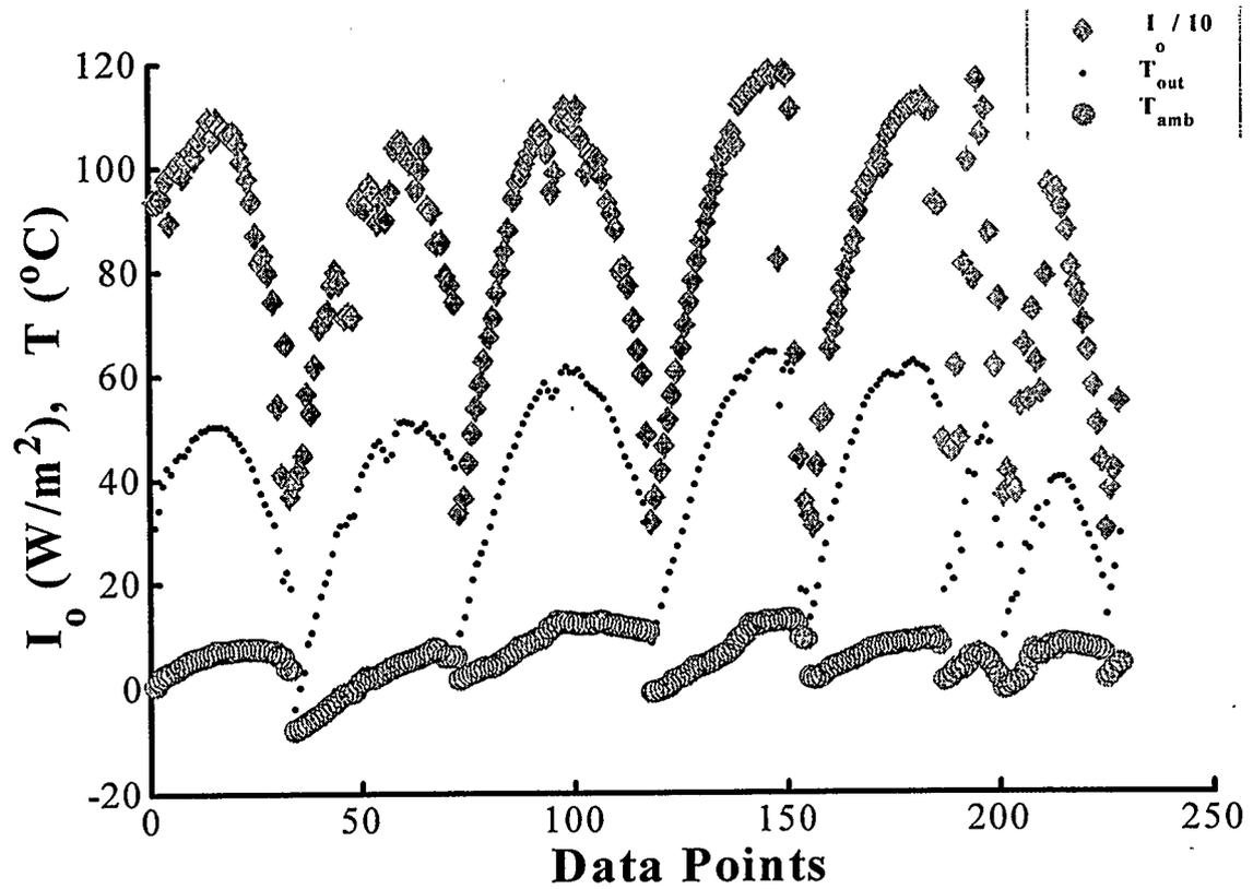
Figure 5.5 Collector Outlet Air Temperature compared to Ambient Air Temperature with Solar Intensity  $> 300 W/m^2$ , for airflow rate of 31.21 L/s
