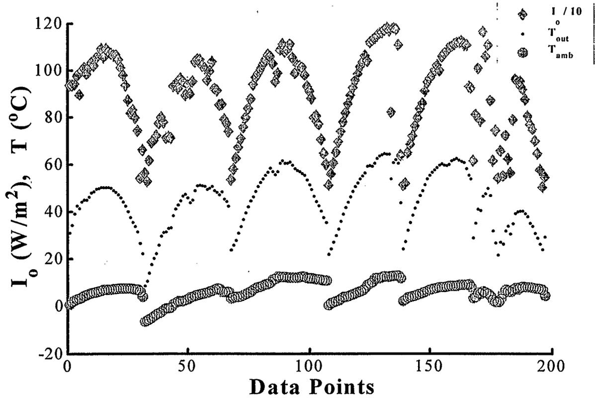
Figure 5.6 Collector Outlet Air Temperature compared to Ambient Air Temperature with Solar
