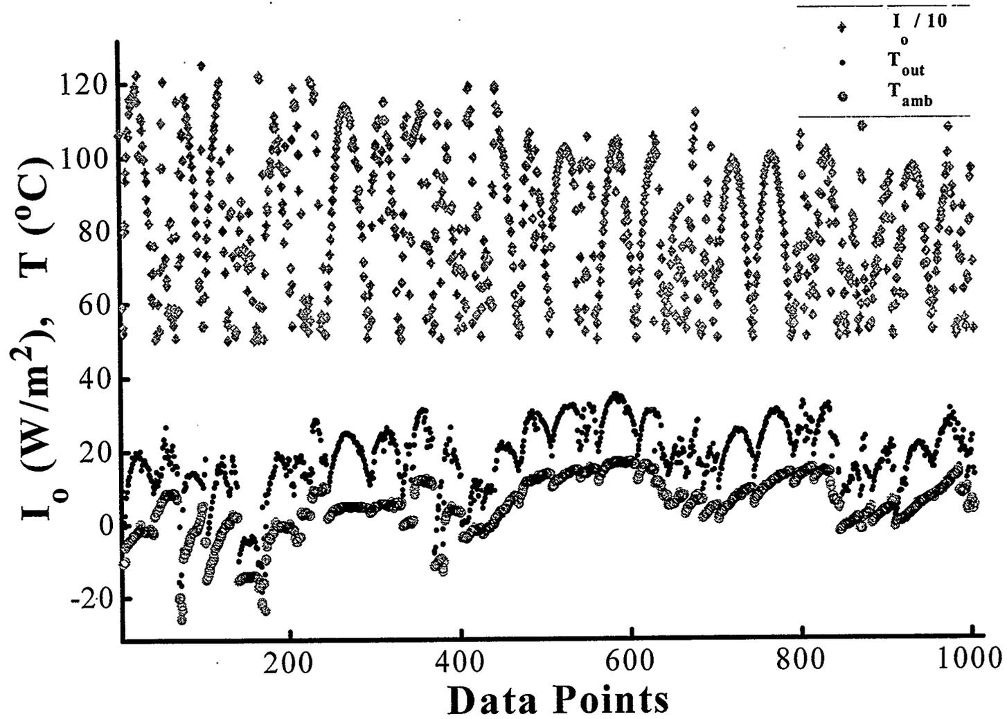
Figure 5.14 Collector Outlet Air Temperature compared to Ambient Air Temperature with Solar Intensity  $> 500 \text{ W}/\text{m}^2$ , for airflow rate of  $73.78 \text{ L}/\text{s}$
