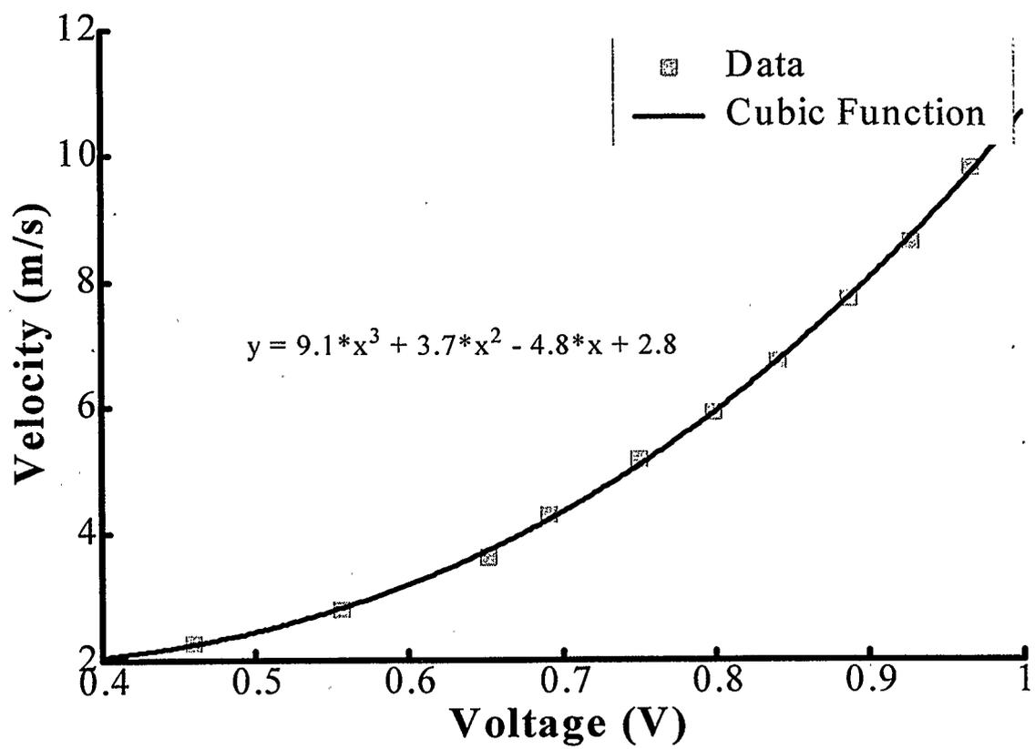
Figure 3.5 Calibration of Hot Wire Anemometer
