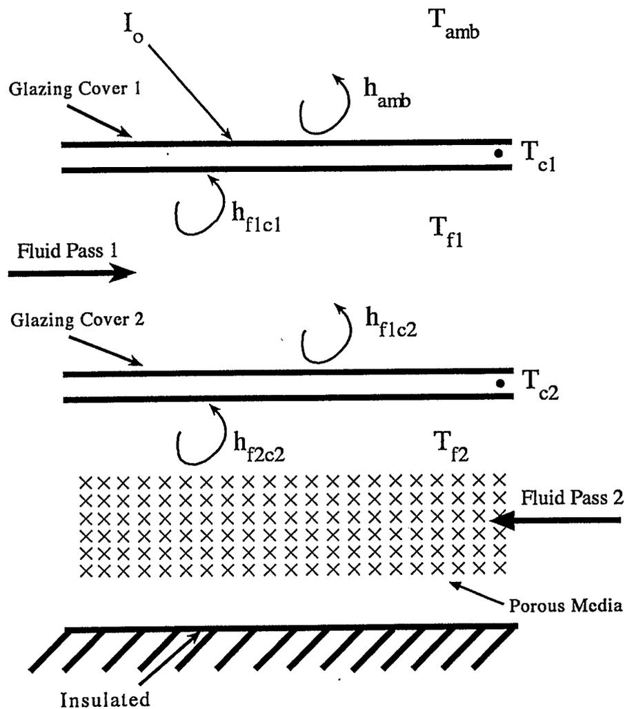
**Figure 4.2** Analysis of Heat Transfer in Collector
