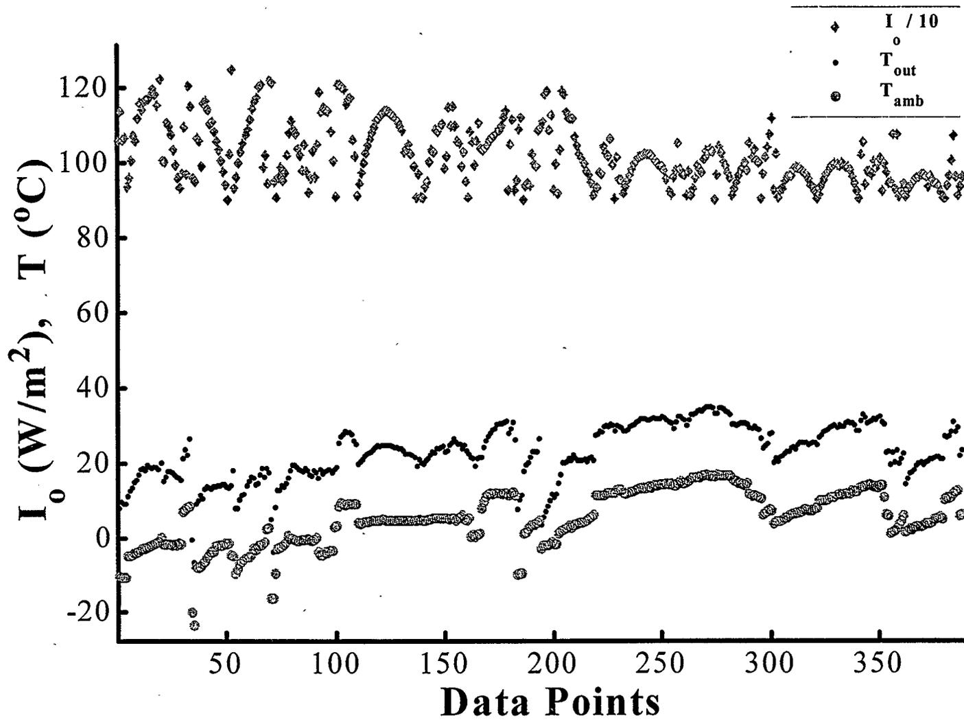
Figure 5.16 Collector Outlet Air Temperature compared to Ambient Air Temperature with Solar Intensity > 900 W/m<sup>2</sup>, for airflow rate of 73.78 L/s
