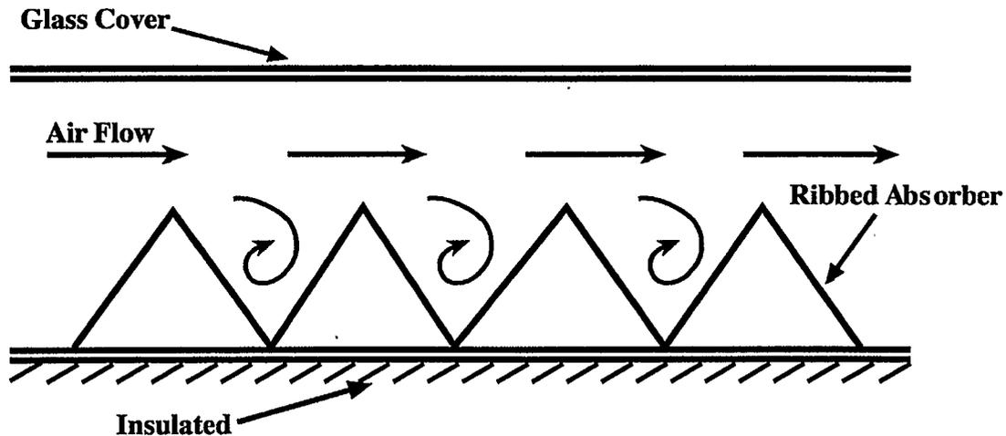
Figure 2.1 Flow Separation Through Ribbed Collectors
