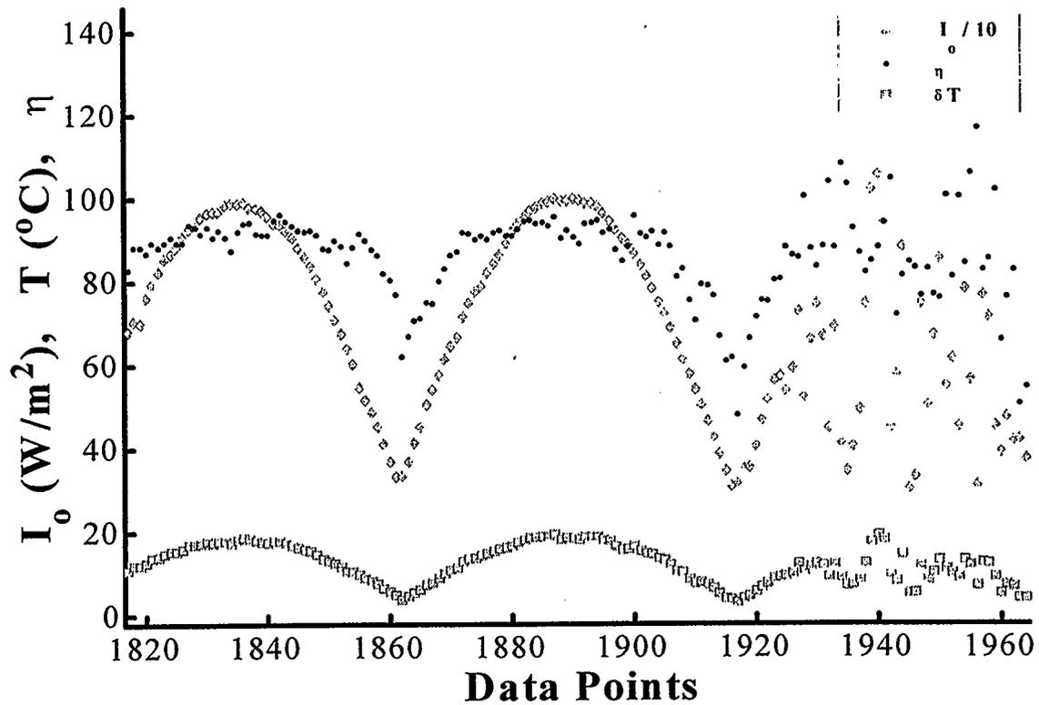
**Figure 5.2** Unsteady State Performance of Collector, for airflow of 73.78 L/s
