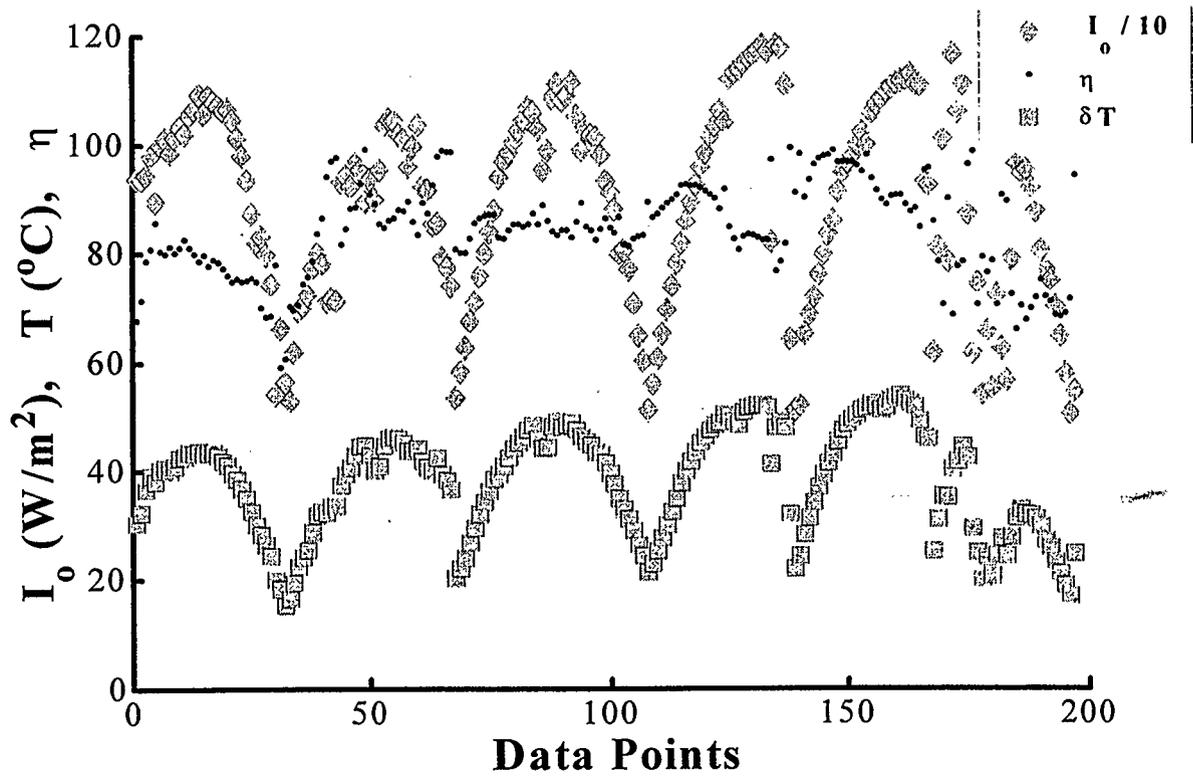
Figure 5.10 Collector Thermal Efficiency with Solar Intensity  $> 500 \text{ W/m}^2$ , with 31.21 L/s Airflow
