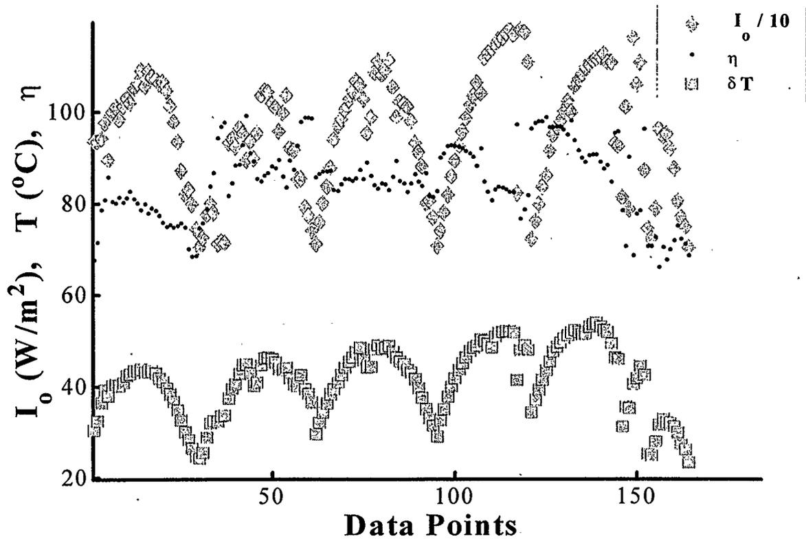
Figure 5.11 Collector Thermal Efficiency with Solar Intensity  $> 700 W/m^2$ , with 31.21 L/s Airflow
