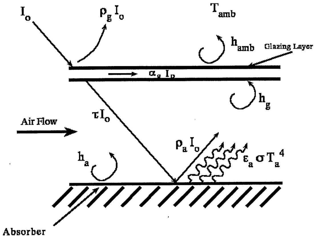
Figure 4.1 Schematic Diagram of Energy Balance in Solar Collector
