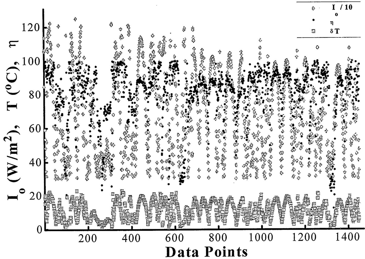
Figure 5.17 Collector Thermal Efficiency with Solar Intensity > 300 W/m<sup>2</sup>, for airflow rate of 73.78 L/s
