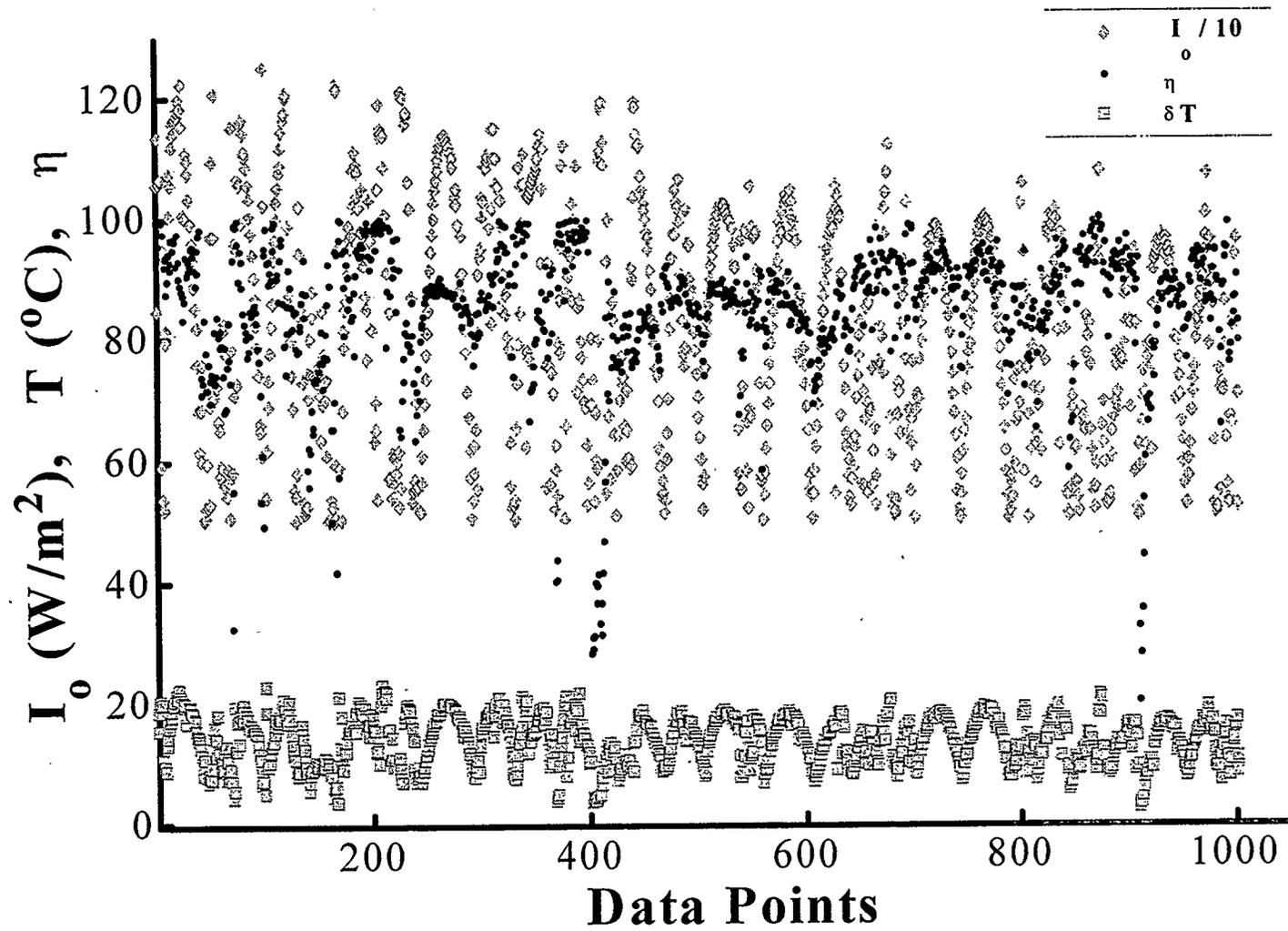
Figure 5.18 Collector Thermal Efficiency with Solar Intensity  $> 500 W/m^2$ , for airflow rate of 73.78 L/s
