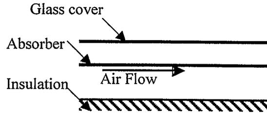
**B. Conventional Collector, with air flowing under absorber**
