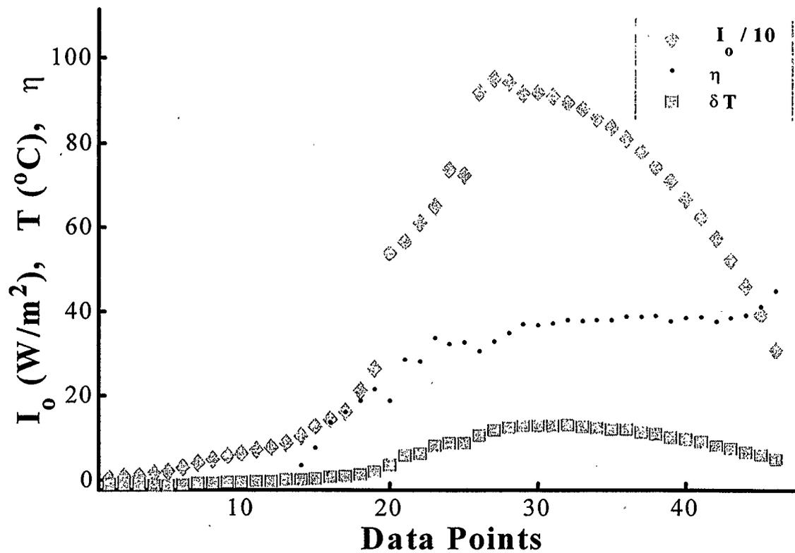
**Figure 5.23 Conventional Collector Efficiency: One Glass Cover & No Porous Media, with airflow rate of 31.21 L/s**
