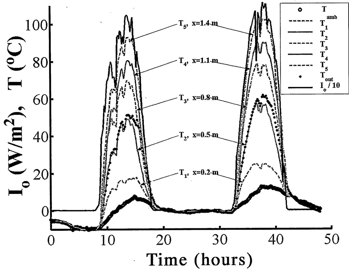
Figure 5.3 Porous Bed Temperature Distribution with 31.21 L/s Airflow
