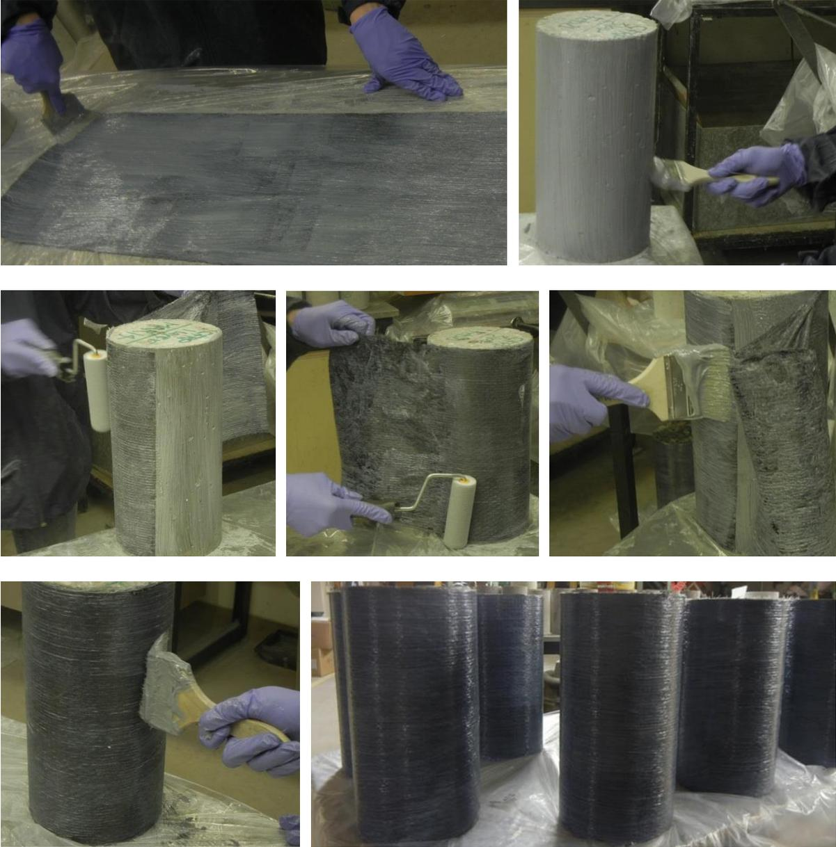
**Figure 3-6: Procedures for wrapping cylinders with CFRP sheets**
