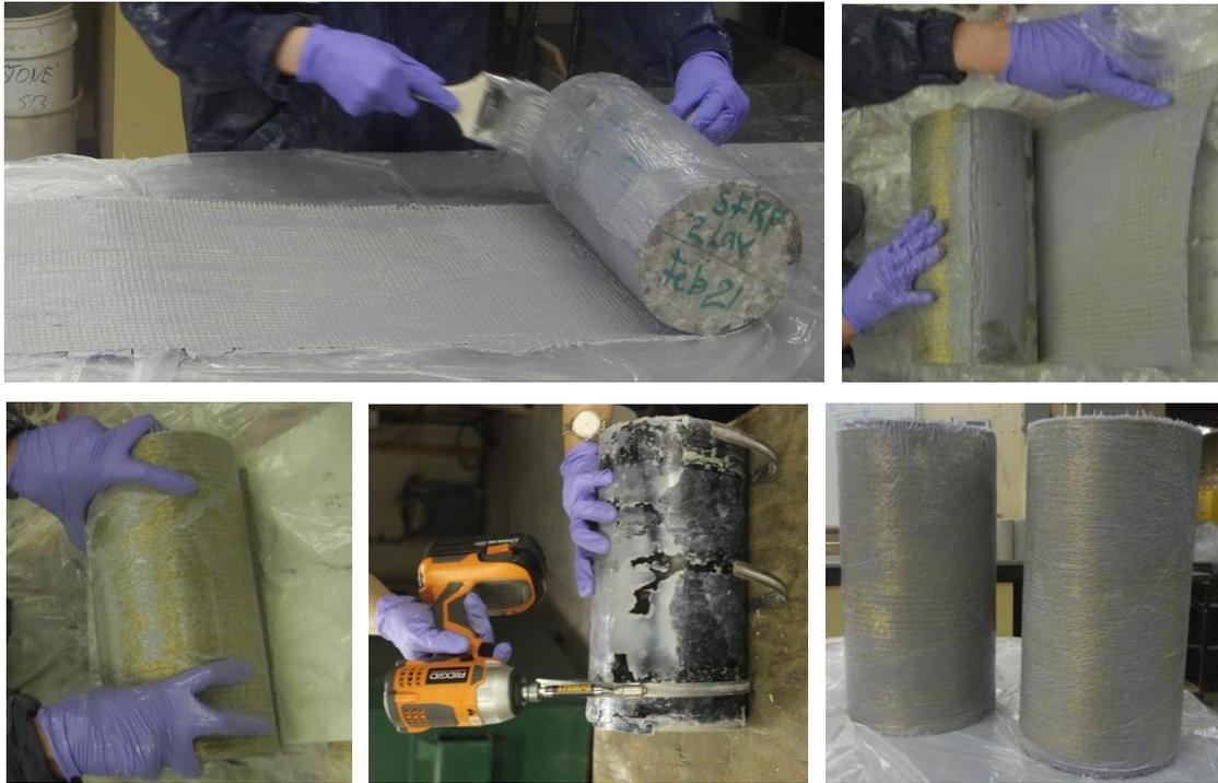
**Figure 3-7: Procedures for wrapping cylinders with SFRP sheet**
