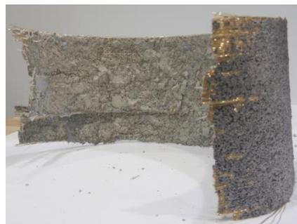
**Figure 4-5: SFRP sheet – concrete interface**
