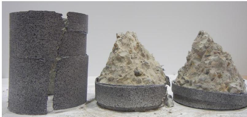
**Figure 4-2: Typical failure mode of CFRP-wrapped cylinders**
