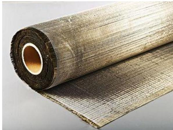
**Figure 2-6: Multi-directional basalt fabric, GBF.com (2015)**
