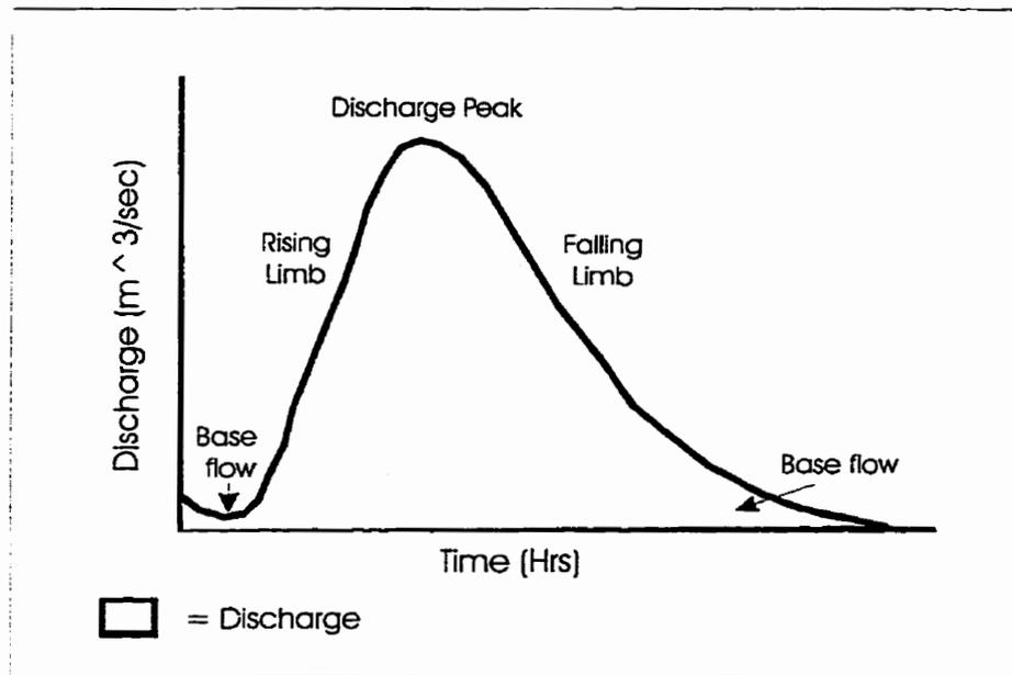
Figure 3.1: The Discharge Hydrograph.
