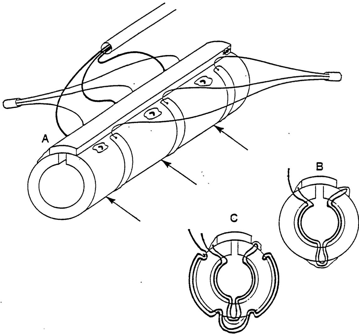
Figure 1. Vagal recording cuff electrode. The arrows in A point to the position of the electrodes within the cuff. A cross-sectional view is shown in B. External electrodes are shown in C.
