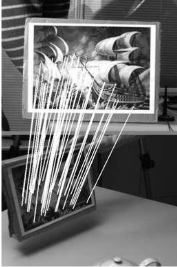
Figure 4. BazAR utilizes the Ferns algorithm to rapidly track surfaces without the need for fiduciary markers [20].
