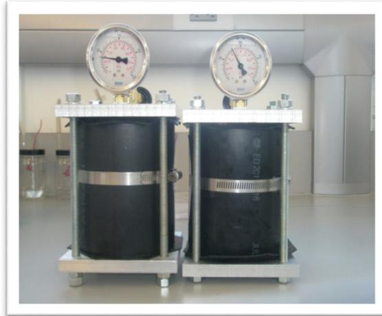
**Figure 4-1: Pressurized HDPE Pipe Samples**
