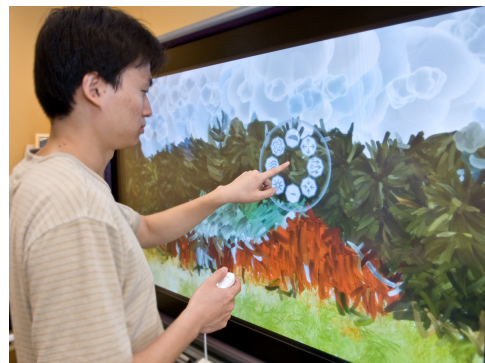
(b) Direct touch using SMART's DVIT.
