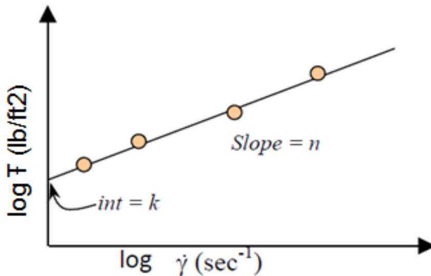
Figure 1.10: Log-Log Power Law fluid shear stress vs. shear rate (From Fracturing Fluid Main Functions, website)
