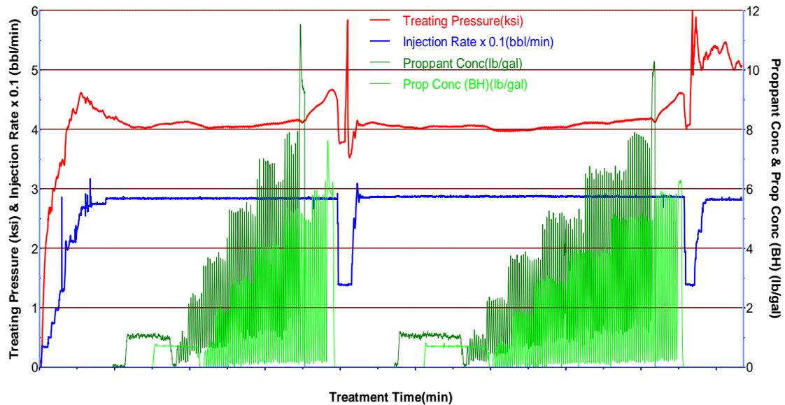
Figure 4.10: Cardium horizontal multiple stages channel fracturing treatment plot (Treatment data from Schlumberger fracturing job database). Note: Treatment time is hidden for confidentiality reason.
