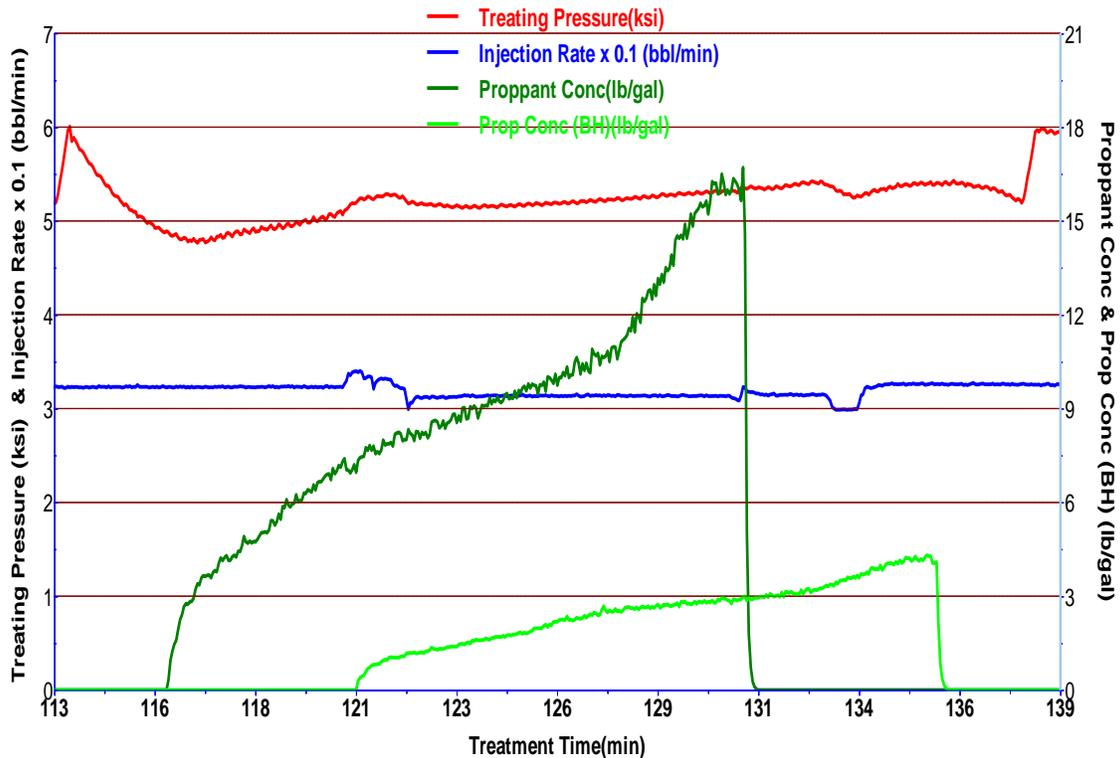
Figure 1.2: Continuously ramp-up proppant concentration illustration (Treatment data from Schlumberger fracturing job database)
