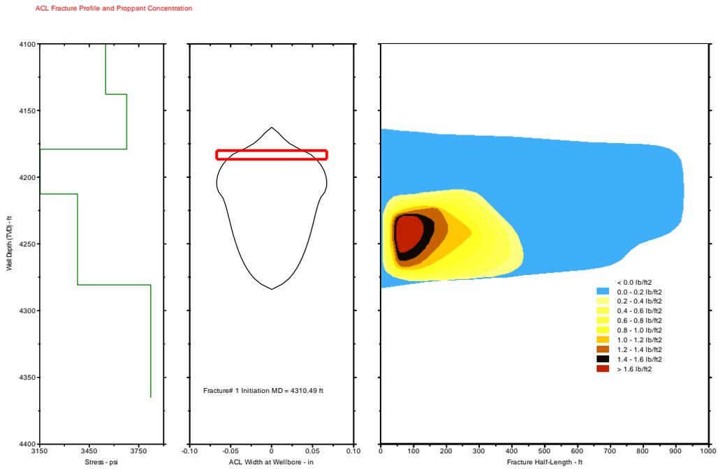
Figure 2.7: Low viscosity fluid with 2-D flow proppant distribution after closure
