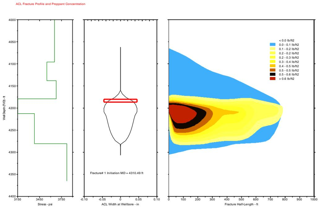
Figure 2.9: Medium viscosity fluid with 2-D flow proppant distribution after closure
