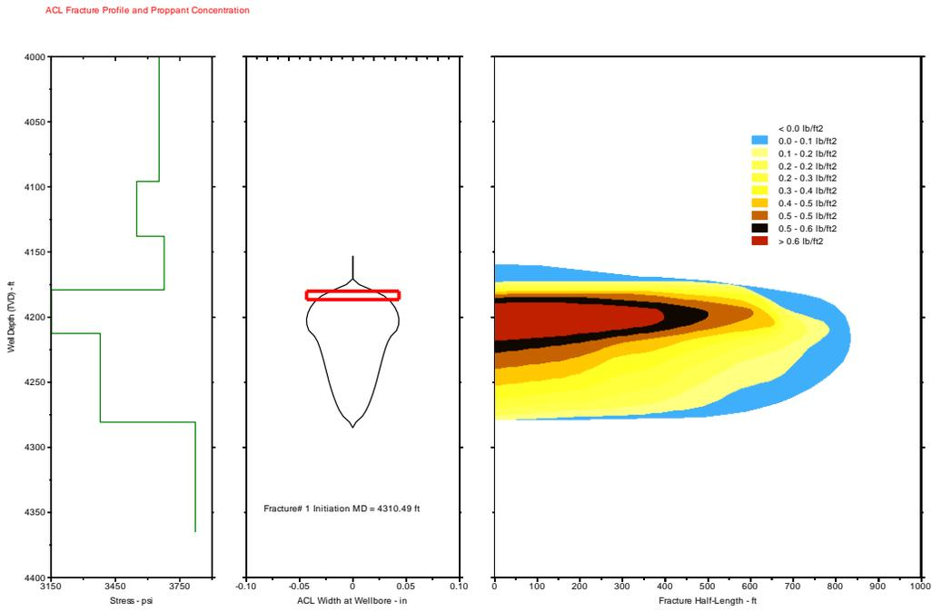
Figure 2.10: High viscosity fluid without 2-D flow proppant distribution after closure
