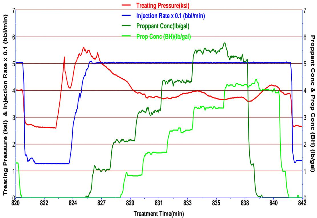
Figure 1.3: Stair step proppant concentration illustrations (Treatment data from Schlumberger fracturing job database)
