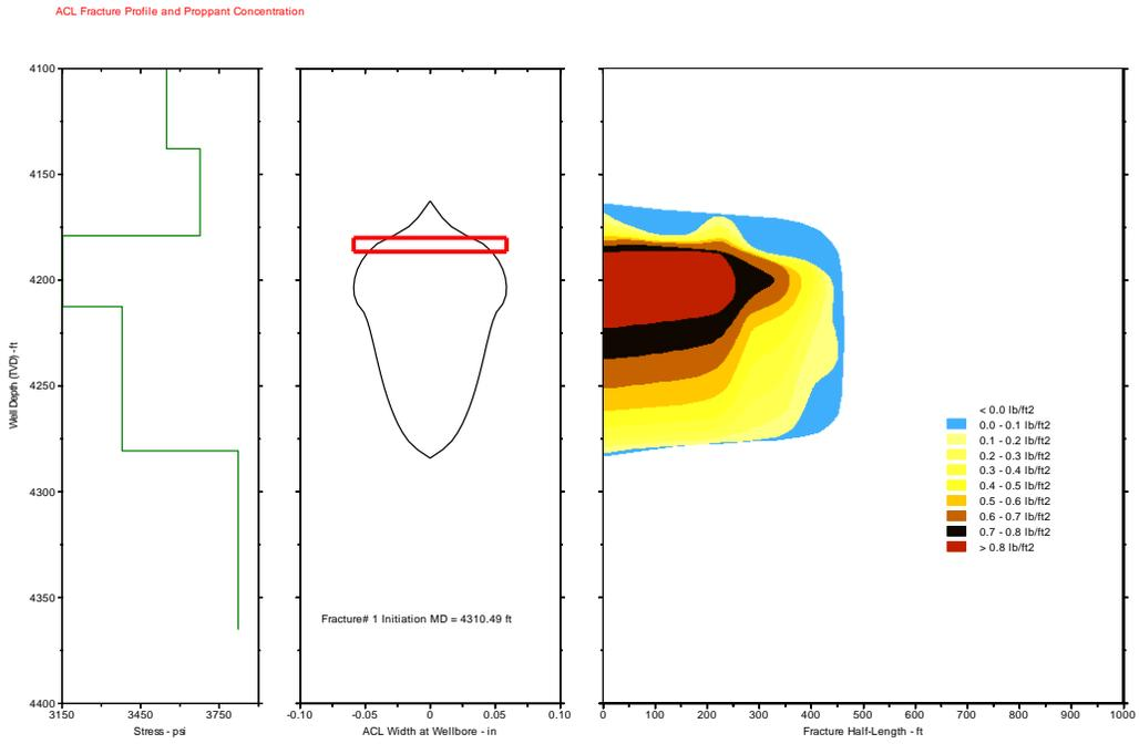
Figure 2.6: Low viscosity fluid without 2-D flow proppant distribution after closure
