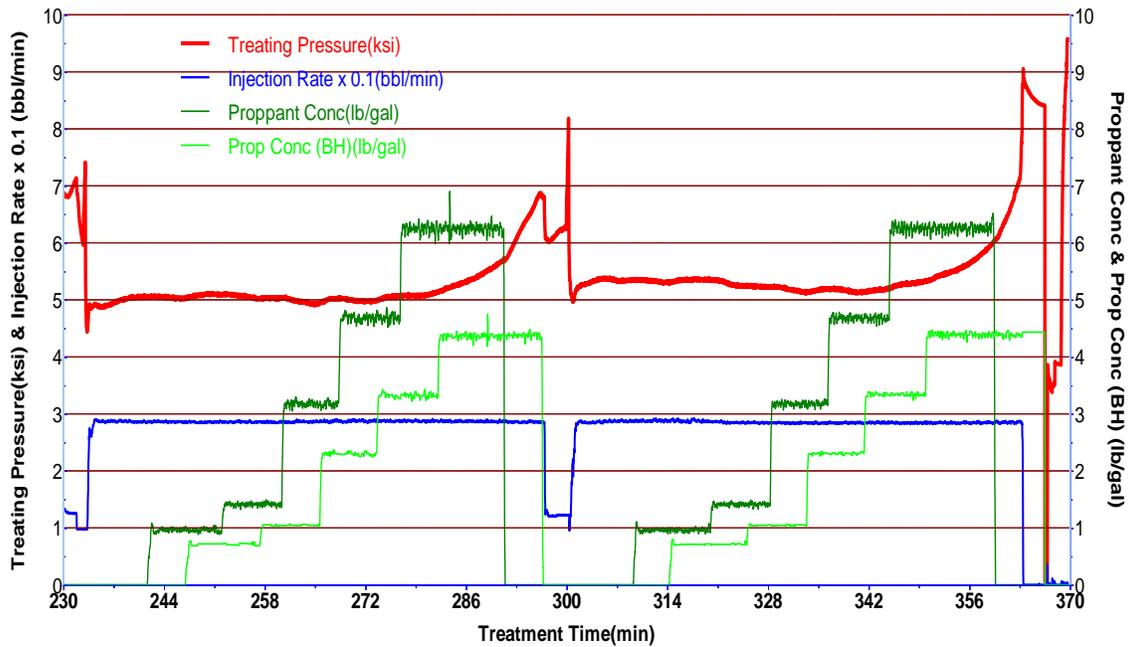
Figure 4.9: Cardium horizontal multiple stages conventional fracturing treatment plot (Treatment data from Schlumberger fracturing job database)
