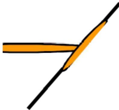
Figure 3.3: Hydraulic fracture opens the natural fracture and propagates along the natural fracture (From Keshavarzi, 2012)
