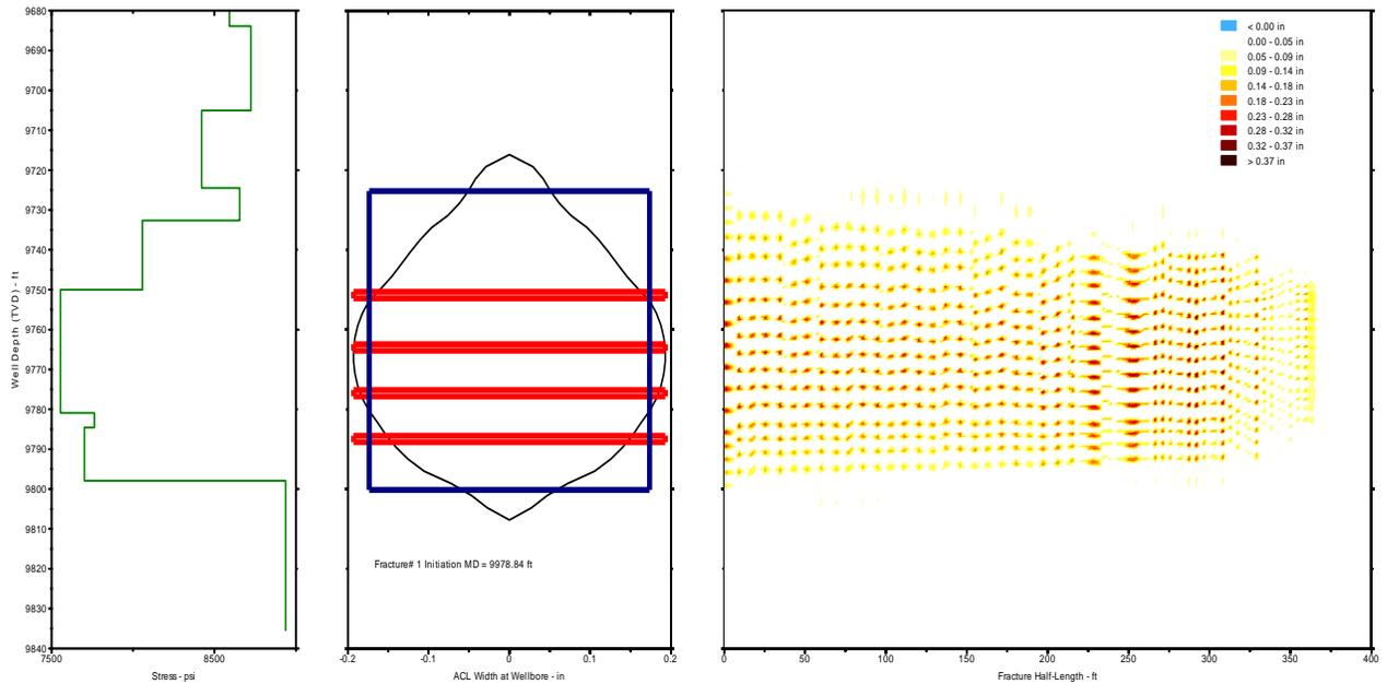
Figure 4.6: Channel fracturing geometry (By Schlumberger FracCADE simulator)
