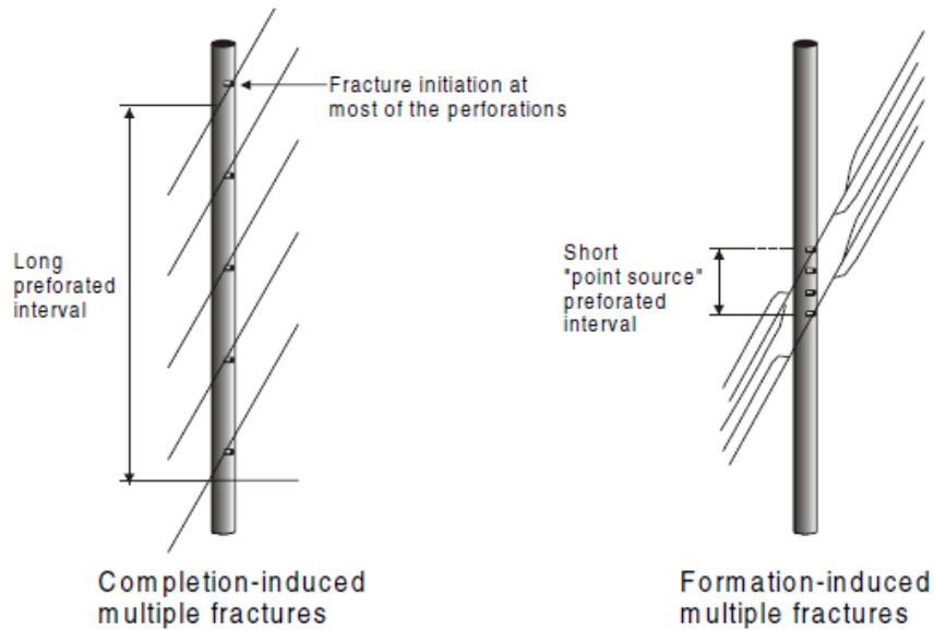
Figure 3.5: Cased-hole multiple hydraulic fractures: (left) A long perforated interval with numerous perforations can provide multiple fracture initiation points; (right) A naturally fractured formation can cause bifurcation of the hydraulic fractures as it intersects these natural fractures (From Weijers, et al., 2000).
