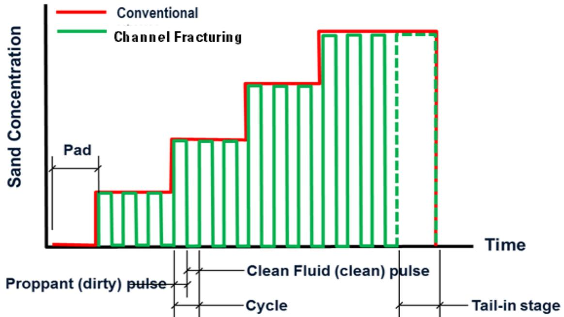
Figure 1.4: Channel fracturing proppant concentration illustrations (Courtesy of Schlumberger)
