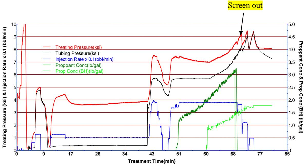
Figure 4.3: Wild River Cadomin formation screen out with 11,023 lbs pumped out of 88,185 lbs designed (Treatment data from Schlumberger fracturing job database)
