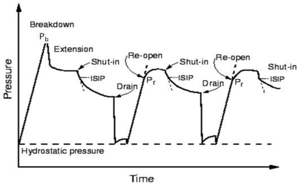
Figure 1.5: Pressure-time curve of a typical hydraulic fracturing experiment showing three pressurization cycles. The first cycle achieves a breakdown of the formation, whereas the two following cycles reopen the newly created fracture. During the shut-in phase the instantaneous shut-in pressure (ISIP), is observed which is identical to the least principal stress (From Brudy, 1995).
