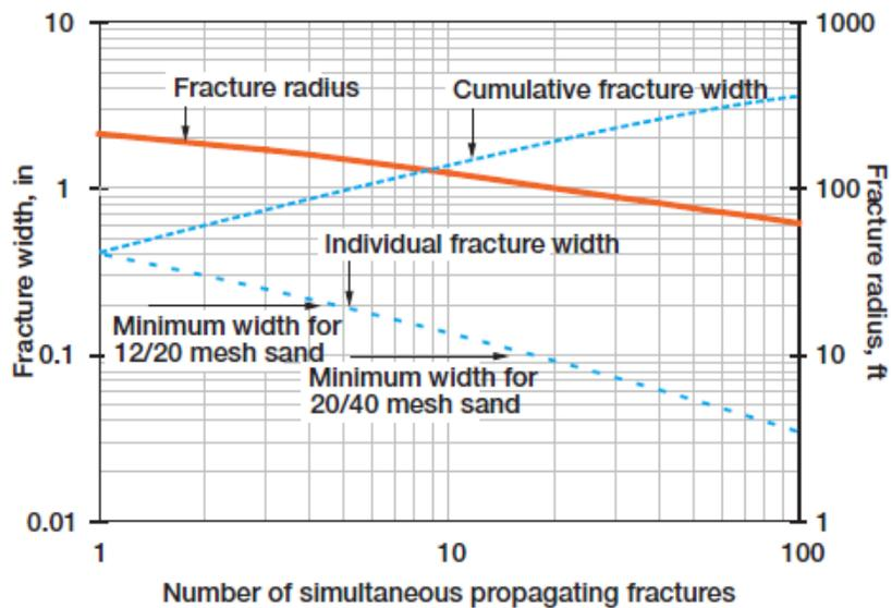
Figure 3.6: Change in individual fracture width, cumulative fracture width and fracture radius with a change in the equivalent number of simultaneous propagating multiple fractures (From Weijers, et al., 2000)
