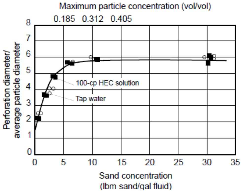
Figure 2.1: Proppant admittance through perforations (Gruesbeck and Collins, 1978)
