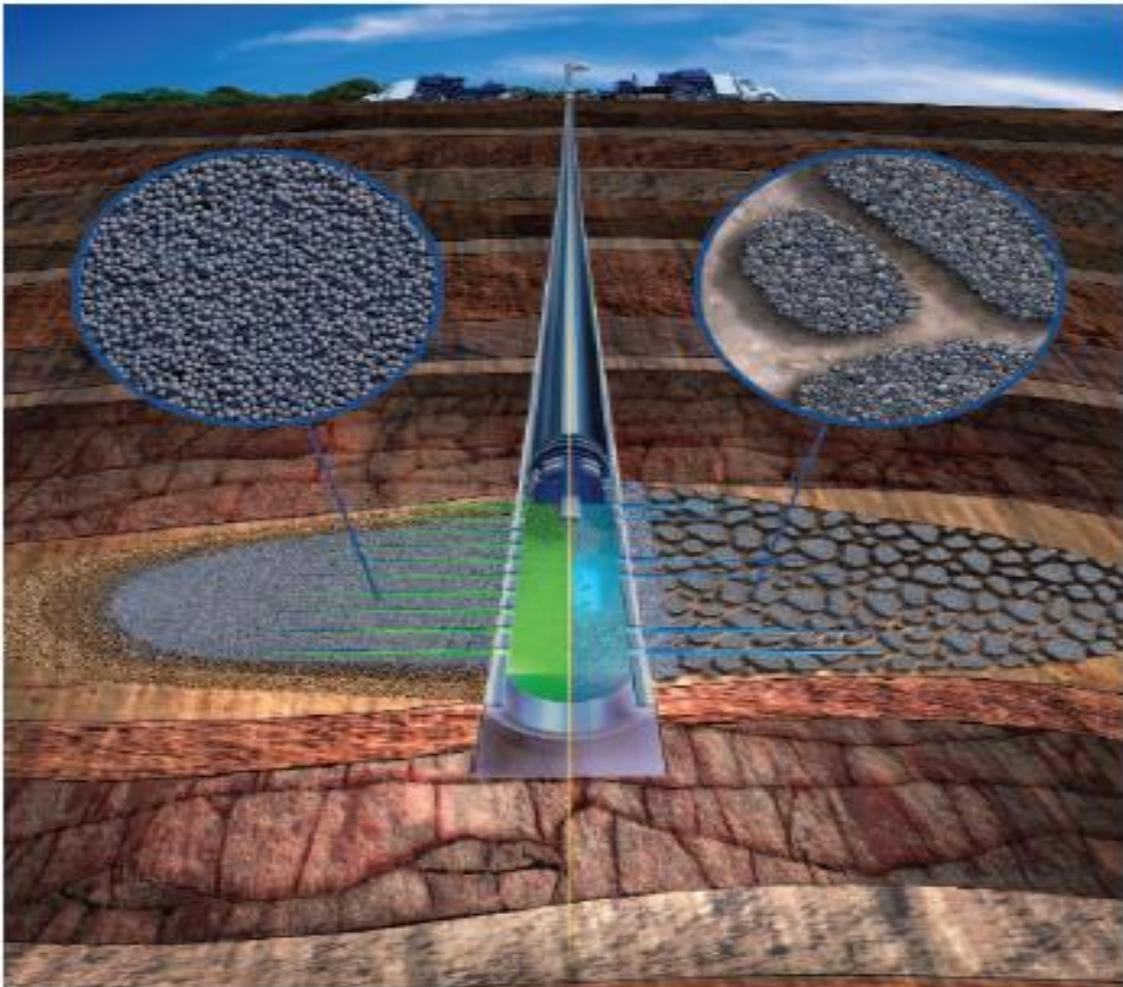
Figure 1.1: Conventional fracturing (left) and channel fracturing technique (right) (Courtesy of Schlumberger)
