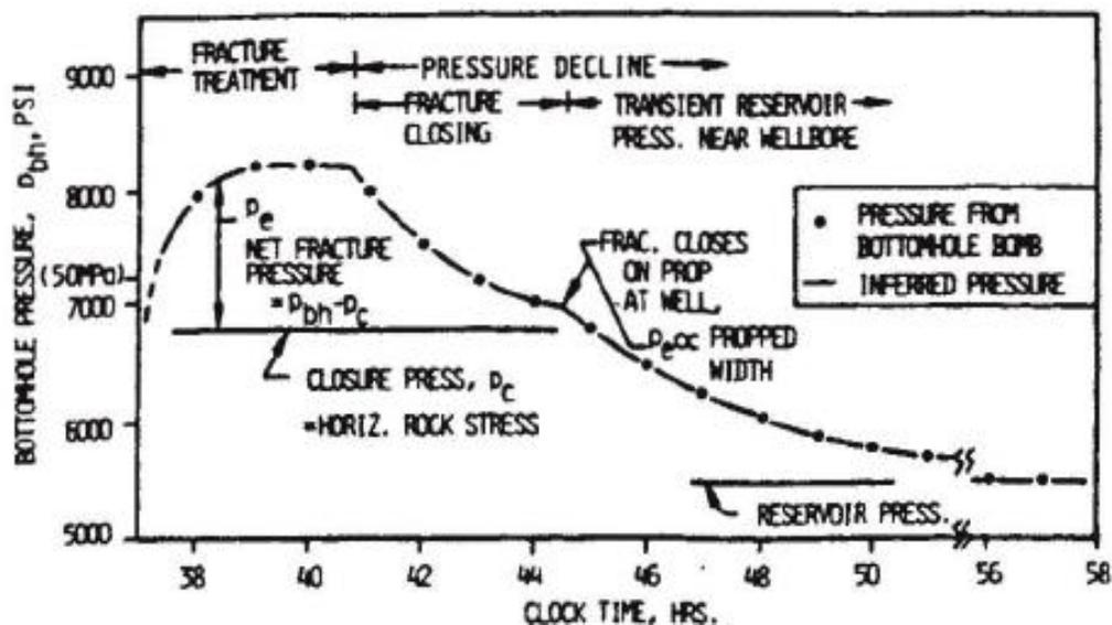
Figure 1.7: Example of fracturing-related pressures (Nolte, 1988)
