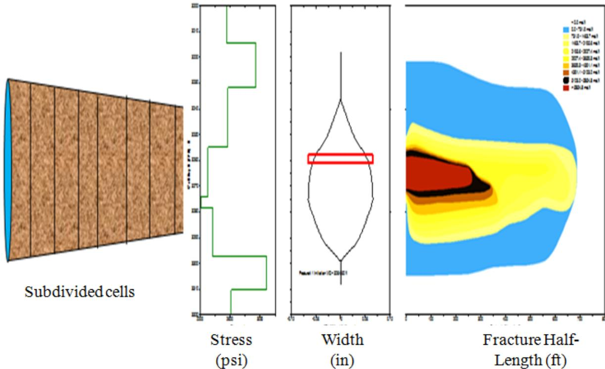
Figure 2.4: Pseudo 3-D model (By Schlumberger FracCADE Simulator)
