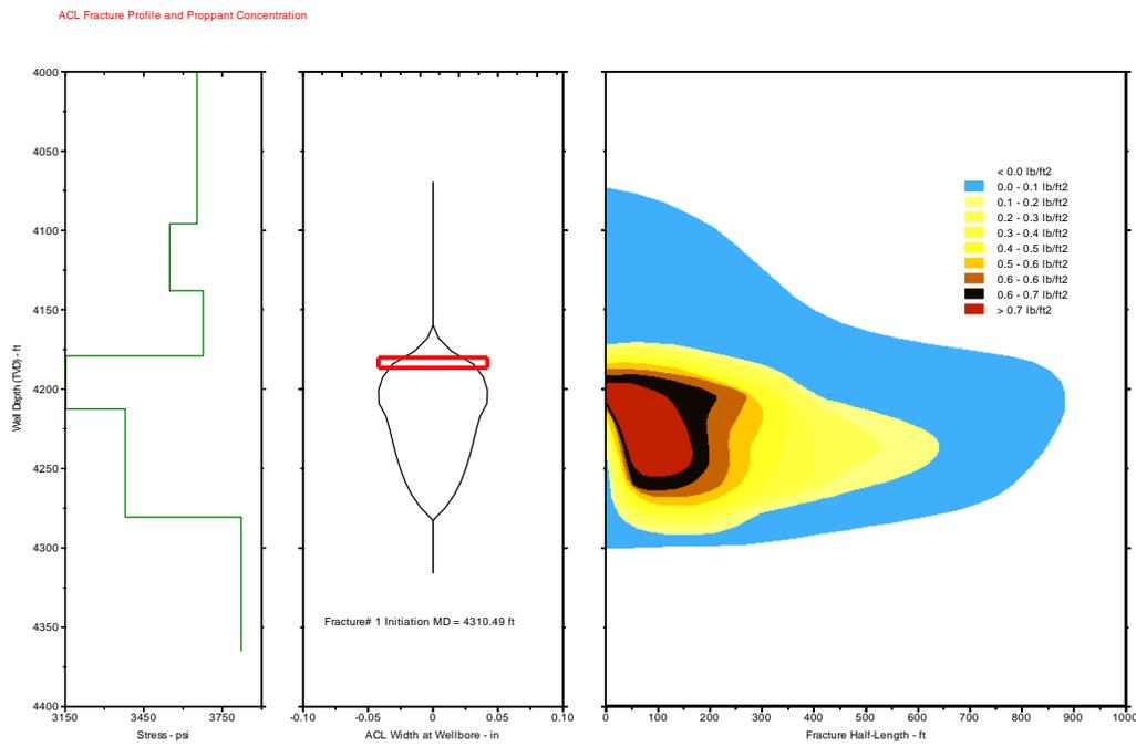
Figure 2.11: High viscosity fluid with 2-D flow proppant distribution after closure
