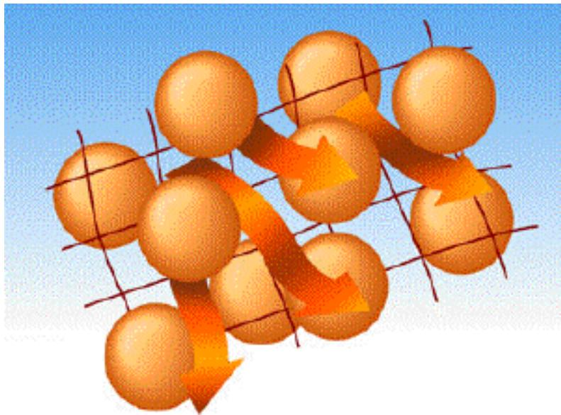
Figure 3.9: Fiber network interlocking proppant (From Heitmann, et al., 2002)
