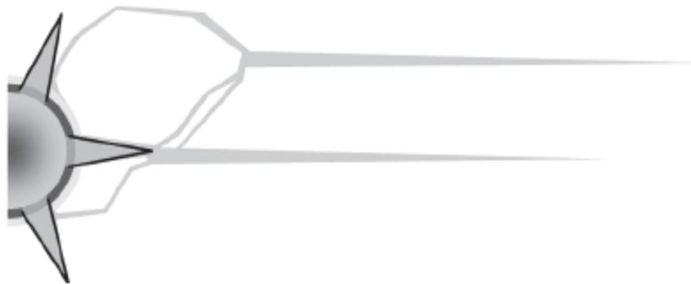
Figure 3.8: Diagrammatic illustration of the restricted flow paths between the perforations and the main fractures that cause tortuosity (From Economides, et al., 2007)
