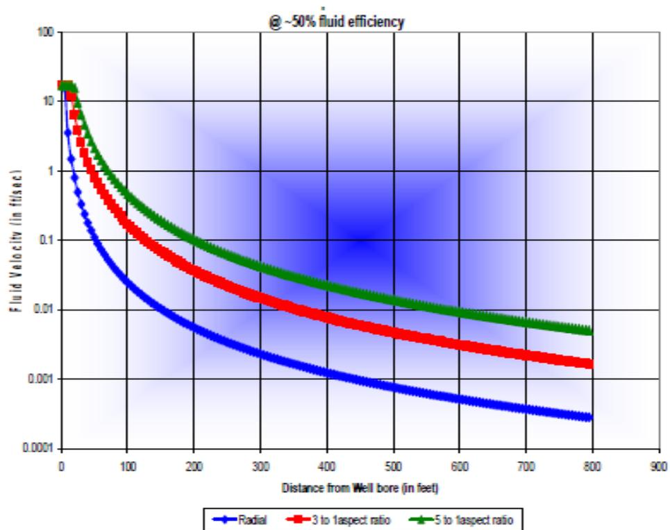
Figure 3.7: Slurry velocity decay vs. distance from wellbore (10 bpm Injection Rate, 10 ft of Height @ Wellbore Velocity 17.1ft/sec @ Wellbore) (From Brannon, et al., 2007)
