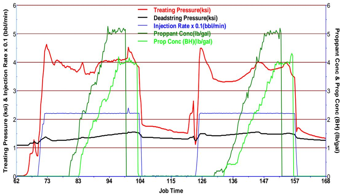
Figure 3.1: Treatment plot for 2 stages fracturing (Surface pressure vs. Deadstring pressure, treatment data from Schlumberger fracturing job database)
