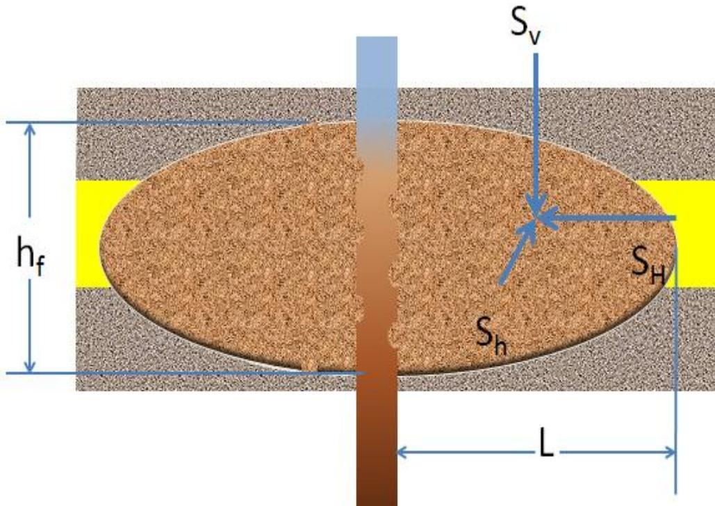
Figure 1.6: Underground stresses direction and vertical fracture geometry when overburden is maximum stress (By author)
