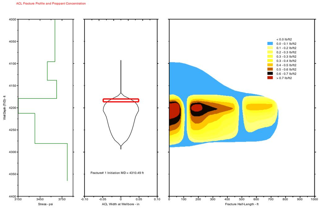
Figure 2.8: Medium viscosity fluid without 2-D flow proppant distribution after closure
