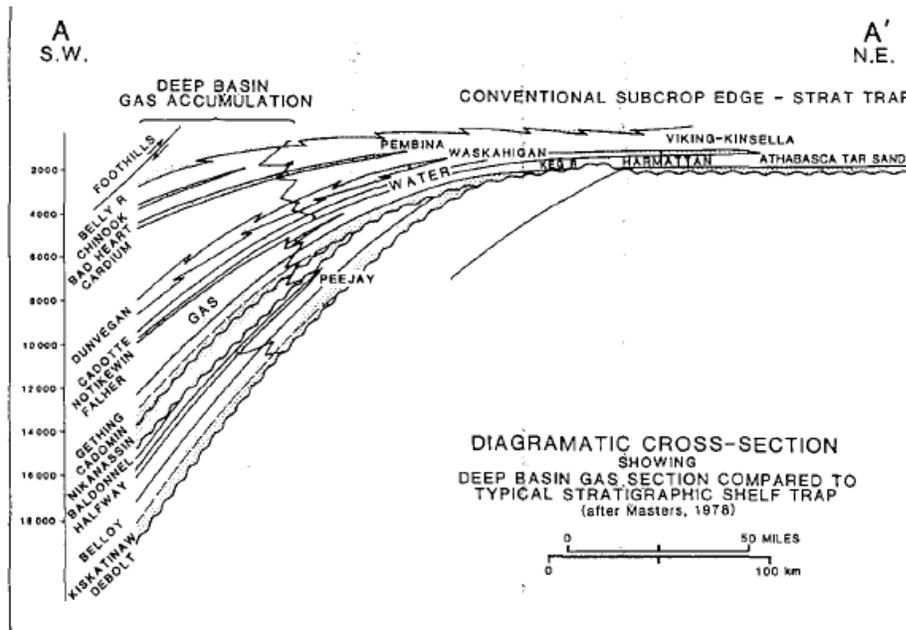
Figure 4.2: Diagrammatic cross section showing Deep Basin Gas Section compared to typical stratigraphic shelf trap (From Maters, 1978)
