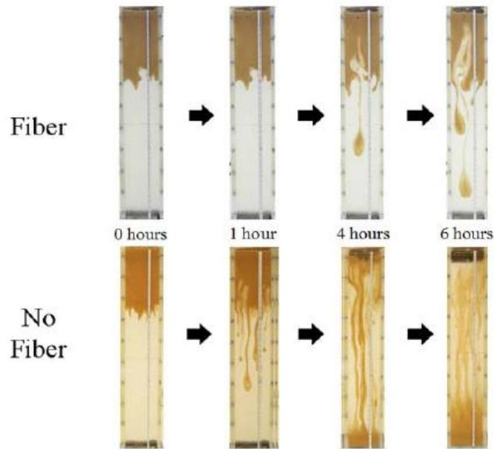
Figure 3.11: Proppant slug setting with and without fiber (From Medvedev, et al., 2013)
