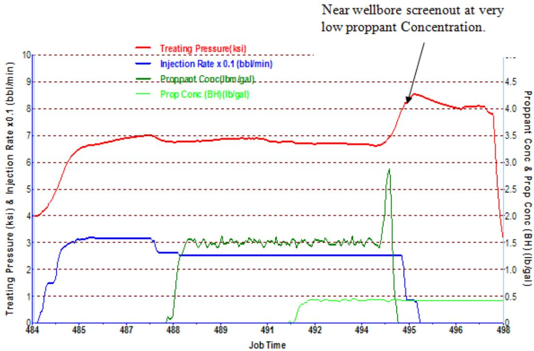
Figure 3.2: Wellbore screenout treatment plot (Treatment data from Schlumberger fracturing job database)
