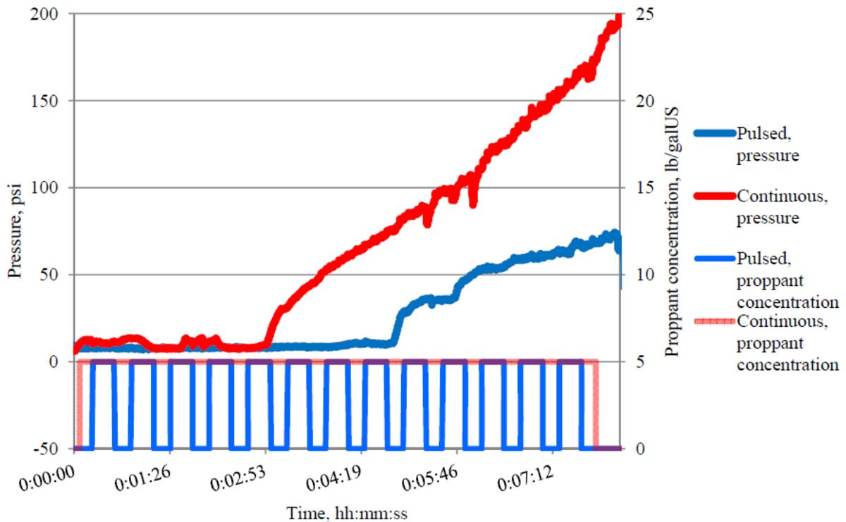
Figure 3.12: Comparison of screenout characteristics of continuous and pulsed injection proppant (From Medvedev, et al., 2013)
