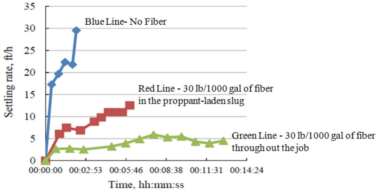
Figure 3.10: Settling rate of front of 12 lb/gal added proppant slug in a slot with different fiber concentration as shown in the plot (From Medvedev, et al., 2013).
