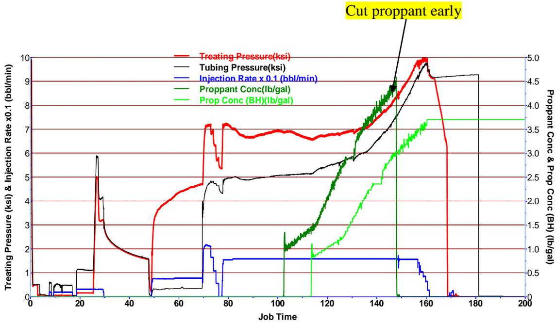
Figure 4.4: Wild River Cadomin formation cut sand with 57,320 lbs pumped out of 132,277 lbs designed (Treatment data from Schlumberger fracturing job database)
