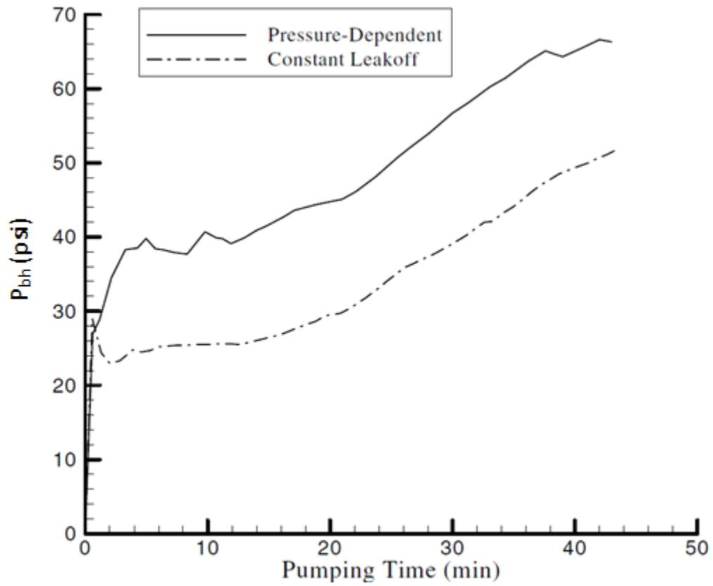
Figure 3.4: Bottom-hole pressure ( $P_{bh}$ ) history – a circular fracture (From Yew et al., 2000)
