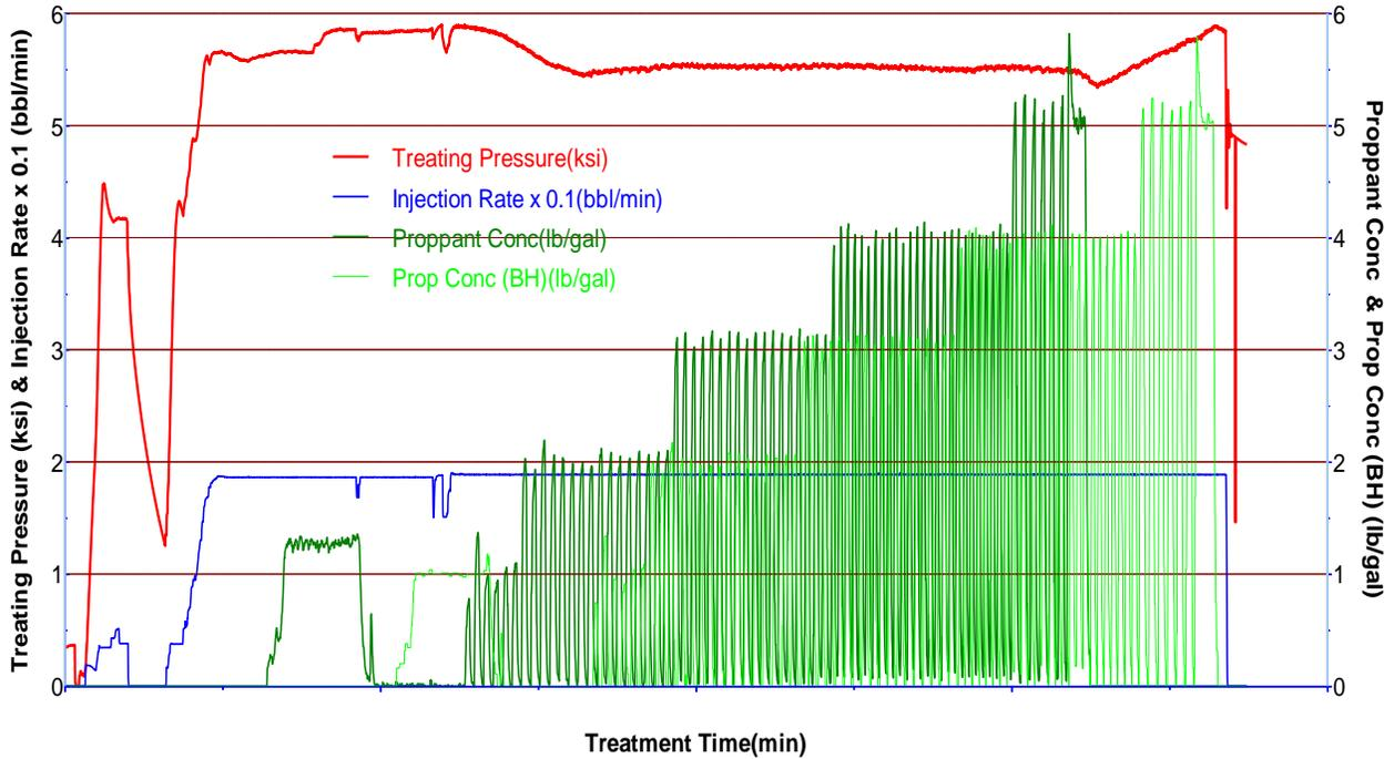
Figure 4.7: Wild River Cadomin formation channel fracturing treatment plot (Treatment data from Schlumberger fracturing job database). Note: treatment time is hidden for confidentiality reason
