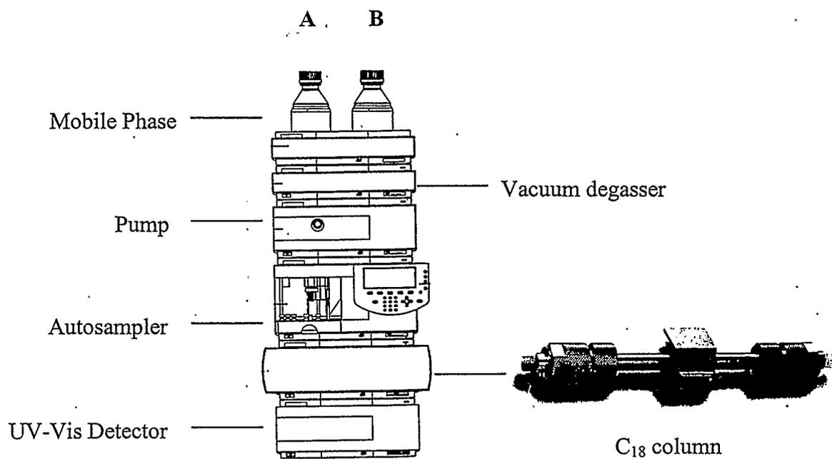
**Figure 3.1.** HPLC instrumentation for the analysis of GSNO (Taken from the reference manual of Agilent Technologies, 1999) (2).
