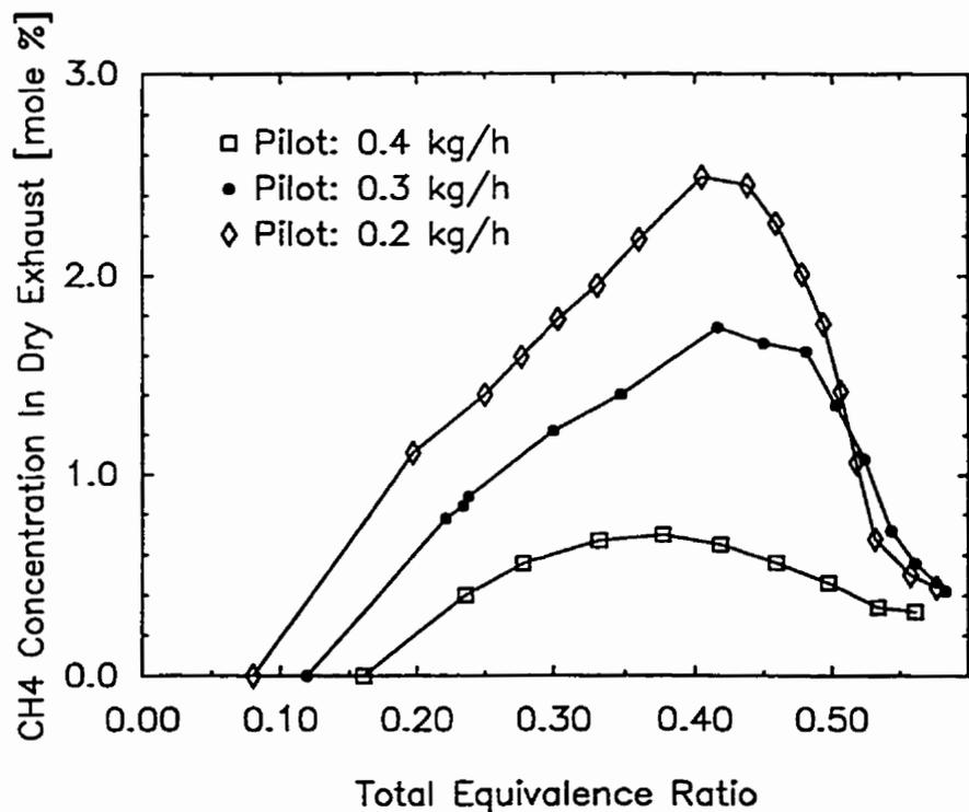
Figure 4.4.2 Variation of Dry Exhaust CH4 Concentration with Total Equivalence Ratio for Dual Fuel Operation with Methane when Using a 41.5 Cetane Number Fuel with Different Pilot Quantities
