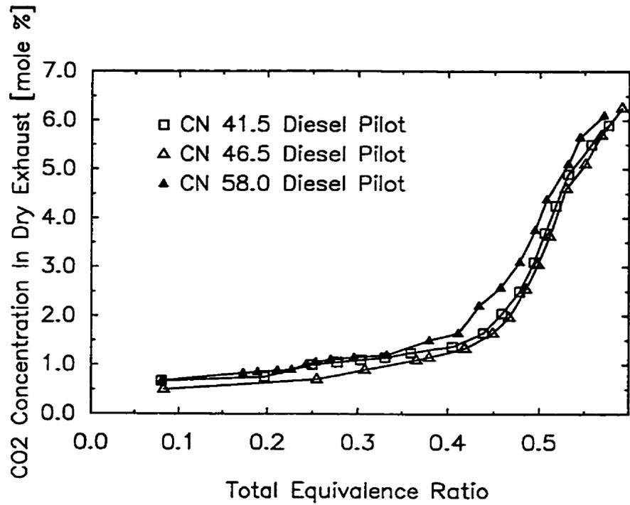
Figure F.1.5 Variation of Dry Exhaust CO<sub>2</sub> Concentration with Total Equivalence Ratio for Dual Fuel Operation with Methane when Using Different Cetane Number Fuels with a 0.20 kg/h Pilot
