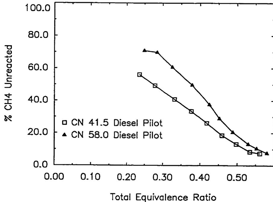
Figure 4.4.10 Variation of the Percent of CH<sub>4</sub> Unreacted with Total Equivalence Ratio for Dual Fuel Operation with Methane when Using Different Cetane Number Fuels with a 0.40 kg/h Pilot
