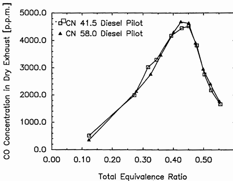
Figure 4.4.20 Variation of Dry Exhaust CO Concentration with Total Equivalence Ratio for Dual Fuel Operation with Propane when Using Different Cetane Number Fuels with a 0.30 kg/h Pilot
