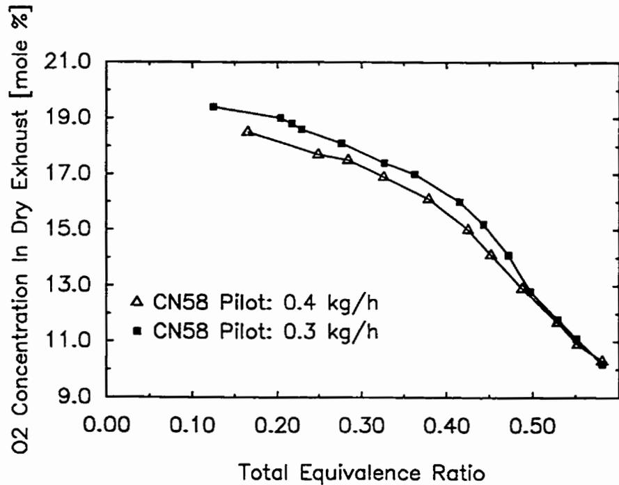
Figure F.1.12 Variation of Dry Exhaust O<sub>2</sub> Concentration with Total Equivalence Ratio for Dual Fuel Operation with Methane when Using Different Pilot Quantities with a 58.0 Cetane Number Pilot
