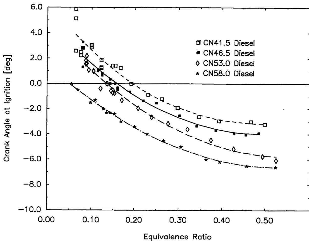
Figure 4.2.1 Variations of the Point of Ignition with Equivalence Ratio for Diesel Operation when Using Different Cetane Number Fuels
