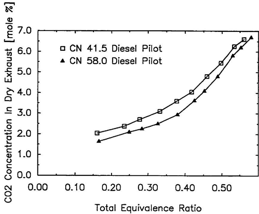
Figure F.1.9 Variation of Dry Exhaust CO<sub>2</sub> Concentration with Total Equivalence Ratio for Dual Fuel Operation with Methane when Using Different Cetane Number Fuels with a 0.40 kg/h Pilot
