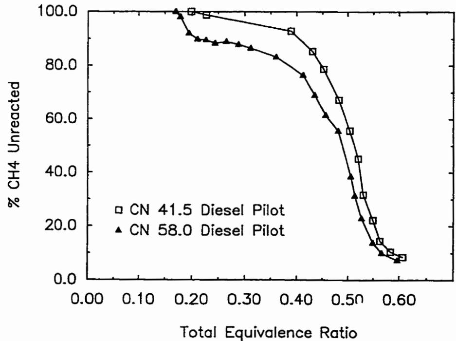
Figure 4.4.16 Variation of the Percent of CH4 Unreacted with Total Equivalence Ratio for Dual Fuel Operation with a CH4-N2 Mixture (50% by Mass CH4) when Using Different Cetane Number Fuels with a 0.20 kg/h Pilot
