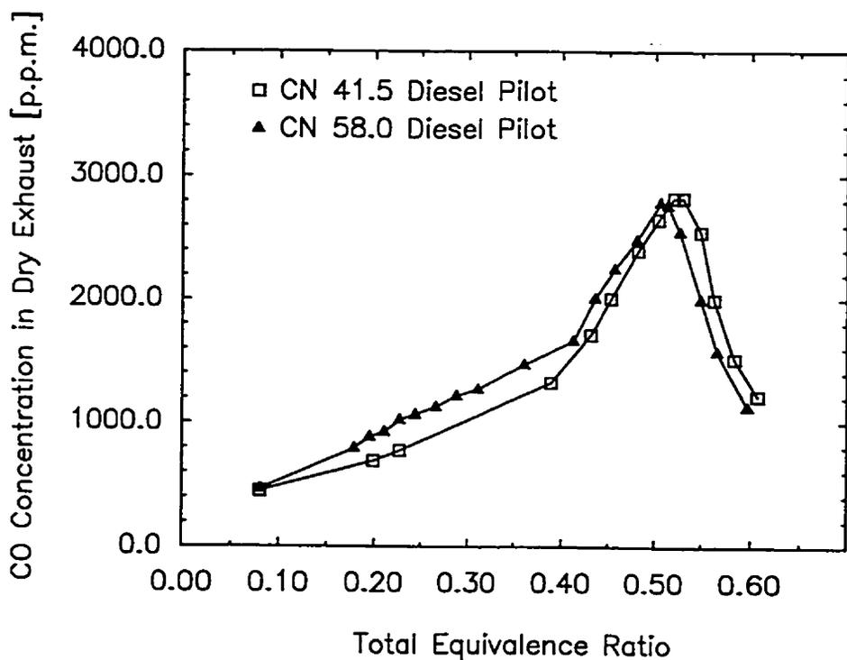
Figure 4.4.14 Variation of Dry Exhaust CO Concentration with Total Equivalence Ratio for Dual Fuel Operation with a CH<sub>4</sub>-N<sub>2</sub> Mixture (50% by Mass CH<sub>4</sub>) when Using Different Cetane Number Fuels with a 0.20 kg/h Pilot
