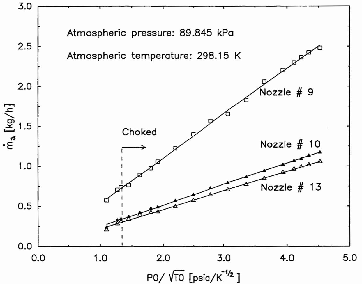
Figure A.1.1 Calibration of Choked Nozzles for Metering Gases
