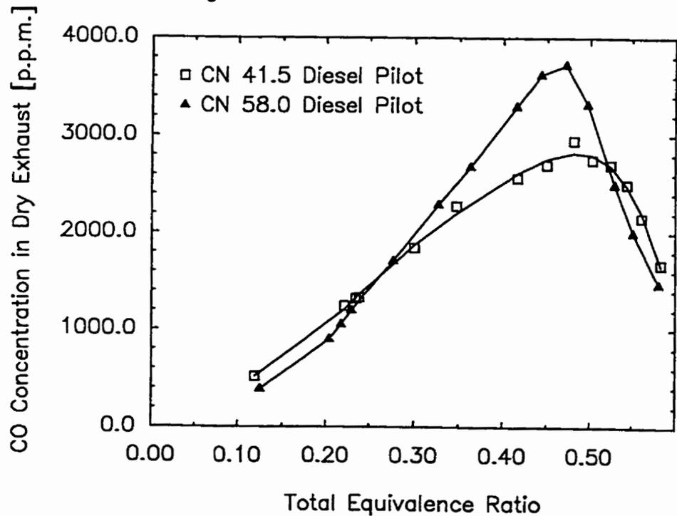
Figure 4.4.12 Variation of Dry Exhaust CO Concentration with Total Equivalence Ratio for Dual Fuel Operation with Methane when Using Different Cetane Number Fuels with a 0.30 kg/h Pilot
