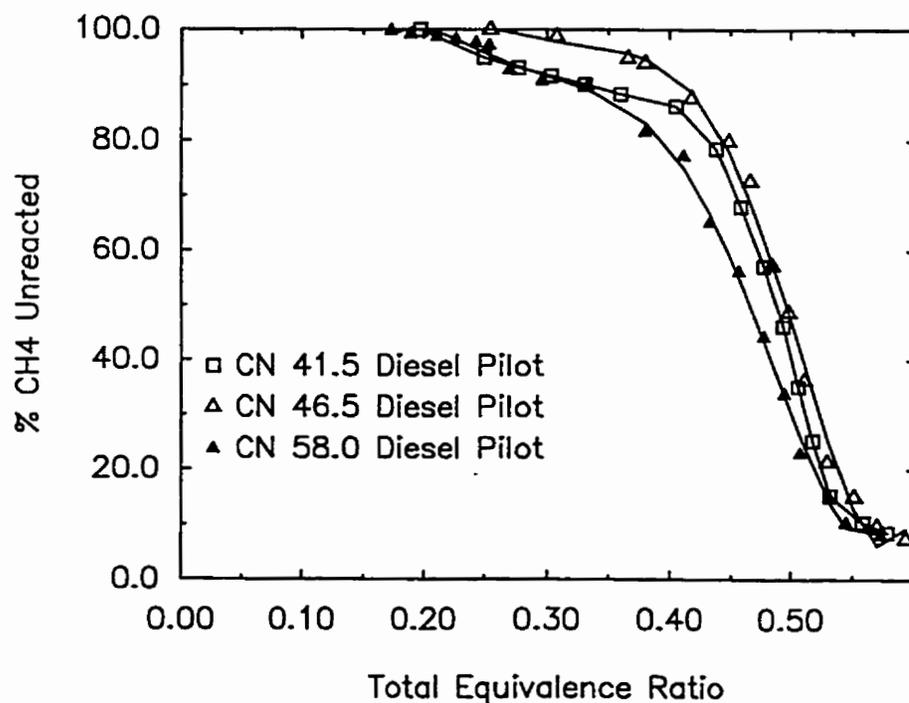
Figure 4.4.6 Variation of the Percent of CH<sub>4</sub> Unreacted with Total Equivalence Ratio for Dual Fuel Operation with Methane when Using Different Cetane Number Fuels with a 0.20 kg/h Pilot
