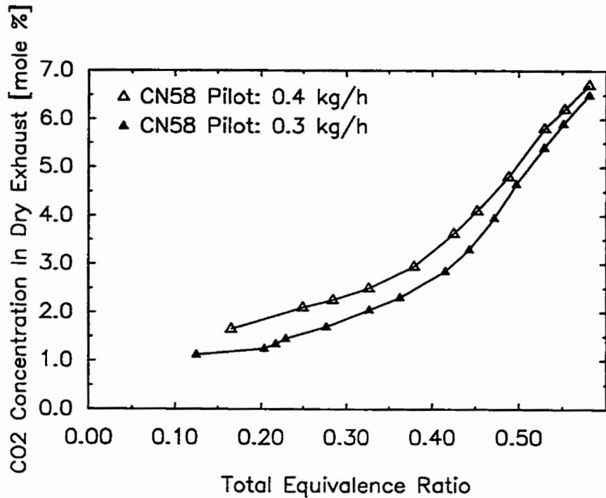
Figure F.1.11 Variation of Dry Exhaust CO<sub>2</sub> Concentration with Total Equivalence Ratio for Dual Fuel Operation with Methane when Using Different Pilot Quantities with a 58.0 Cetane Number Pilot
