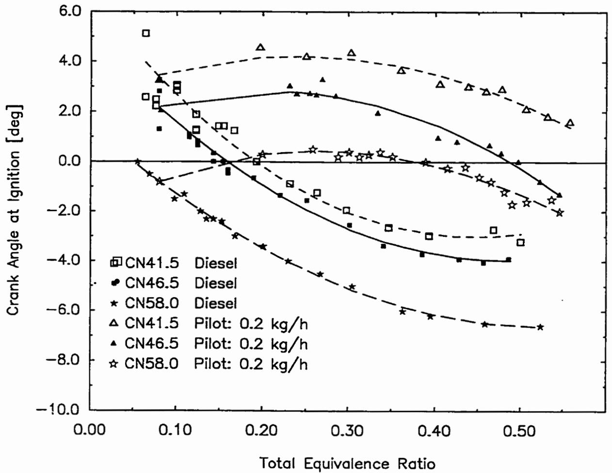
Figure 4.2.5 Variations of the Point of Ignition with Total Equivalence Ratio for Dual Fuel Operation with Methane when Using Different Cetane Number Fuels with a 0.20 kg/h Pilot
