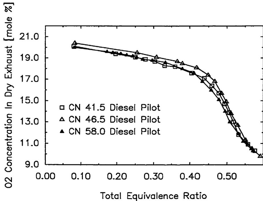
Figure F.1.6 Variation of Dry Exhaust O<sub>2</sub> Concentration with Total Equivalence Ratio for Dual Fuel Operation with Methane when Using Different Cetane Number Fuels with a 0.20 kg/h Pilot
