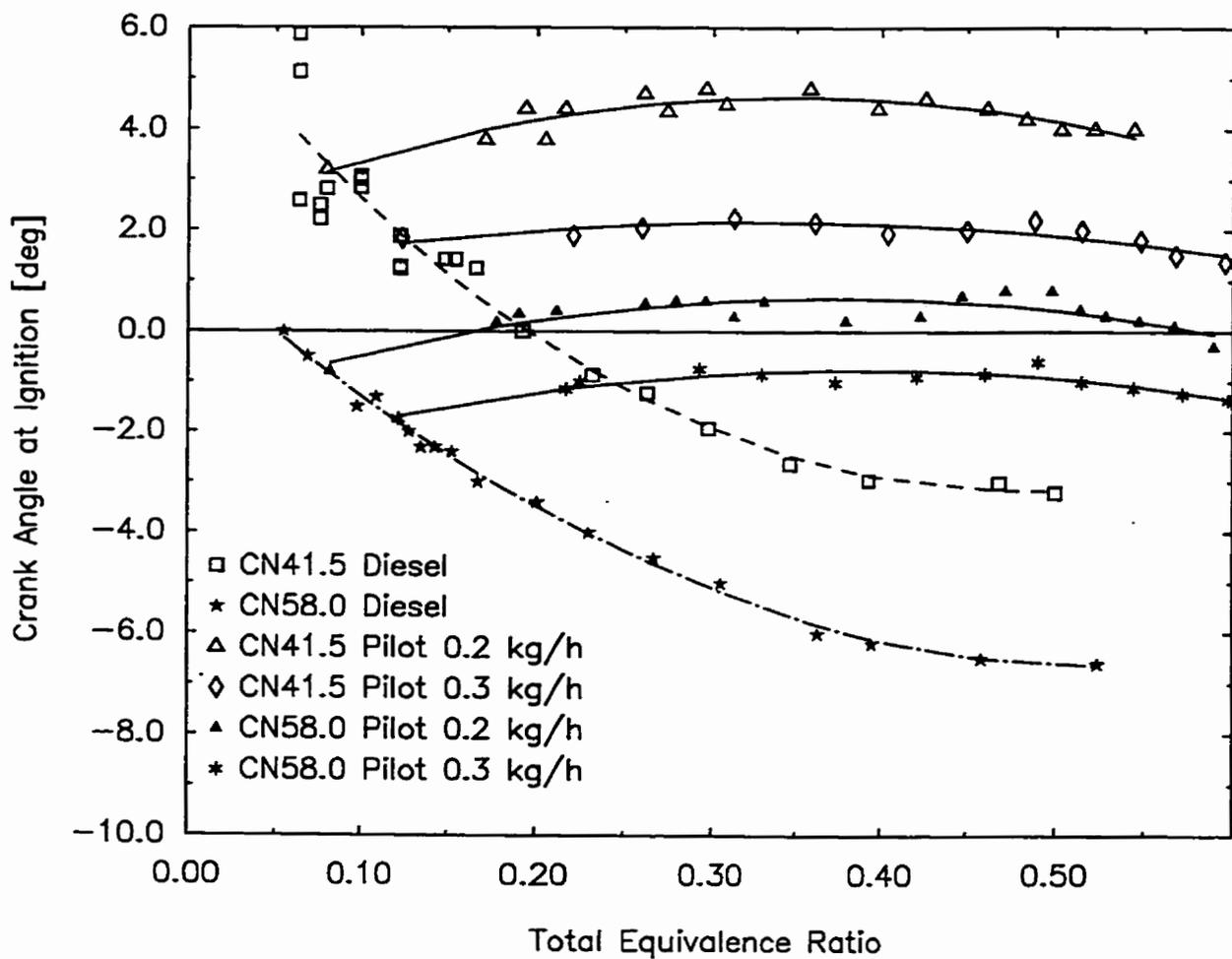
Figure 4.2.7 Variations of the Point of Ignition with Total Equivalence Ratio for Dual Fuel Operation when Using Different Cetane Number Fuels and Different Pilot Quantities with a CH<sub>4</sub>-N<sub>2</sub> Mixture (50% by mass CH<sub>4</sub>)
