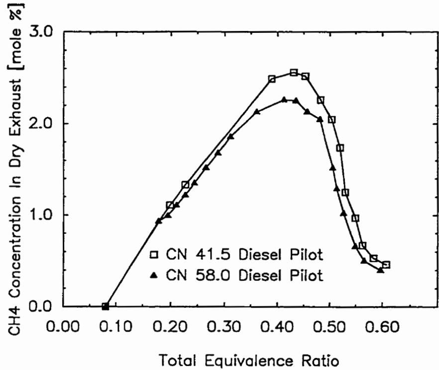
Figure 4.4.15 Variation of Dry Exhaust CH4 Concentration with Total Equivalence Ratio for Dual Fuel Operation with a CH4-N2 Mixture (50% by Mass CH4) when Using Different Cetane Number Fuels with a 0.20 kg/h Pilot
