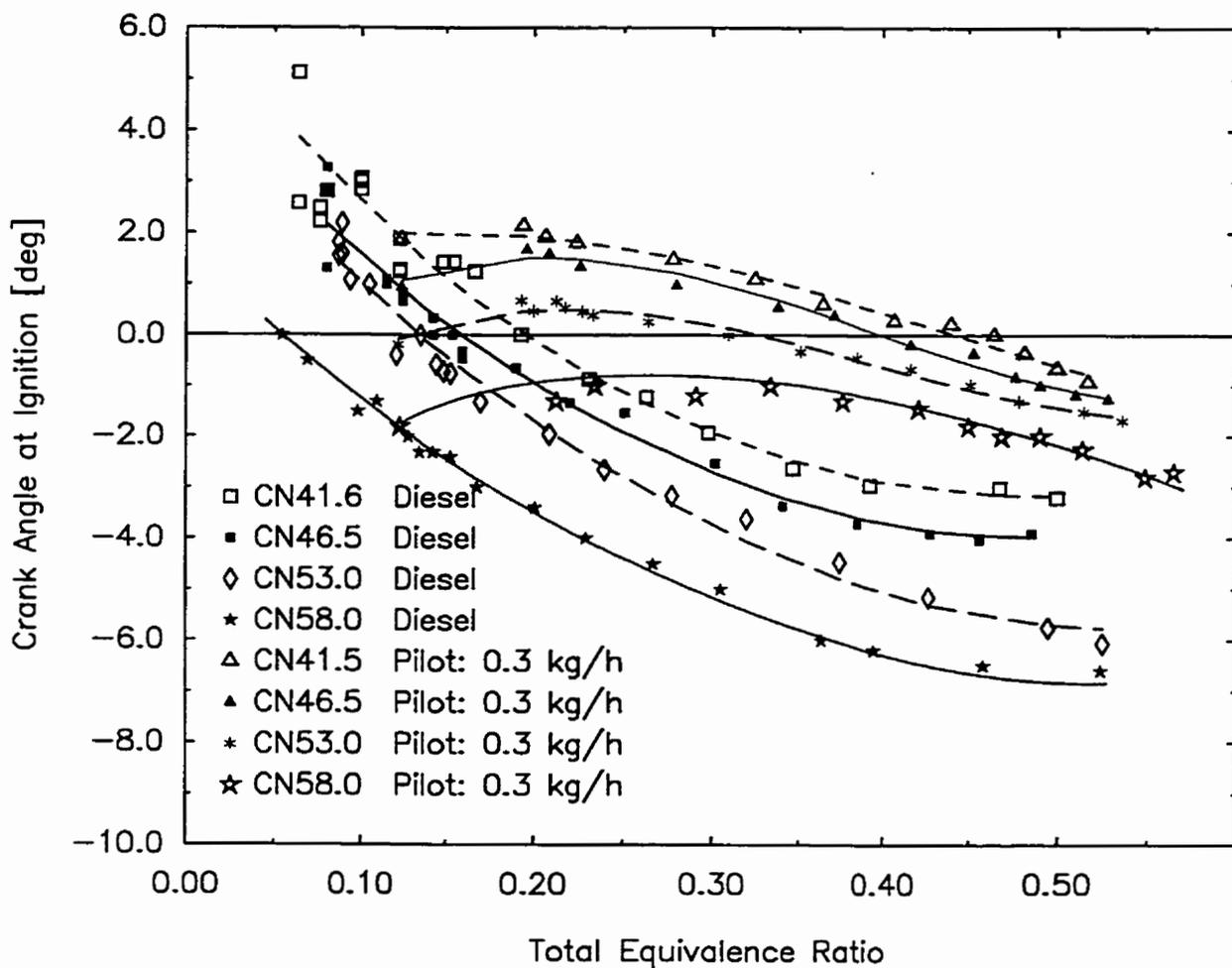
Figure 4.2.4 Variations of the Point of Ignition with Total Equivalence Ratio for Dual Fuel Operation with Methane when Using Different Cetane Number Fuels with a 0.30 kg/h Pilot
