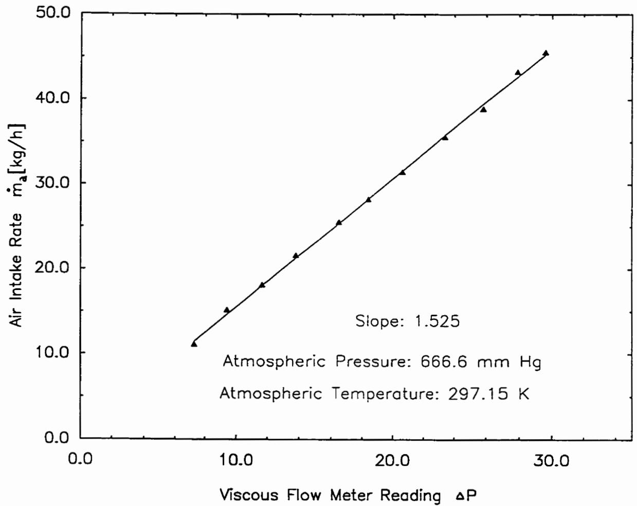
Fig. B.1.1. Calibration of the Viscous Flow Air Meter
