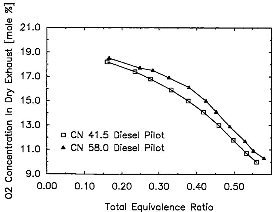
Figure F.1.10 Variation of Dry Exhaust O<sub>2</sub> Concentration with Total Equivalence Ratio for Dual Fuel Operation with Methane when Using Different Cetane Number Fuels with a 0.40 kg/h Pilot
