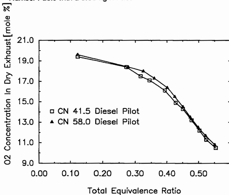
Figure F.1.16 Variation of Dry Exhaust O<sub>2</sub> Concentration with Total Equivalence Ratio for Dual Fuel Operation with Propane when Using Different Cetane Number Fuels with a 0.30 kg/h Pilot
