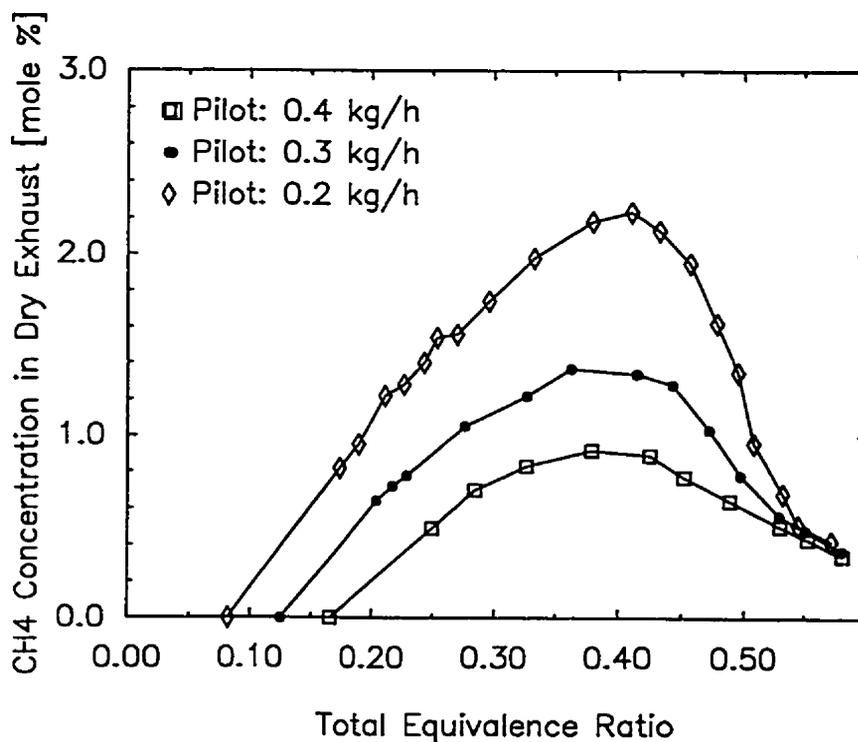
Figure 4.4.4 Variation of Dry Exhaust CH4 Concentration with Total Equivalence Ratio for Dual Fuel Operation with Methane when Using a 58.0 Cetane Number Fuel with Different Pilot Quantities
