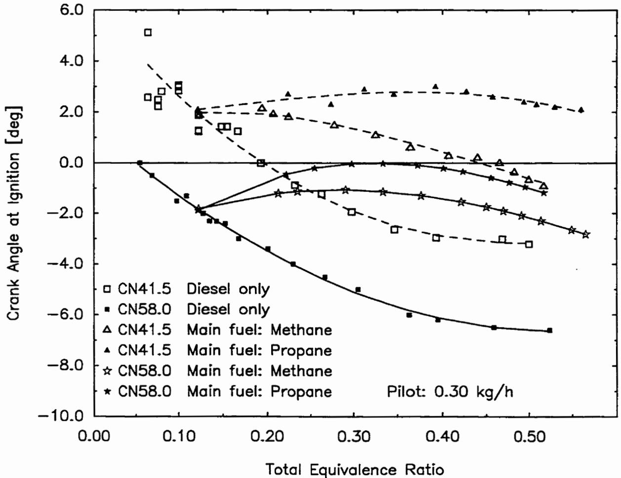
Figure 4.2.6 Variations of the Point of Ignition with Total Equivalence Ratio for Dual Fuel Operation with Propane when Using Different Cetane Number Fuels as Compared to the Corresponding Values Obtained when Operating with Methane
