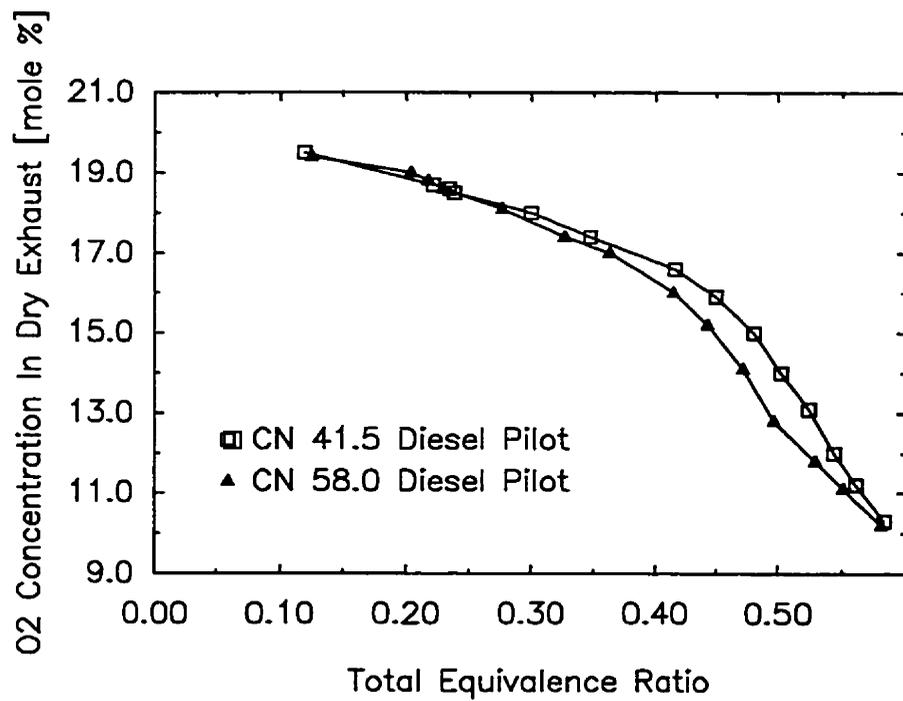
Figure F.1.8 Variation of Dry Exhaust O<sub>2</sub> Concentration with Total Equivalence Ratio for Dual Fuel Operation with Methane when Using Different Cetane Number Fuels with a 0.30 kg/h Pilot
