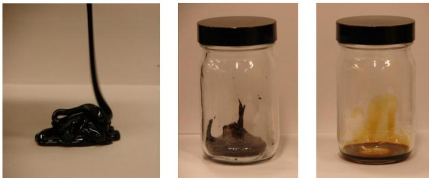
Figure 5–6: Digital photographs of gas-free bitumen (left) and flashed-off liquid samples (middle and right) taken from liquid-liquid equilibrium study of Surmont bitumen / propane mixtures.
