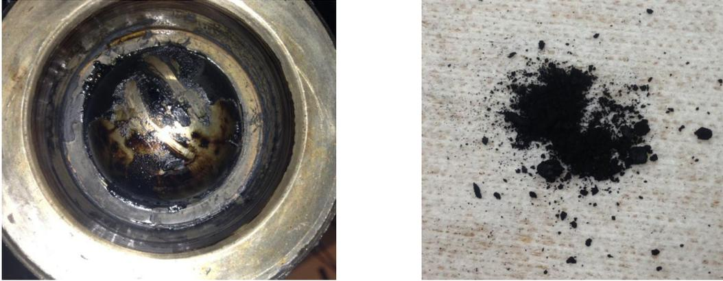
Figure 6–1: Digital photographs of the precipitated asphaltene from the mixture of Surmont bitumen / *n*-hexane at the temperature of 100°C and at a concentration of 0.6 *n*-hexane weight fraction; a) immediately after experiment; b) after evaporation of *n*-hexane.
