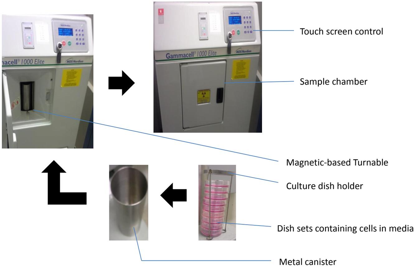
**Figure B: Gamma Cell 1000® Elite (irradiator)**
