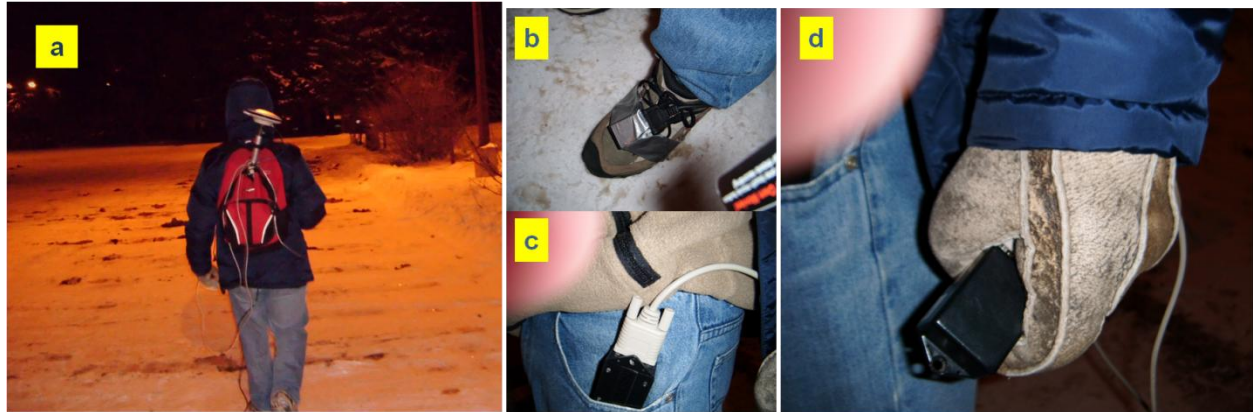
Figure 5-2: Outdoor data collection: (a) the test subject is carrying the backpack with a small laptop and a GPS antenna used as reference. The subject carries a foot mounted IMU (b), an IMU in his pocket (c) and an IMU in a swinging hand (d).
