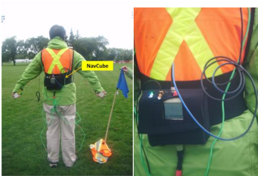
Figure 5-4: (Left) Test subject wearing the NavCube at the waist, two IMUs are foot mounted and two IMUs are in the user's hand; (Right) Zoom on the NavCube
