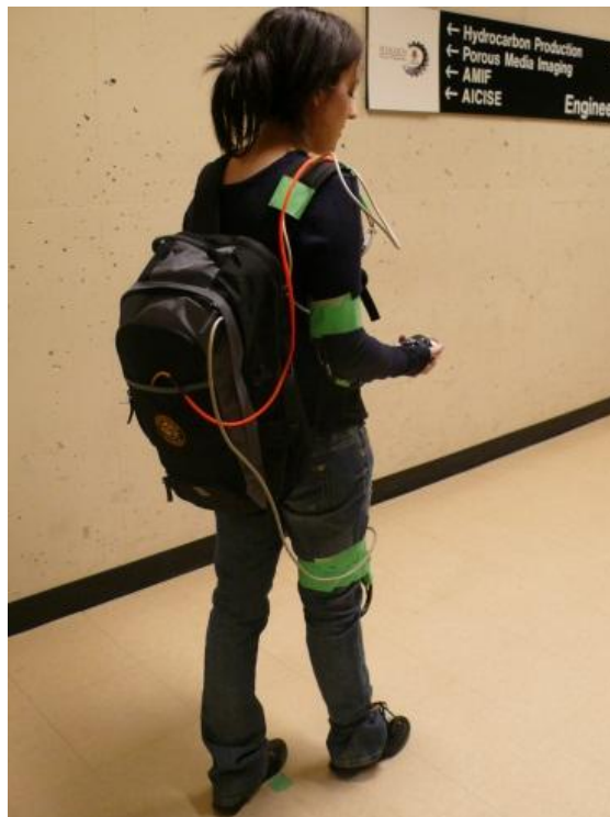
Figure 5-1: Test set up: the IMUs are connected to a laptop carried inside a backpack
