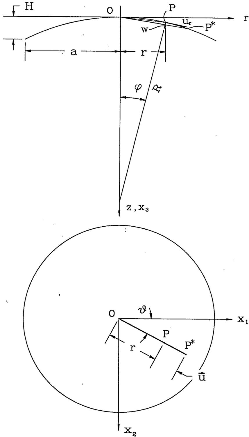
Figure 2.3: Displacement field of the shell
