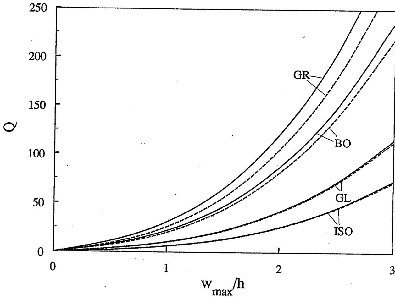
Figure 4.62: Effect of material properties on the static large-deflection response of an elastically supported three-layer circular plate (  $K_b=1$ ,  $K_i=2$ ,  $a/h=10$  )
