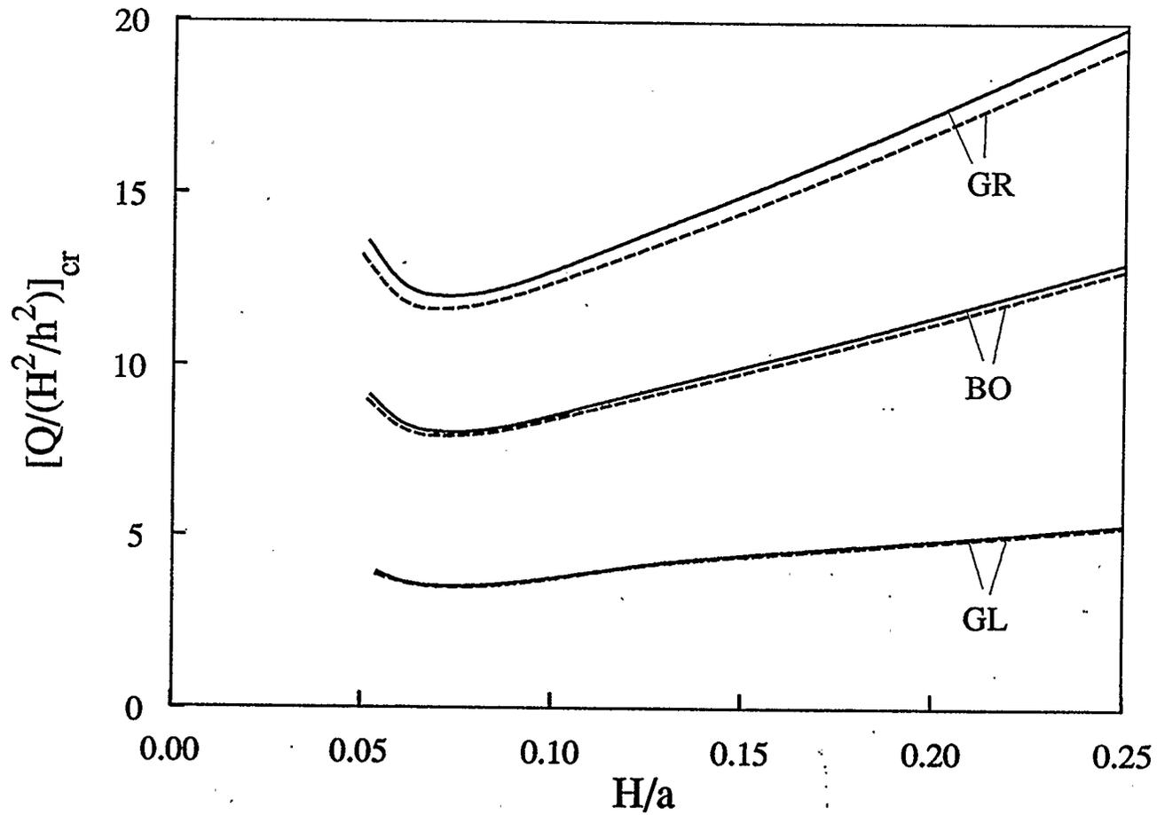
Figure 4.44: Effect of material properties on buckling load of an immovable simply-supported three-layer shallow spherical shell (  $a/h=15$  )
