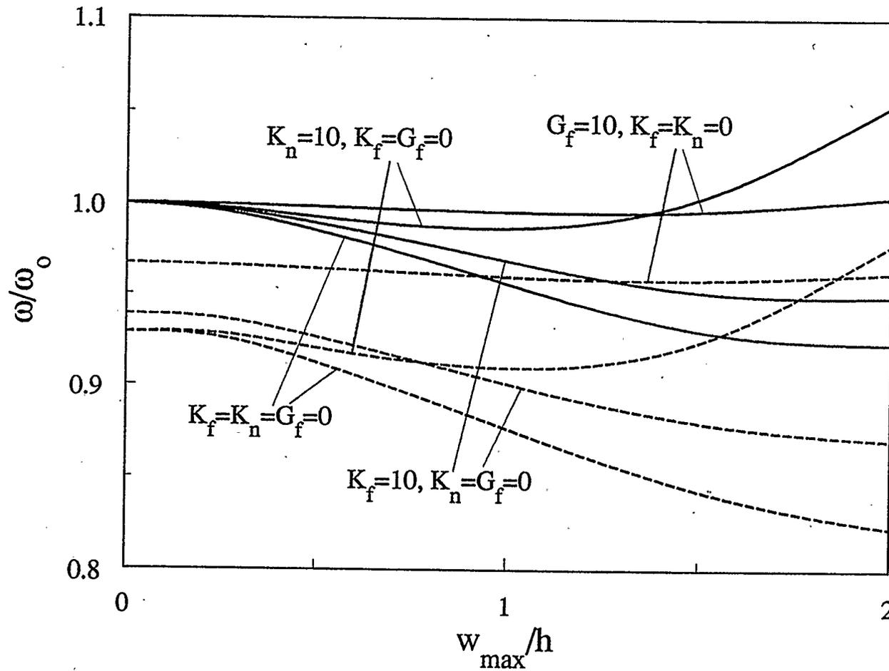
Figure 4.42: Effect of elastic foundations on the frequency-amplitude response of a movable clamped two-layer graphite-epoxy shallow spherical shell (  $a/h=10, H/a=0.15$  )
