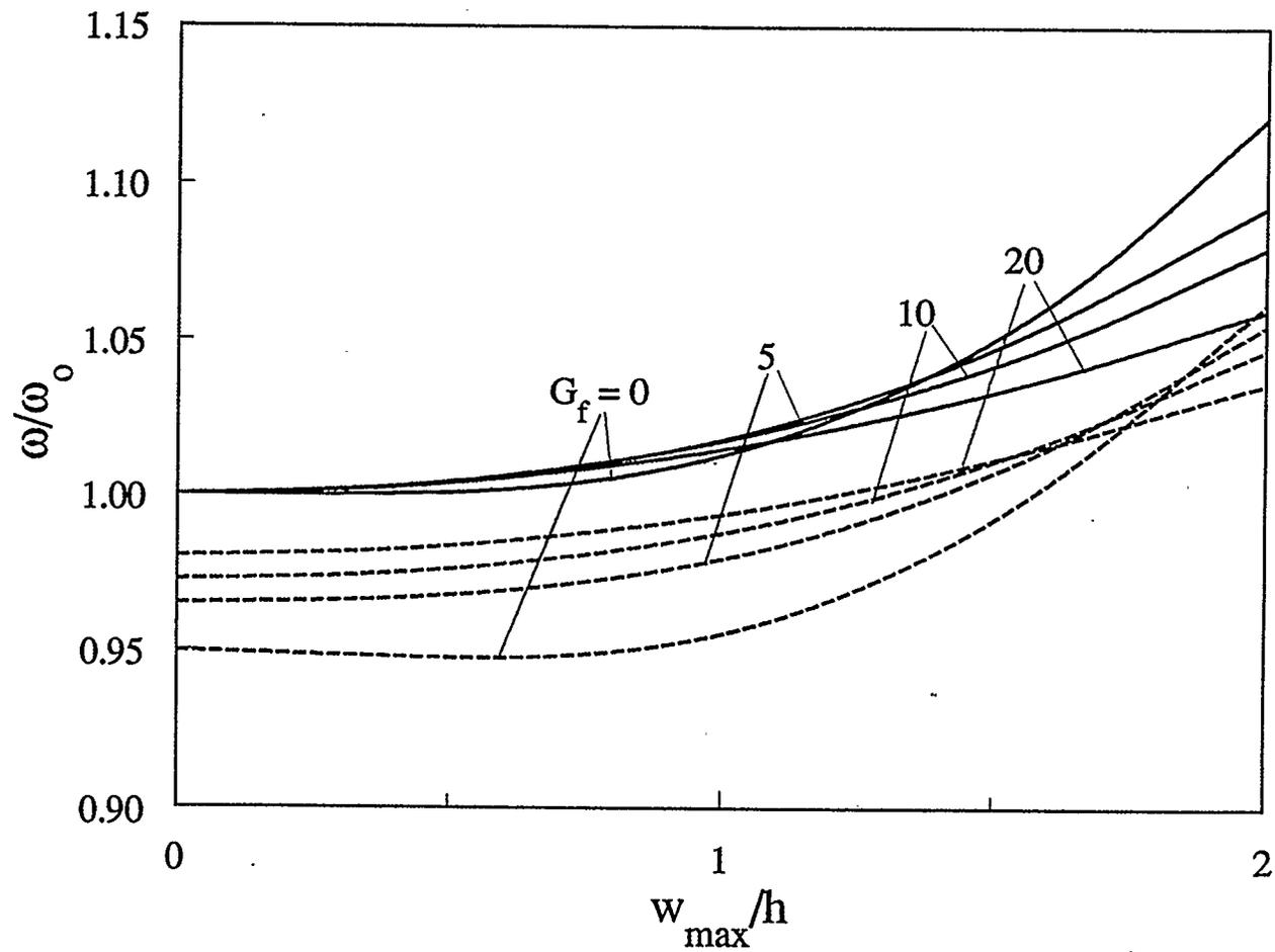
Figure 4.25: Effect of Pasternak foundation parameter on the frequency-amplitude response of a movable clamped five-layer boron-epoxy imperfect shallow spherical shell ( $\bar{W}_1=0.1, K_f=10, K_n=10, a/h=10, H/a=0.15$ )
