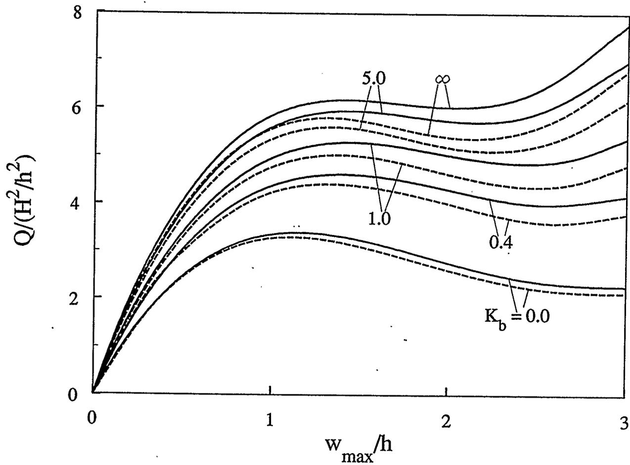
Figure 4.51: Effect of rotational edge stiffness on the postbuckling response of a three-layer boron-epoxy shallow spherical shell with a movable edge (  $a/h=12$ ,  $H/a=0.2$  )
