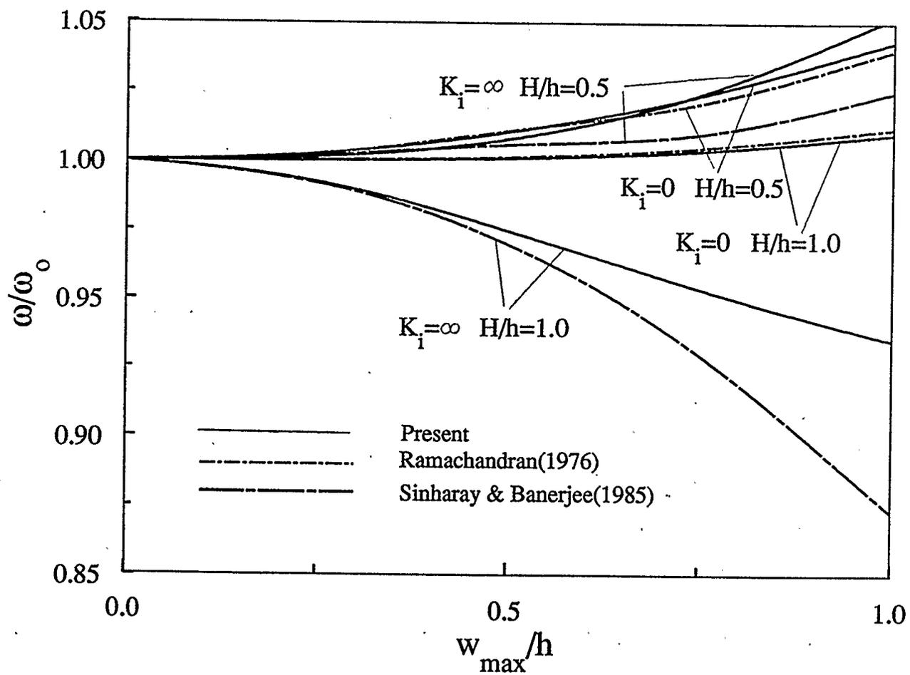
Figure 4.1: Comparison of the frequency-amplitude response for clamped immovable and movable isotropic shallow spherical shells with different shell rises ( $\nu_{\theta r} = 0.3$ )
