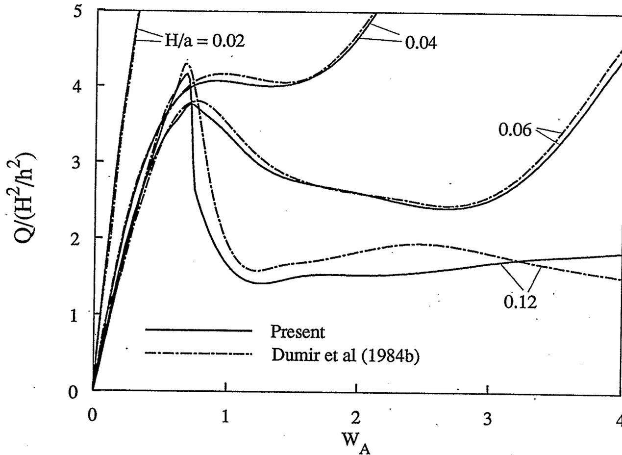
Figure 4.7: Comparison of buckling and postbuckling behaviour for an immovable clamped orthotropic shallow spherical shell with different shell rises ( $E_\theta/E_r=3$ ,  $\nu_{\theta r}=0.3$ )
