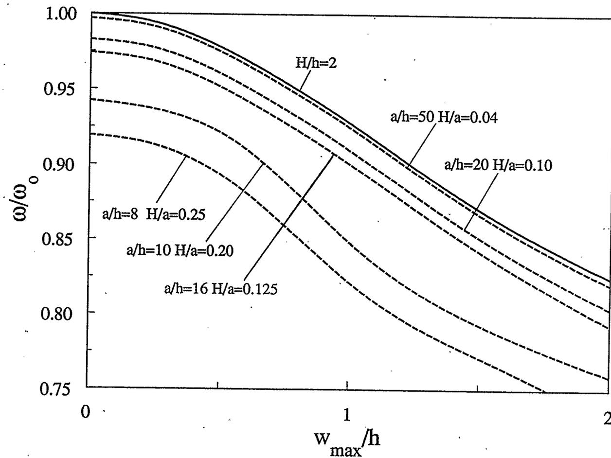
Figure 4.11: Effect of the base radius-to-thickness ratio on the frequency-amplitude response of a movable clamped three-layer graphite-epoxy shallow spherical shell
