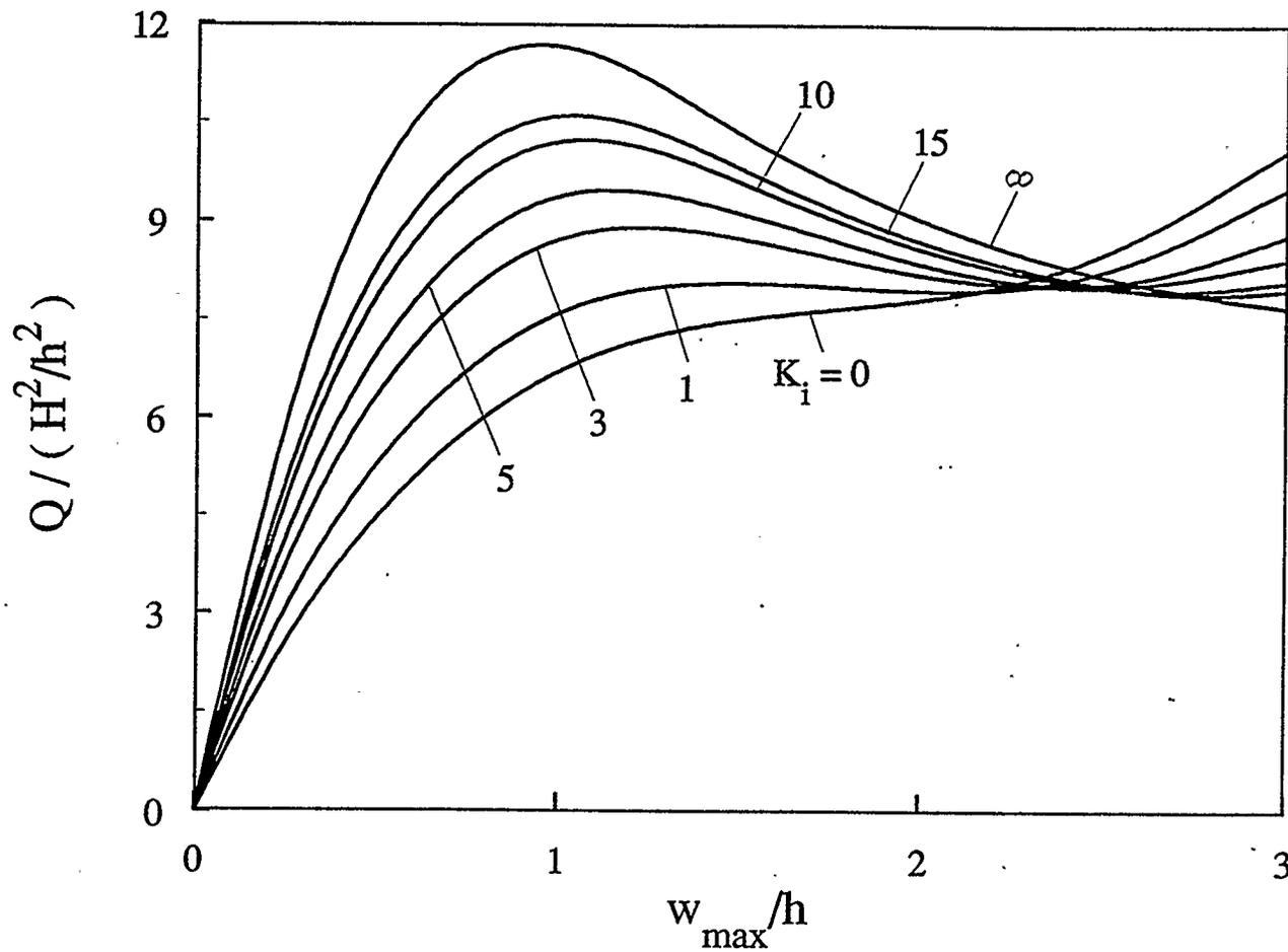
Figure 4.52: Effect of inplane edge stiffness on the postbuckling response of a five-layer boron-epoxy shallow spherical shell with a clamped edge (  $a/h=20$ ,  $H/a=0.125$  )
