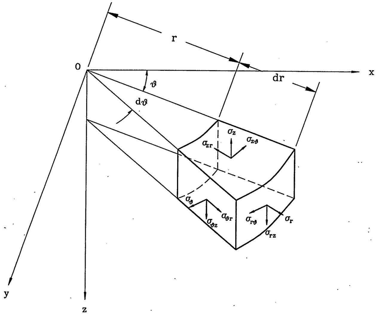
Figure 2.4: Sign convention for stresses in cylindrical coordinates
