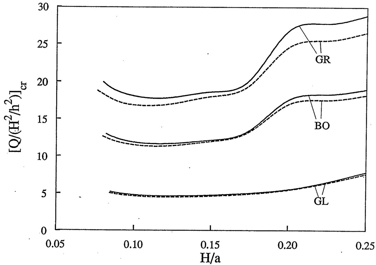
Figure 4.43: Effect of material properties on buckling load of an immovable clamped five-layer shallow spherical shell (  $a/h=20$  )
