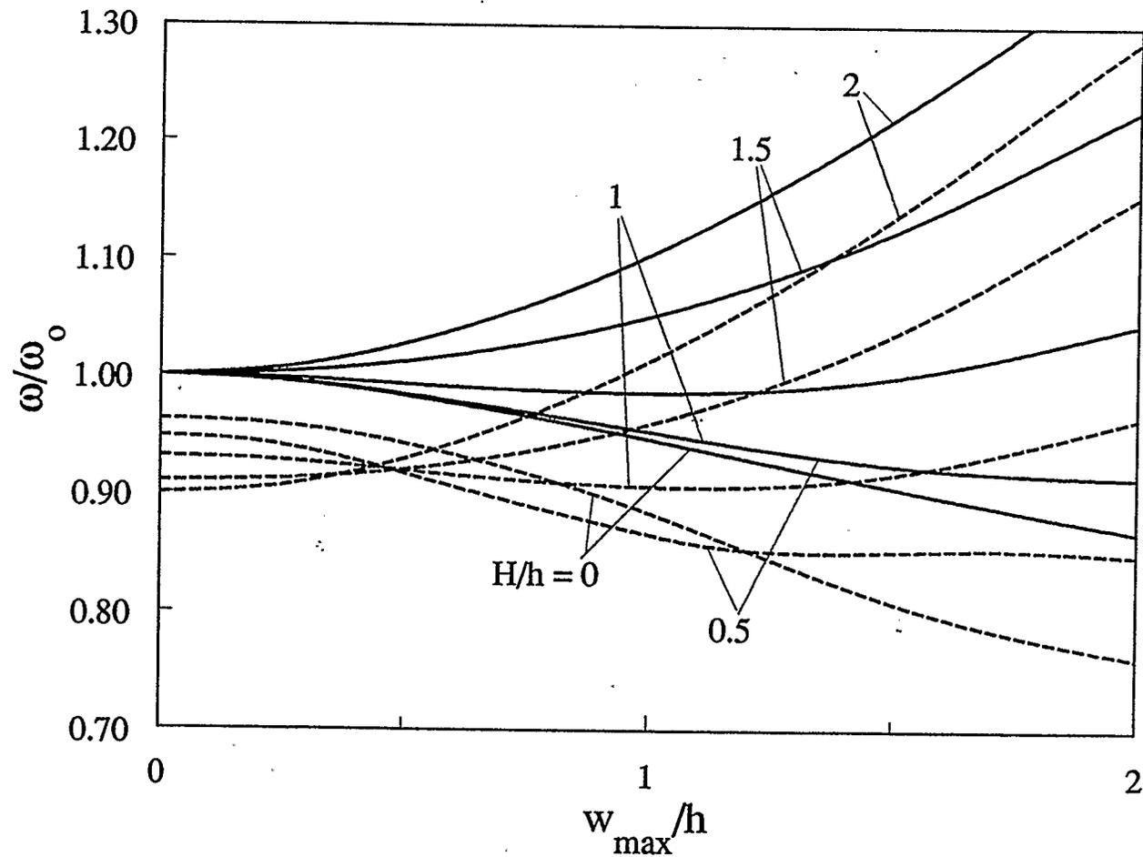
Figure 4.20: Effect of the shell rise on the frequency-amplitude response of an elastically supported five-layer graphite-epoxy shallow spherical shell resting on elastic foundations ( $K_p=2$ ,  $K_i=3$ ,  $K_f=2$ ,  $K_n=2$ ,  $G_f=1.5$ ,  $a/h=10$ )
