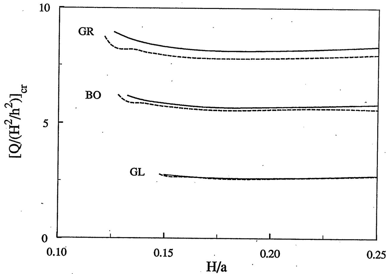
Figure 4.67: Effect of material properties on buckling load of a movable clamped two-layer shallow spherical shell (  $a/h=20$  )
