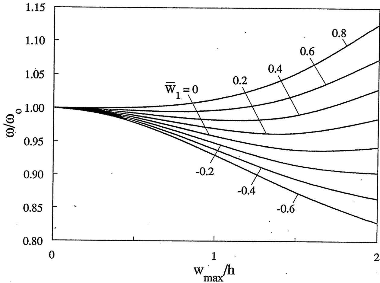
Figure 4.23: Effect of geometrically initial imperfection on the frequency-amplitude response of a movable simply-supported three-layer glass-epoxy shallow spherical shell ( $a/h=12$ ,  $H/a=0.1$ )
