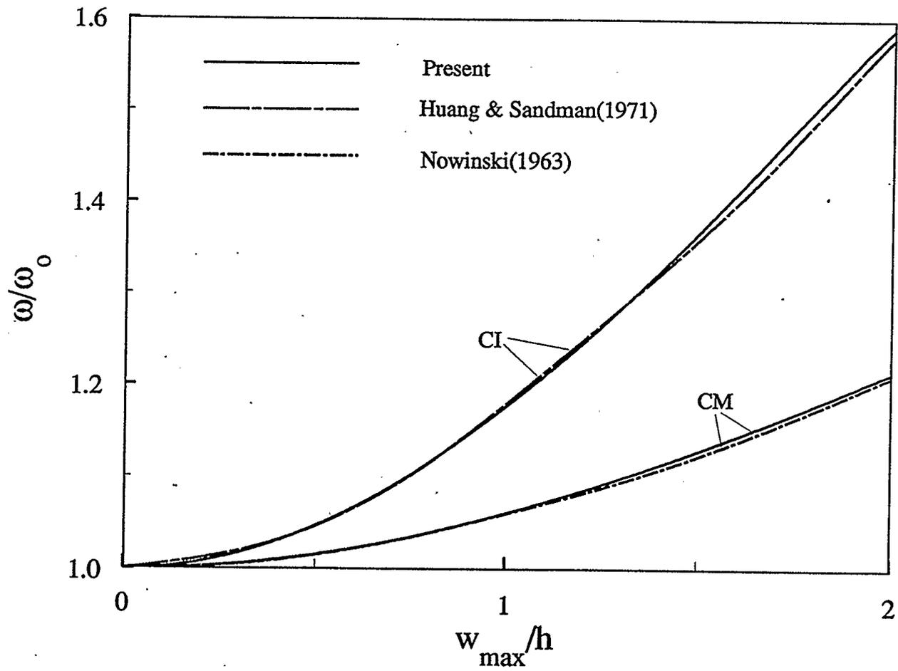
Figure 4.5: Comparison of the frequency-amplitude response for clamped immovable ( $\nu_{\theta r}=1/3$ ) and movable ( $\nu_{\theta r}=0.3$ ) isotropic circular plates
