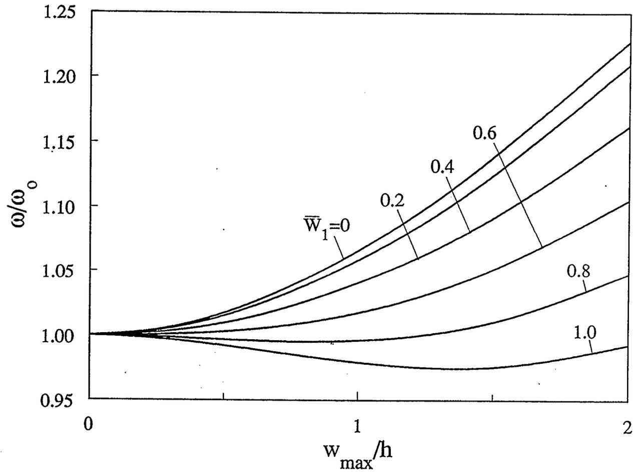
Figure 4.41: Effect of geometrically initial imperfections on the frequency-amplitude response of a movable clamped four-layer glass-epoxy circular plate (  $a/h=15$  )
