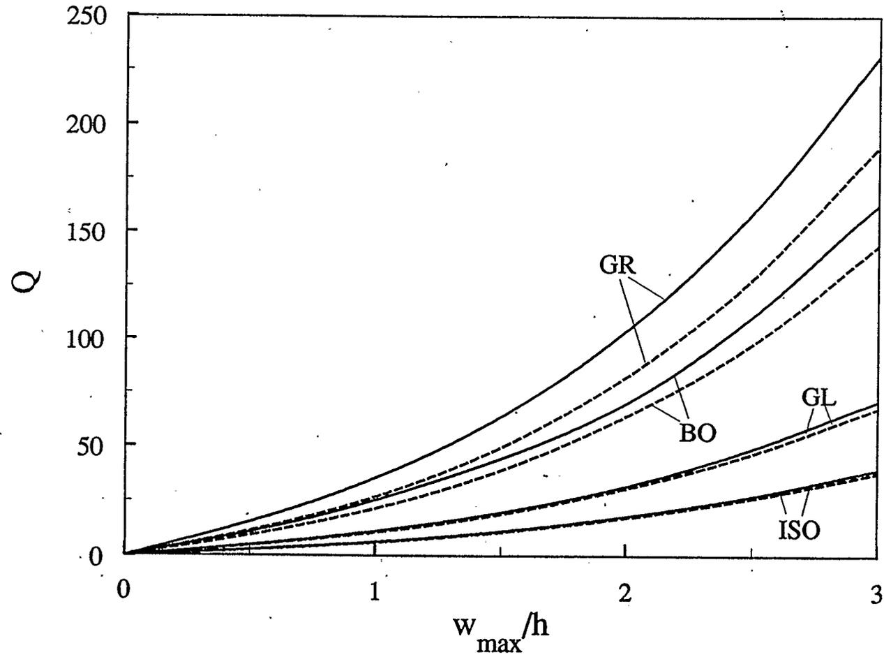
Figure 4.70: Effect of material properties on the static large-deflection response of an elastically supported six-layer circular plate (  $K_p=3$ ,  $a/h=10$  )
