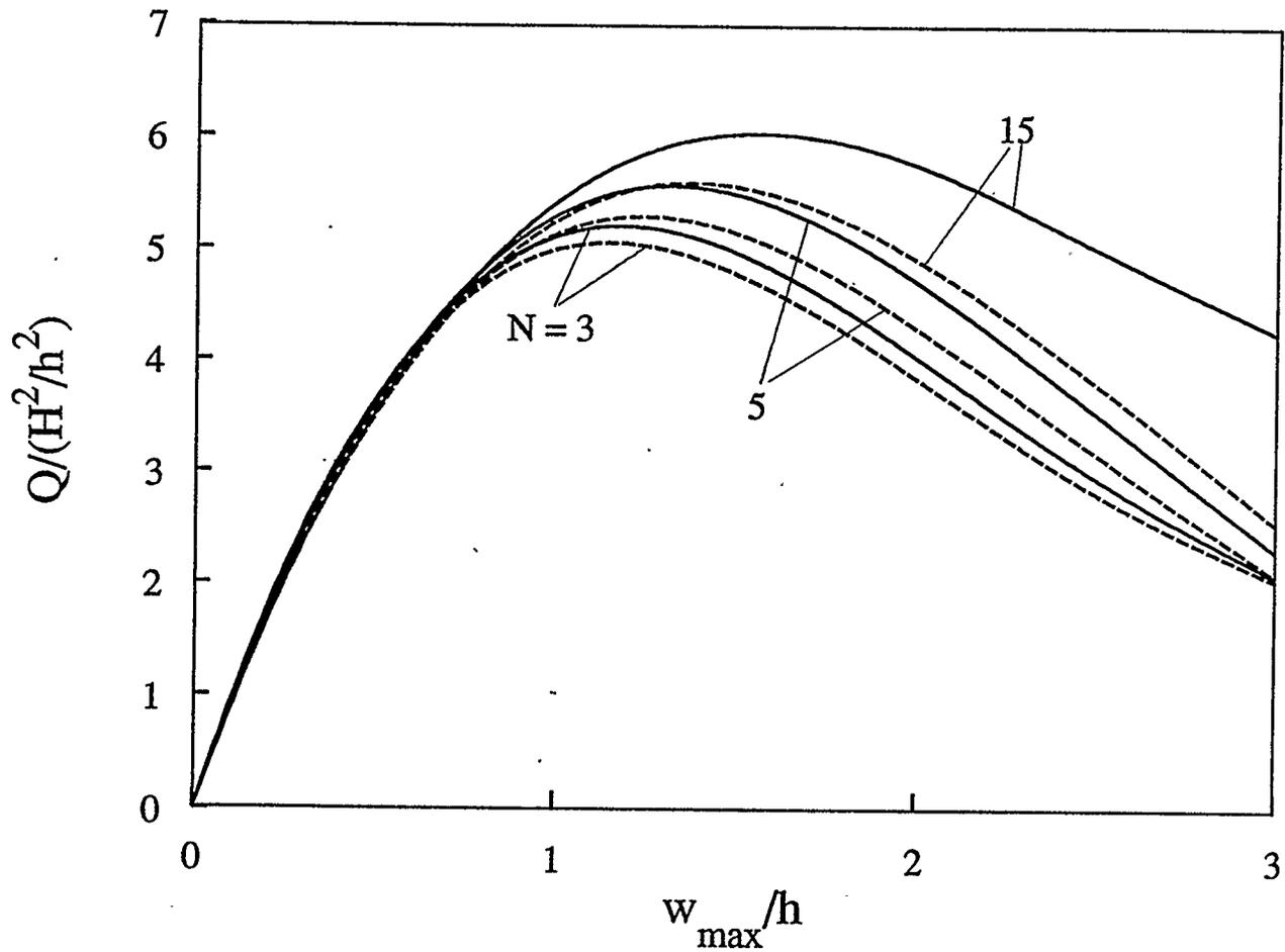
Figure 4.48: Effect of the number of layers on the postbuckling response of a movable simply-supported graphite-epoxy shallow spherical shell (  $a/h=15$ ,  $H/a=0.25$  )
