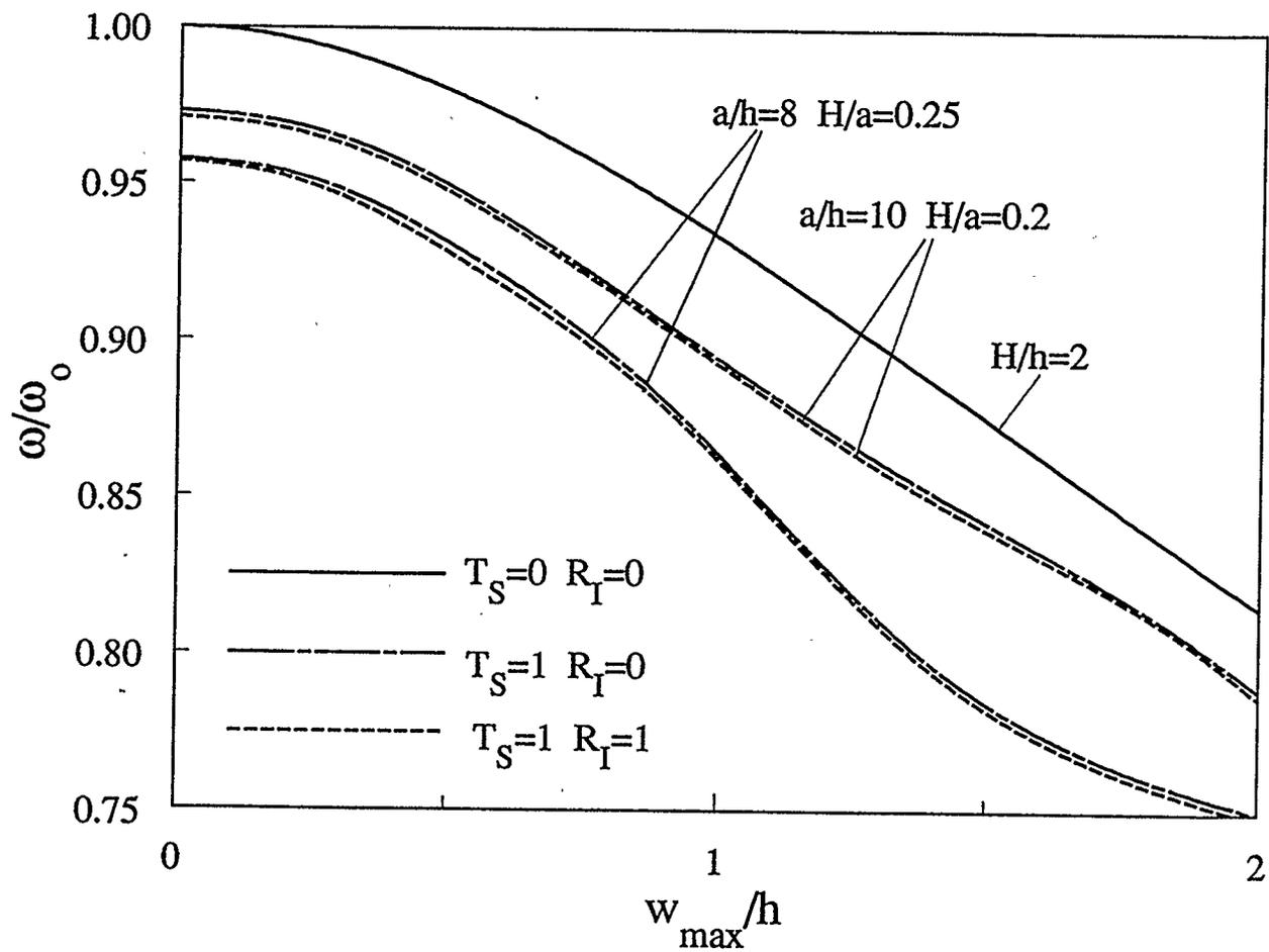
Figure 4.10: Individual effect of transverse shear and rotatory inertia on the frequency-amplitude response of a movable simply-supported five-layer graphite-epoxy shallow spherical shell
