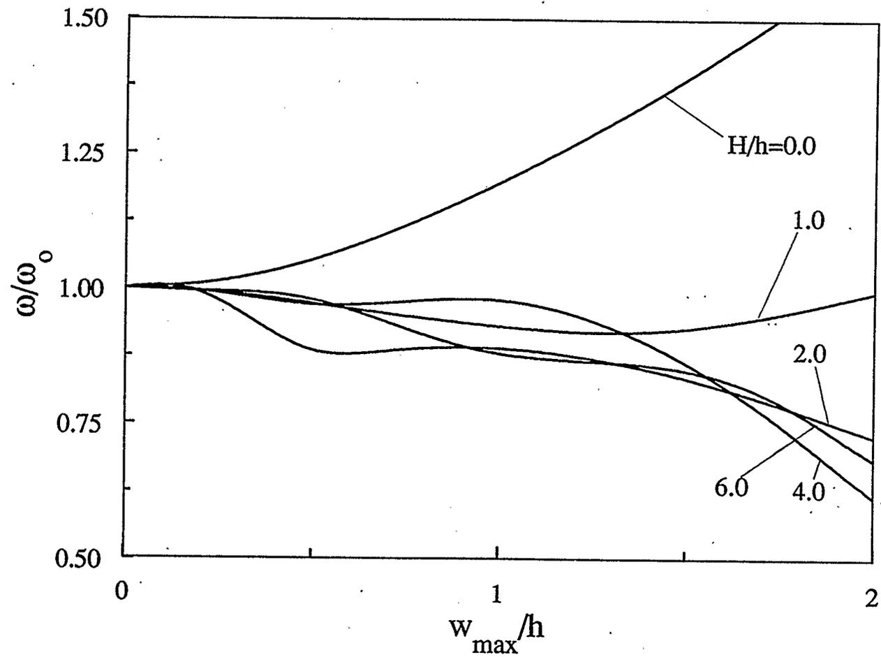
Figure 4.21: Effect of the shell rise on the frequency-amplitude response of an immovable clamped three-layer glass-epoxy shallow spherical shell (  $a/h=25$  )
