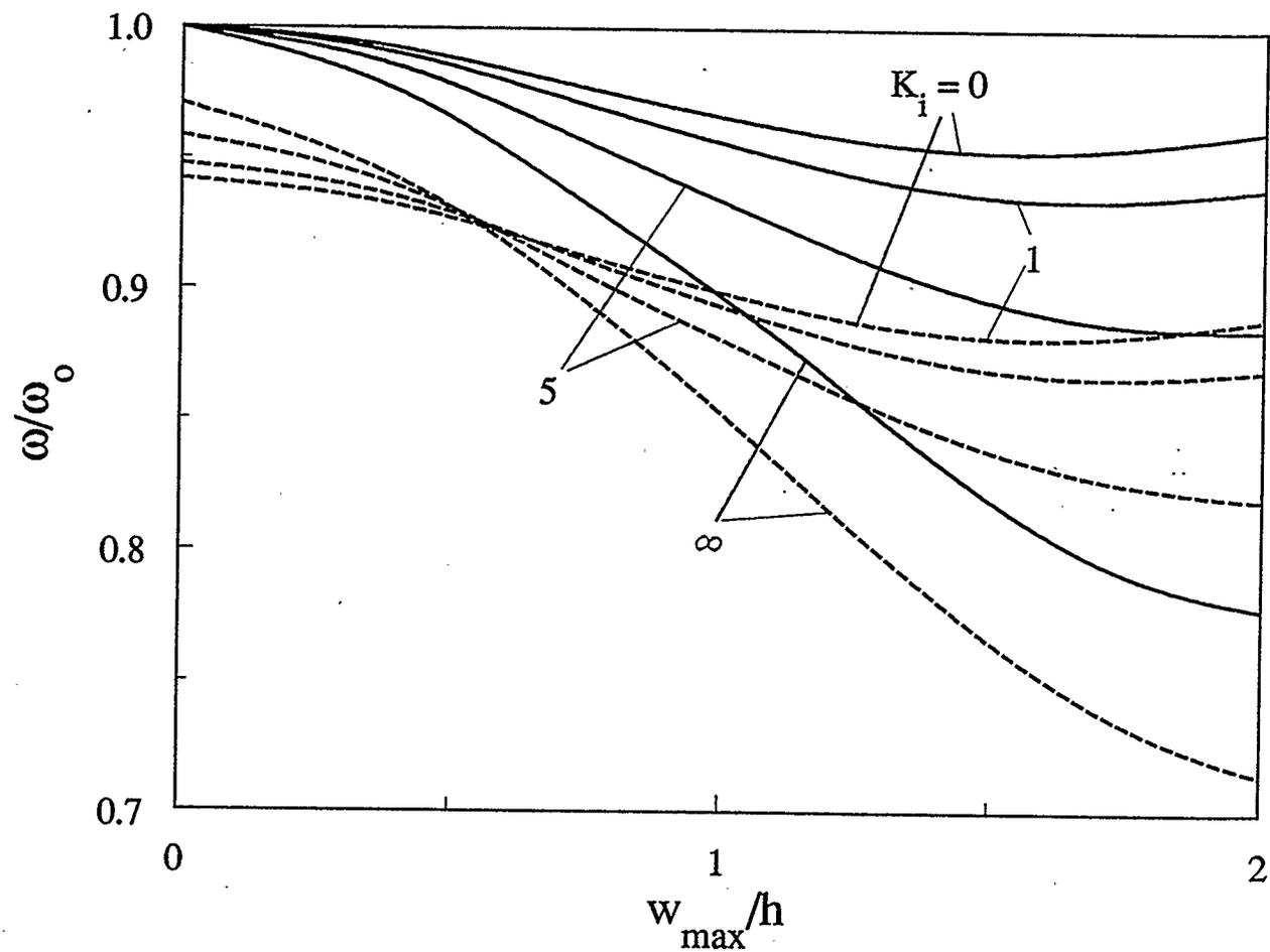
Figure 4.17: Effect of inplane edge stiffness on the frequency-amplitude response of a clamped five-layer graphite-epoxy shallow spherical shell ( $a/h=15$ ,  $H/a=0.1$ )
