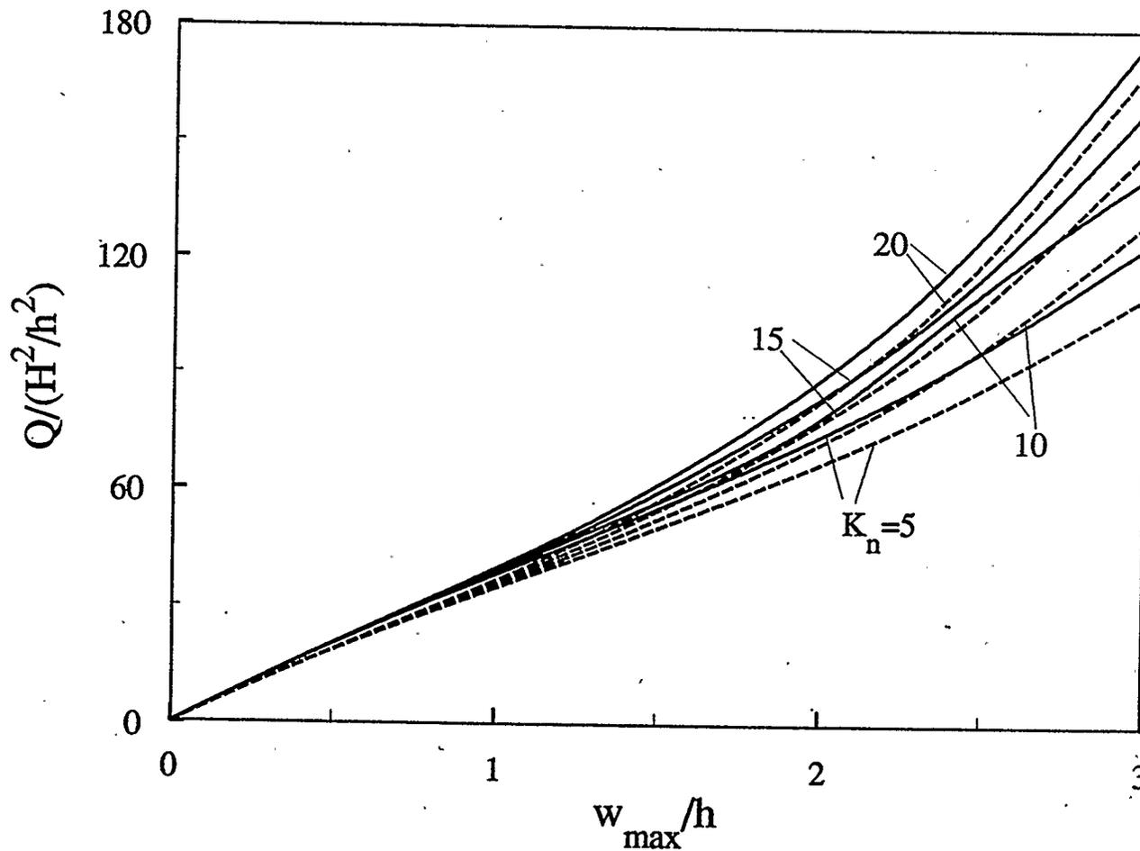
Figure 4.74: Effect of elastic foundation parameters on the postbuckling response of a movable four-layer graphite-epoxy imperfect shallow spherical shell
