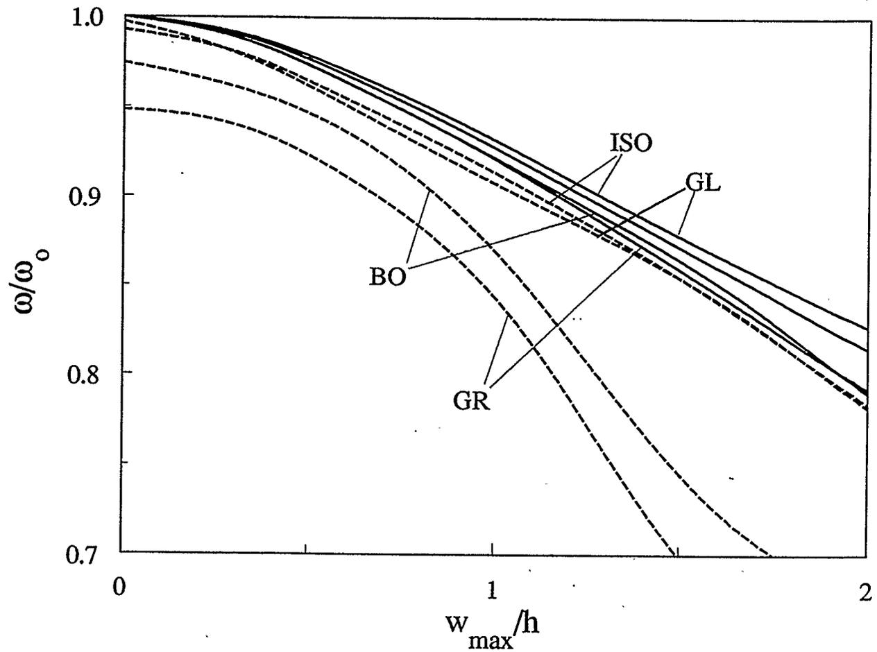
Figure 4.15: Effect of material properties on the frequency-amplitude response of an elastically supported five-layer shallow spherical shell ( $a/h=10$ ,  $H/a=0.2$ )
