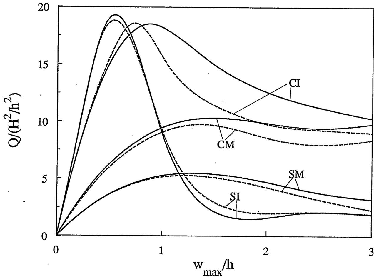
Figure 4.53: Effect of boundary conditions on the postbuckling response of a five-layer graphite-epoxy shallow spherical shell (  $a/h=15$ ,  $H/a=0.2$  )
