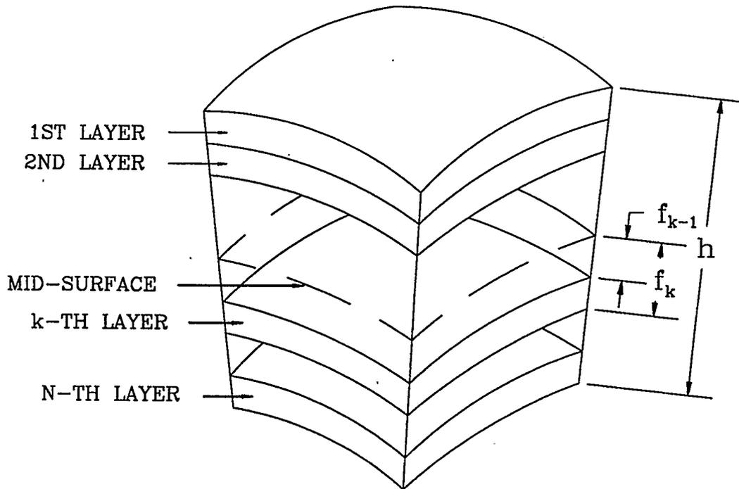
Figure 2.5: Structure of the laminated shell
