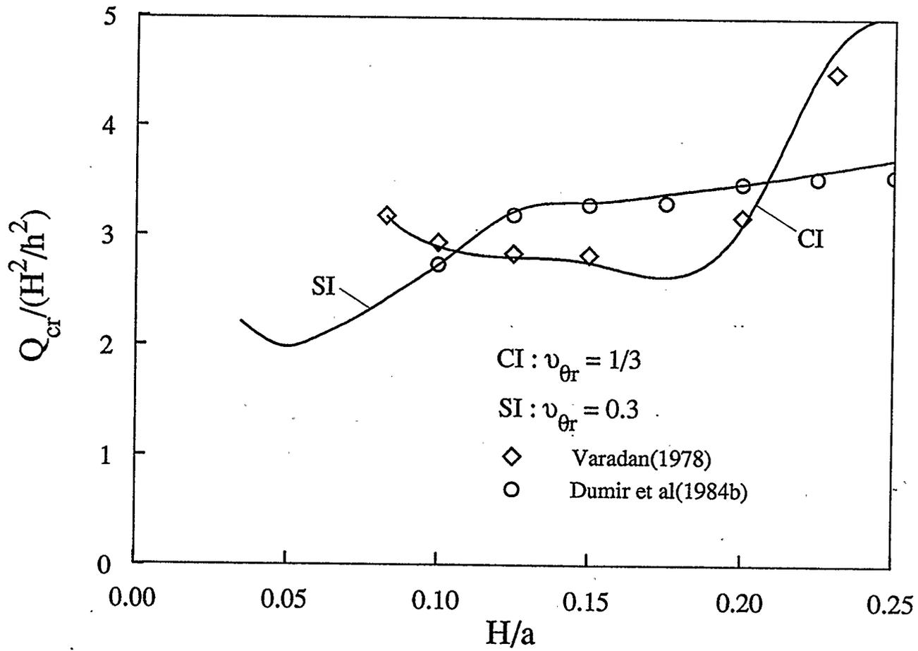
Figure 4.6: Comparison of buckling loads for immovable clamped(CI) and immovable simply-supported(SI) isotropic shallow spherical shells
