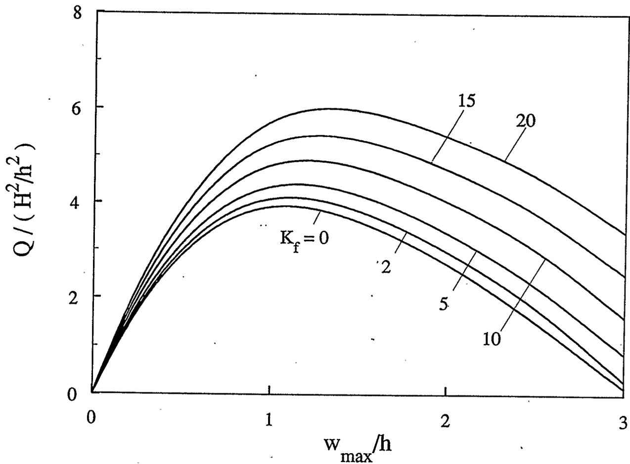
Figure 4.57: Effect of Winkler foundation parameter on the postbuckling response of an elastically supported five-layer glass-epoxy imperfect shallow spherical shell ( $K_b=2$ ,  $K_l=5$ ,  $\bar{W}_1=0.5$ ,  $K_n=5$ ,  $G_f=1$ ,  $a/h=15$ ,  $H/a=0.2$ )
