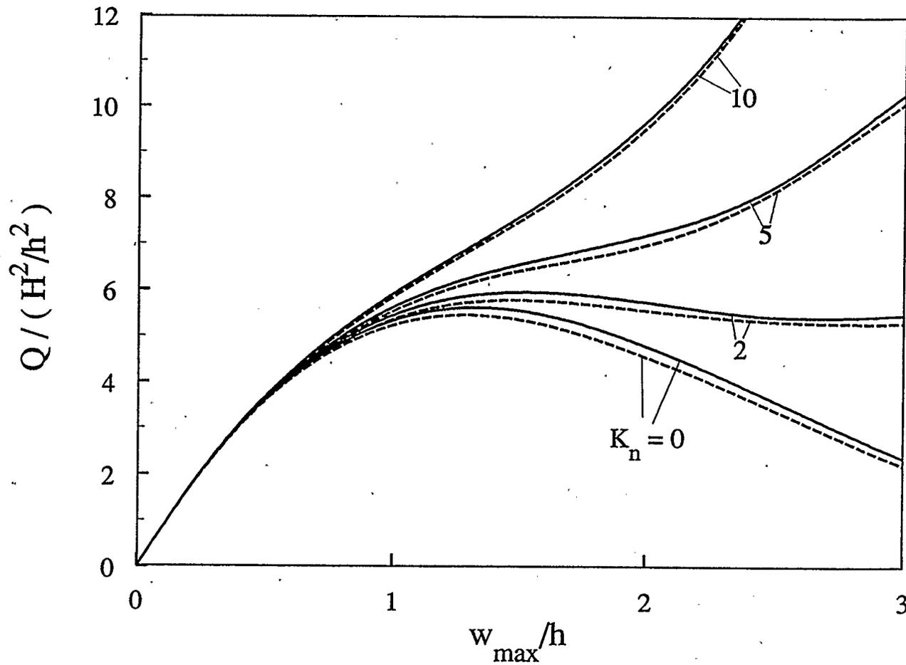
Figure 4.59: Effect of nonlinear Winkler foundation parameter on the postbuckling response of a movable simply-supported five-layer graphite-epoxy shallow spherical shell ( $K_f=0$ ,  $G_f=0$ ,  $a/h=20$ ,  $H/a=0.2$ )
