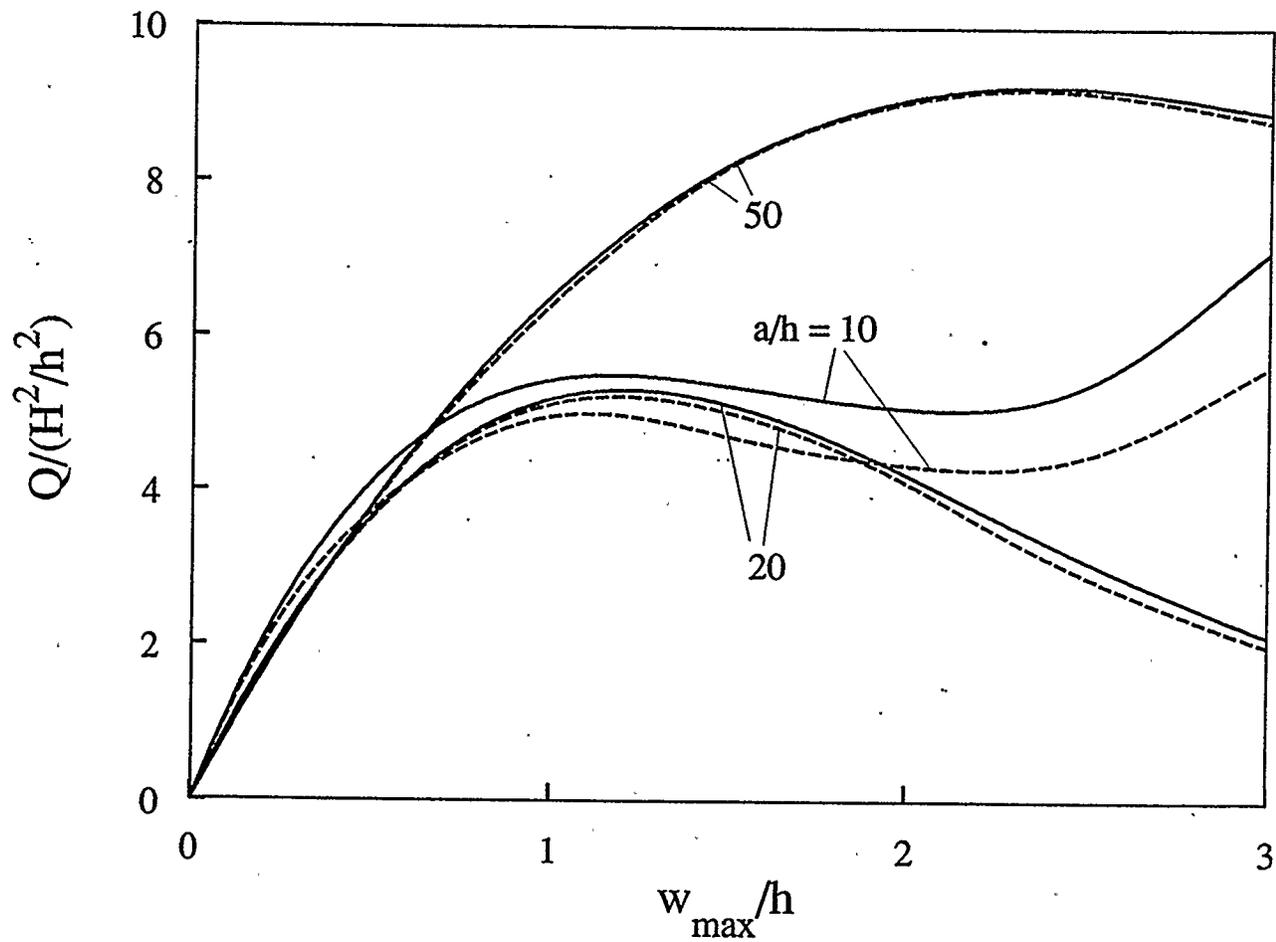
Figure 4.45: Effect of the base radius-to-thickness ratio on the postbuckling response of a movable simply-supported three-layer graphite-epoxy shallow spherical shell ( $H/a=0.2$ )
