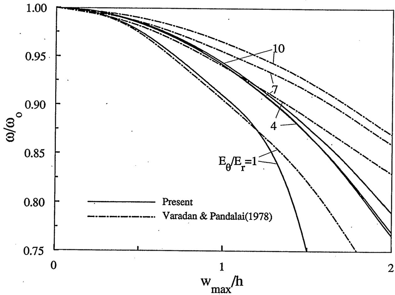
Figure 4.2: Comparison of the frequency-amplitude response for an immovable clamped orthotropic shallow spherical shell with different material properties ( $H/h = 3, \nu_{\theta r} = 1/3$ )
