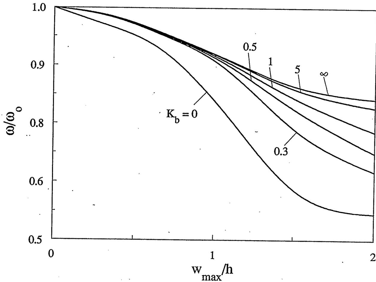
Figure 4.18: Effect of rotational edge stiffness on the frequency-amplitude response of an elastically supported three-layer boron-epoxy shallow spherical shell ( $K_1=5$ ,  $a/h=10$ ,  $H/a=0.15$ )
