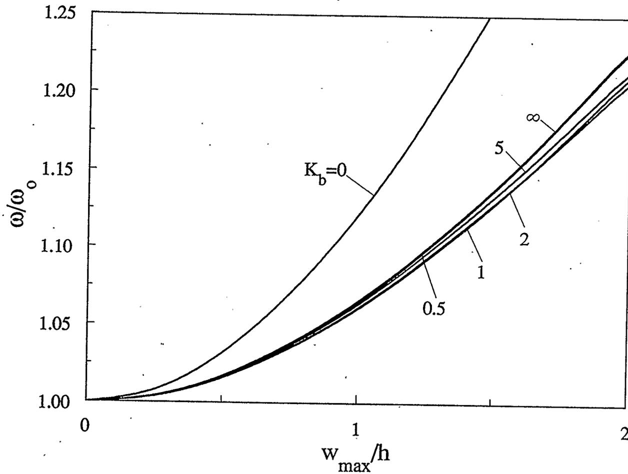
Figure 4.39: Effect of rotational edge stiffness on the frequency-amplitude response of a six-layer glass-epoxy circular plate with a movable edge ( $a/h=15$ )
