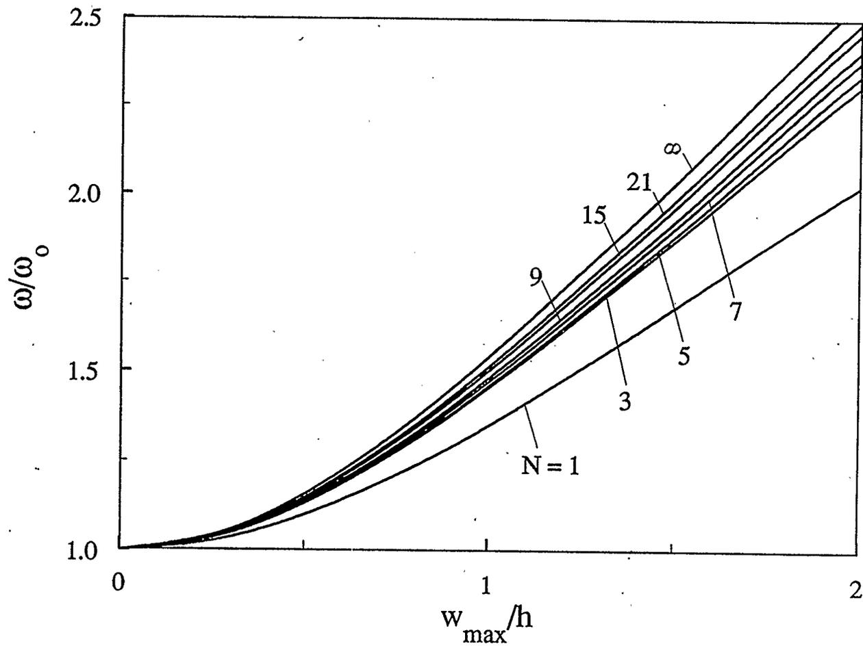
Figure 4.28: Effect of the number of layers on the frequency-amplitude response of an immovable simply-supported boron-epoxy circular plate (  $a/h=12$  )
