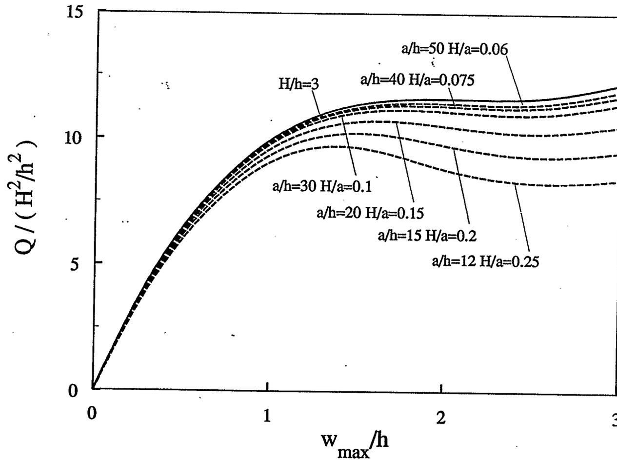
Figure 4.68: Effect of the base radius-to-thickness ratio on the postbuckling response of a movable clamped four-layer graphite-epoxy shallow spherical shell
