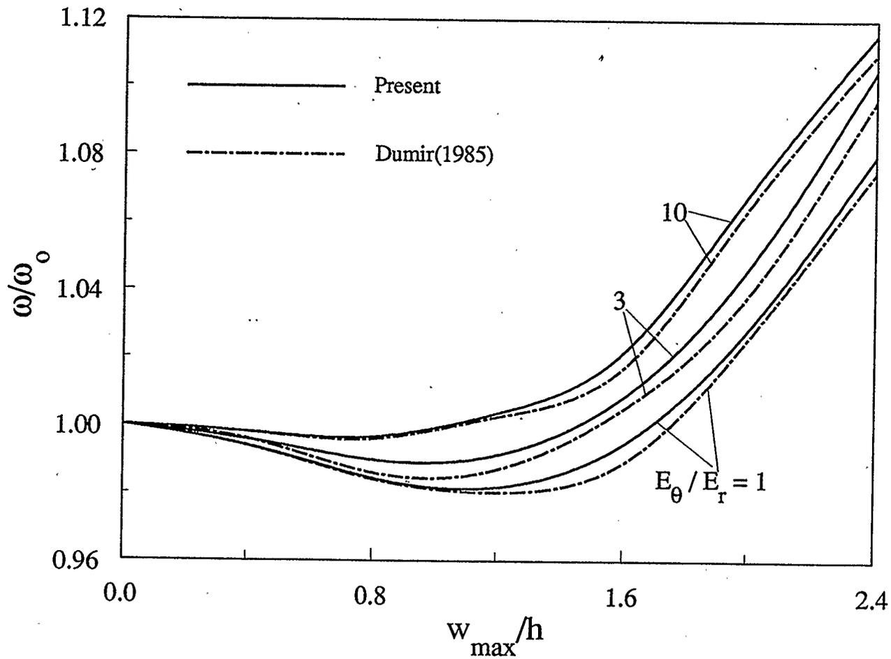
Figure 4.3: Comparison of the frequency-amplitude response for an immovable clamped orthotropic shallow spherical shell resting on elastic foundations
