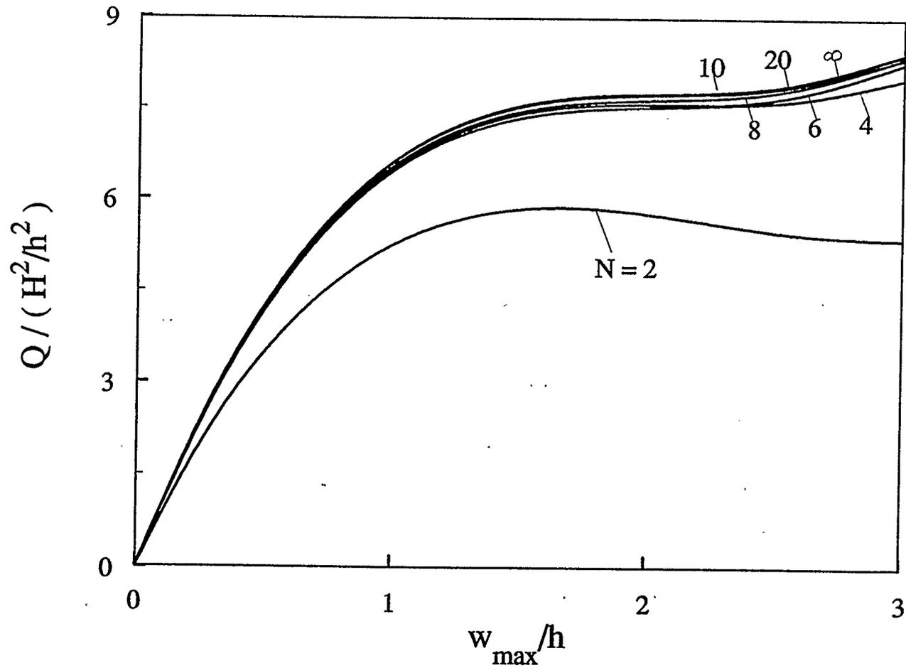
Figure 4.69: Effect of the number of layers on the postbuckling response of a movable clamped boron-epoxy shallow spherical shell (  $a/h=50$ ,  $H/a=0.06$  )
