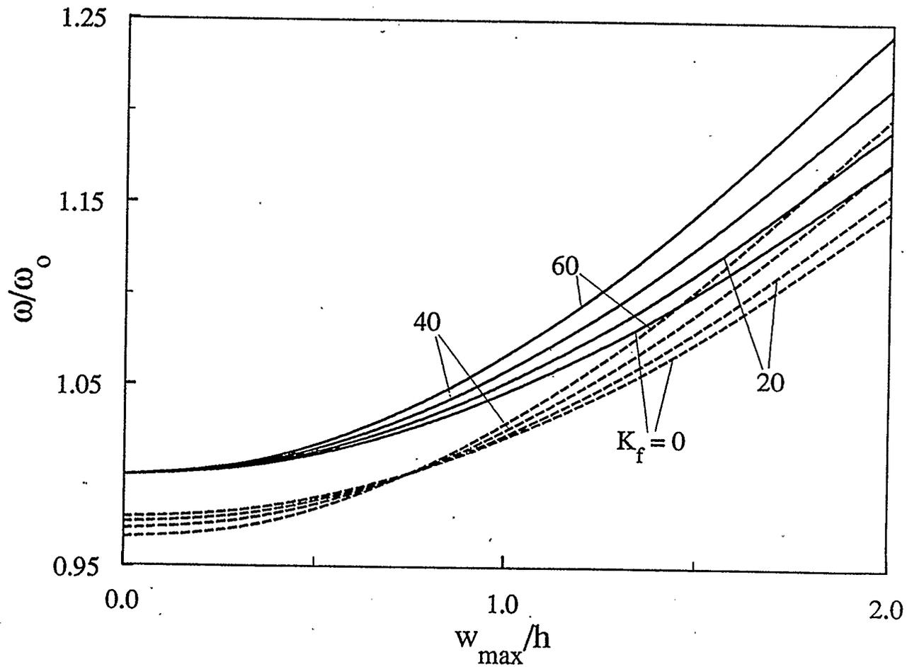
Figure 4.33: Effect of Winkler foundation parameter on the frequency-amplitude response of an elastically supported three-layer graphite-epoxy imperfect circular plate ( $K_b=3$ ,  $K_l=5$ ,  $\bar{W}_1=0.1$ ,  $K_n=10$ ,  $G_f=15$ ,  $a/h=10$ )
