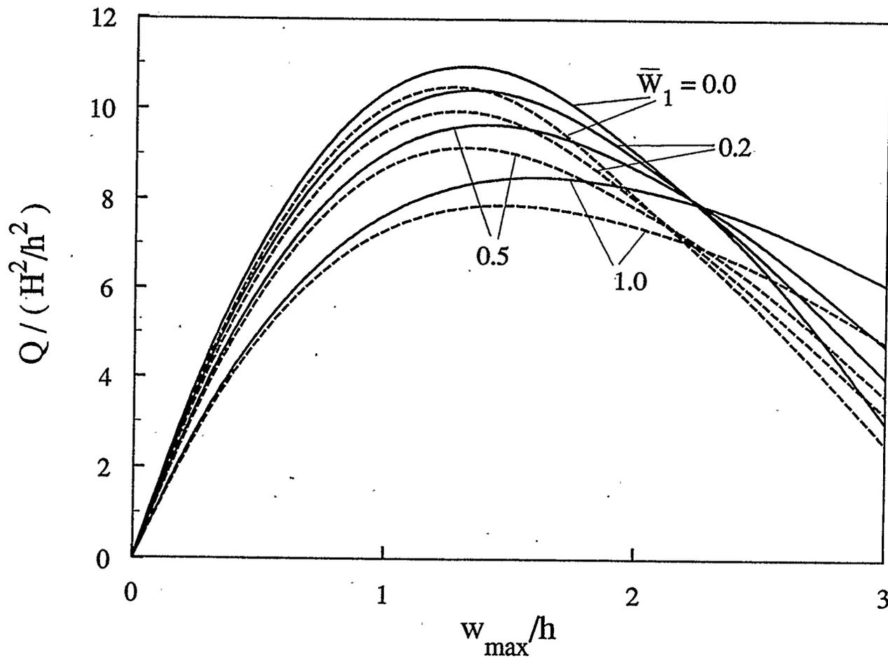
Figure 4.56: Effect of geometrically initial imperfection on the postbuckling response of a movable clamped five-layer graphite-epoxy shallow spherical shell resting on elastic foundations ( $K_f=5$ ,  $K_n=10$ ,  $G_f=0$ ,  $a/h=20$ ,  $H/a=0.2$ )
