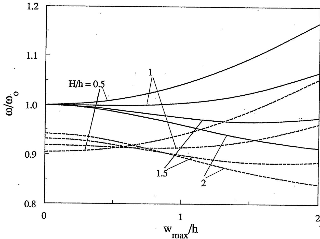
Figure 4.40: Effect of the shell rise on the frequency-amplitude response of a movable clamped four-layer boron-epoxy shallow spherical shell (  $a/h=10$  )
