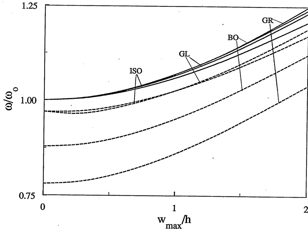
Figure 4.29: Effect of material properties on the frequency-amplitude response of an elastically supported seven-layer circular plate ( $a/h=8$ )
