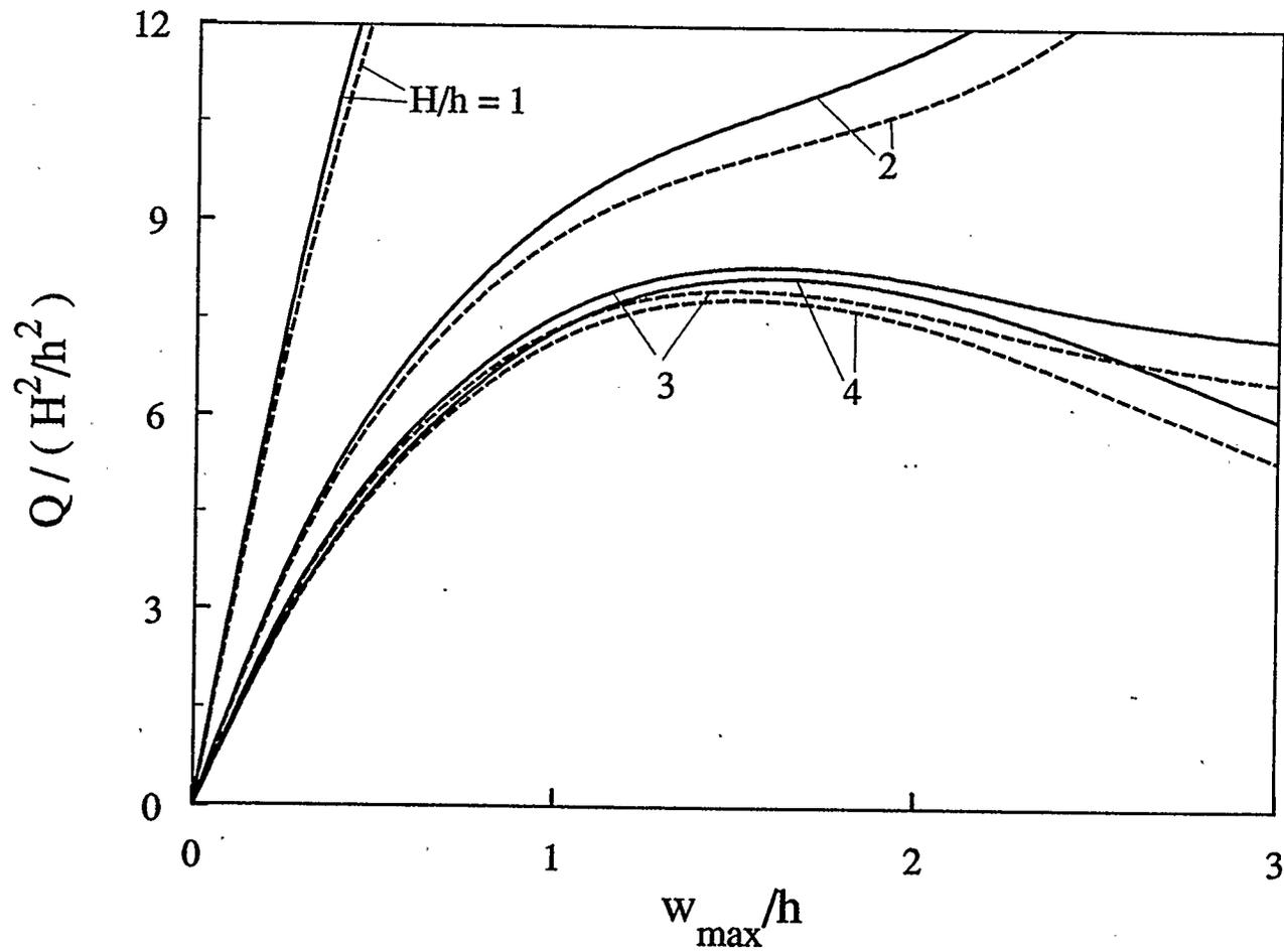
Figure 4.72: Effect of the shell rise on the postbuckling response of a movable clamped two-layer graphite-epoxy shallow spherical shell (  $a/h=20$  )
