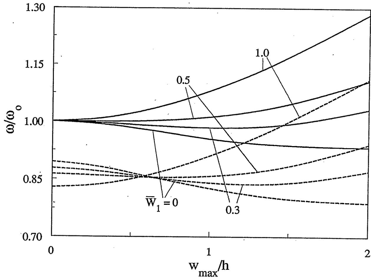
Figure 4.22: Effect of geometrically initial imperfection on the frequency-amplitude response of an elastically supported seven-layer graphite-epoxy shallow spherical shell ( $K_p = \infty$ ,  $K_1 = 2$ ,  $a/h = 10$ ,  $H/a = 0.15$ )
