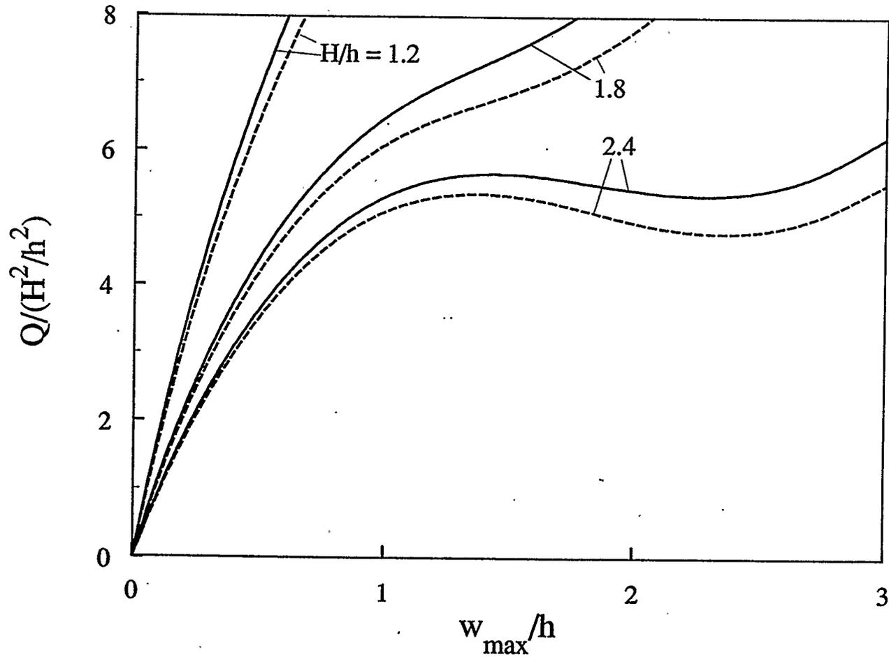
Figure 4.54: Effect of the shell rise on the postbuckling response of an elastically supported three-layer boron-epoxy shallow spherical shell ( $K_p=2$ ,  $K_1=0$ ,  $a/h=12$ )
