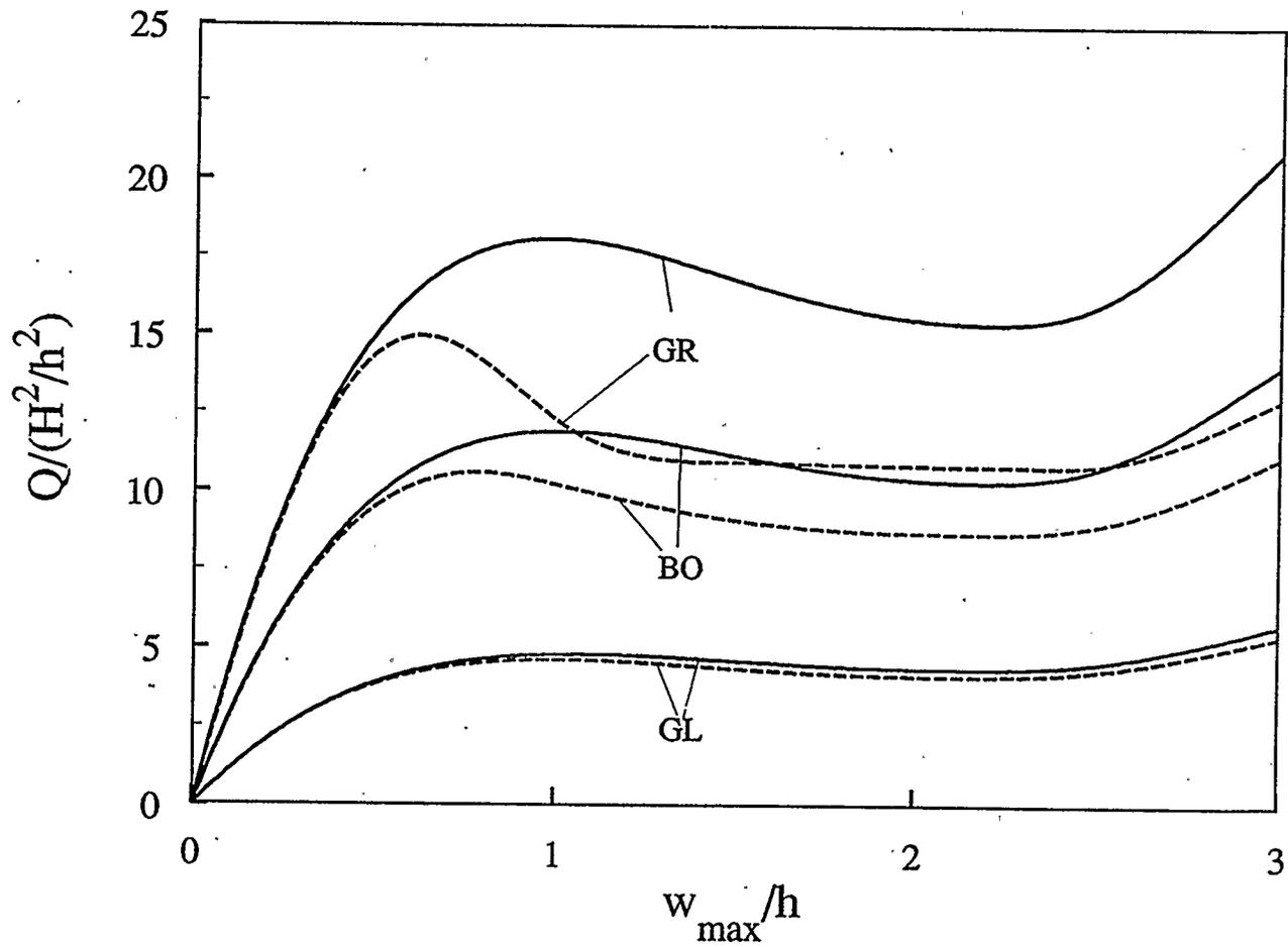
Figure 4.49: Effect of material properties on the postbuckling response of an immovable clamped five-layer shallow spherical shell (  $a/h=10$ ,  $H/a=0.2$  )
