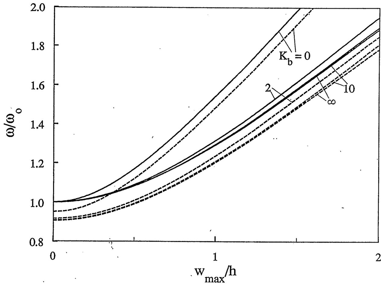
Figure 4.30: Effect of rotational edge stiffness on the frequency-amplitude response of a three-layer graphite-epoxy circular plate with an immovable edge ( $a/h=12$ )
