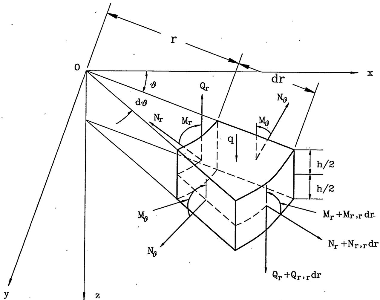
Figure 2.6: Shell element with stress resultants and couples
