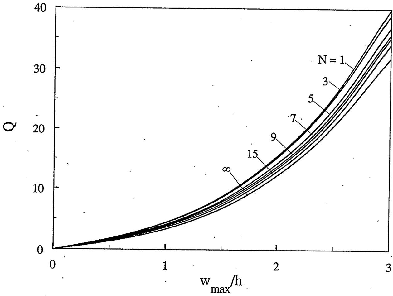
Figure 4.61: Effect of the number of layers on the static large-deflection response of a movable simply-supported glass-epoxy circular plate (  $a/h=12$  )
