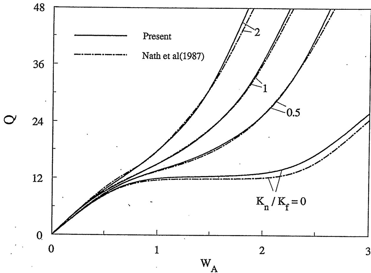
Figure 4.8: Comparison of the static large deflection of an immovable simply-supported orthotropic shallow spherical shell with different values of nonlinear Winkler foundation parameters ( $E_\theta/E_r=1.5$ ,  $\nu_{\theta r}=1/3$ ,  $K_f=9$ ,  $G_f=0$ ,  $H/h=1.5$ )
