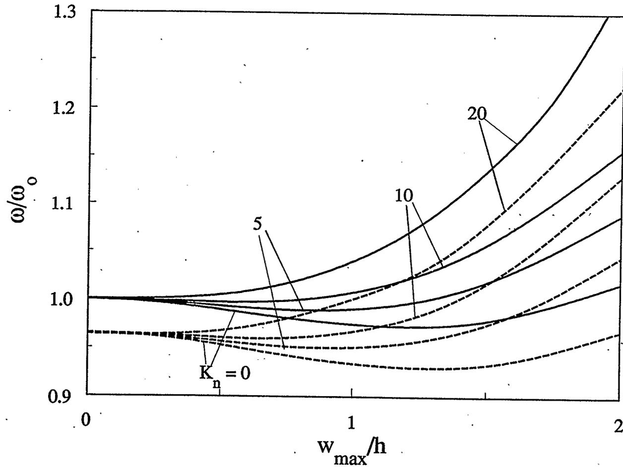
Figure 4.26: Effect of nonlinear Winkler foundation parameter on the frequency-amplitude response of an elastically supported three-layer graphite-epoxy imperfect shallow spherical shell ( $K_b=2$ ,  $K_t=3$ ,  $\bar{W}_1=0.2$ ,  $K_f=5$ ,  $G_f=2$ ,  $a/h=12$ ,  $H/a=0.1$ )
