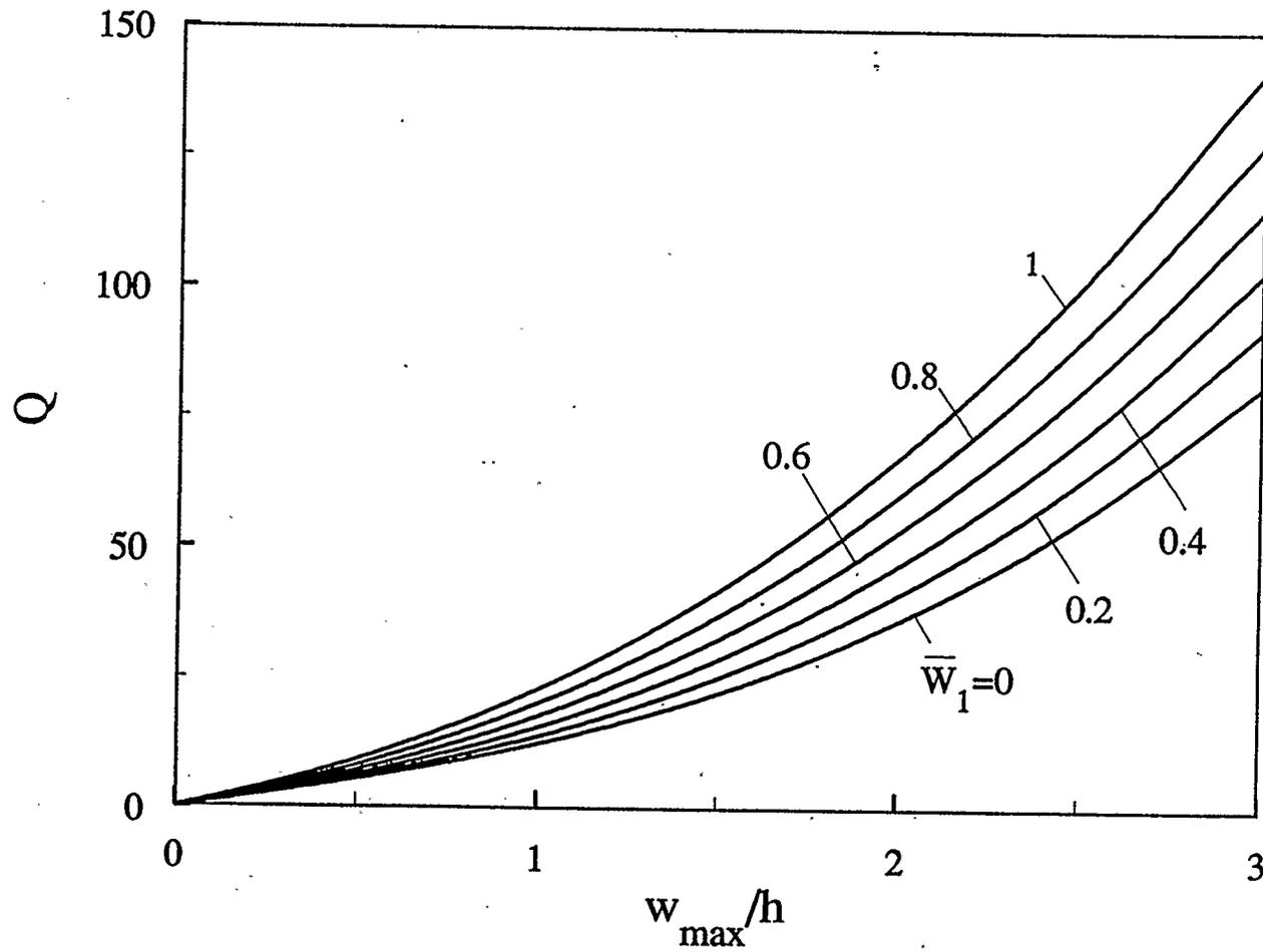
Figure 4.73: Effect of geometrically initial imperfections on the static large-deflection response of a movable clamped four-layer glass-epoxy circular plate (  $a/h=15$  )
