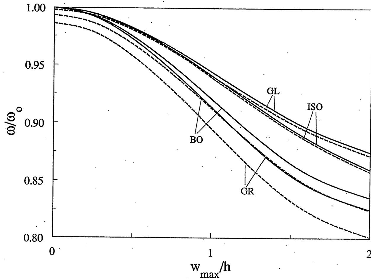
Figure 4.16: Effect of material properties on the frequency-amplitude response of a movable simply-supported three-layer shallow spherical shell ( $a/h=15$ ,  $H/a=0.1$ )
