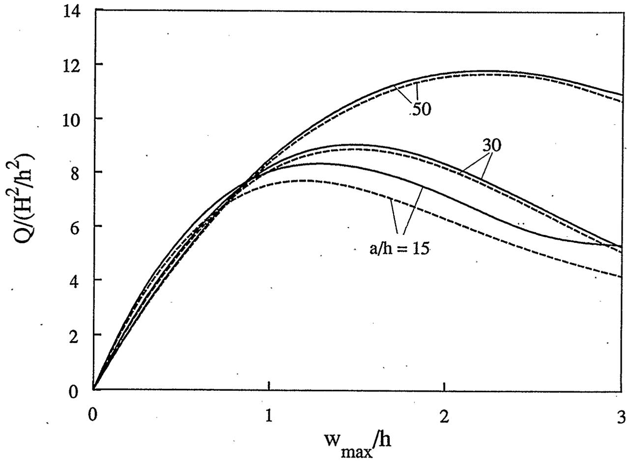
Figure 4.46: Effect of the base radius-to-thickness ratio on the postbuckling response of a movable clamped three-layer graphite-epoxy shallow spherical shell ( $H/a=0.2$ )
