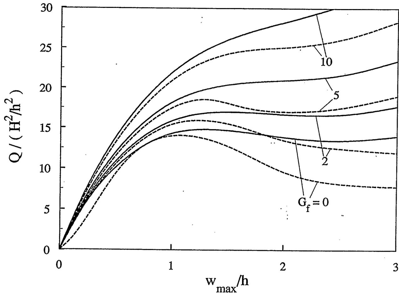
Figure 4.58: Effect of Pasternak foundation parameter on the postbuckling response of an elastically supported seven-layer graphite-epoxy shallow spherical shell ( $K_b=10, K_t=5, K_f=5, K_n=0, a/h=10, H/a=0.25$ )
