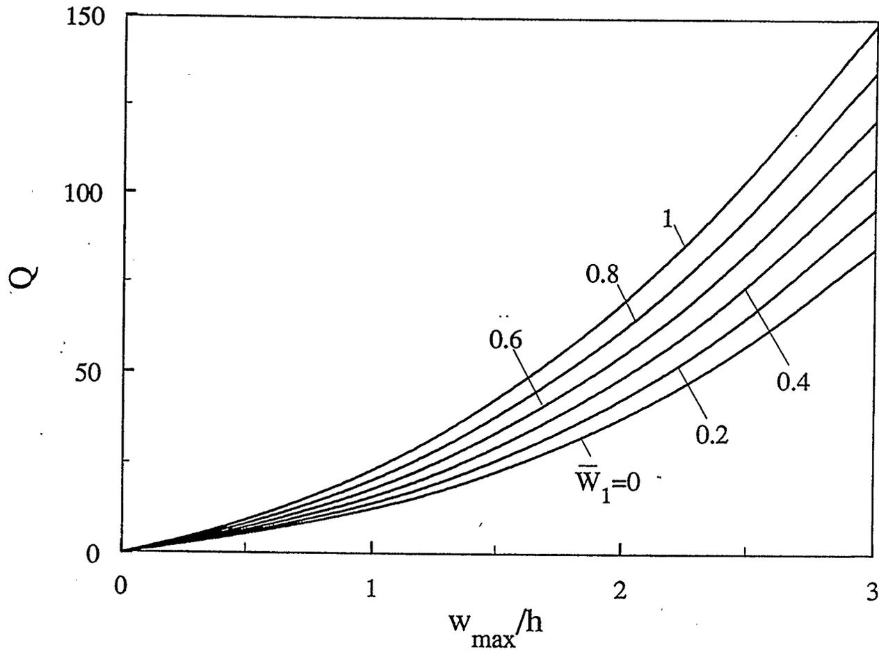
Figure 4.65: Effect of geometrically initial imperfections on static the large-deflection response of a movable clamped five-layer glass-epoxy circular plate (  $a/h=20$  )
