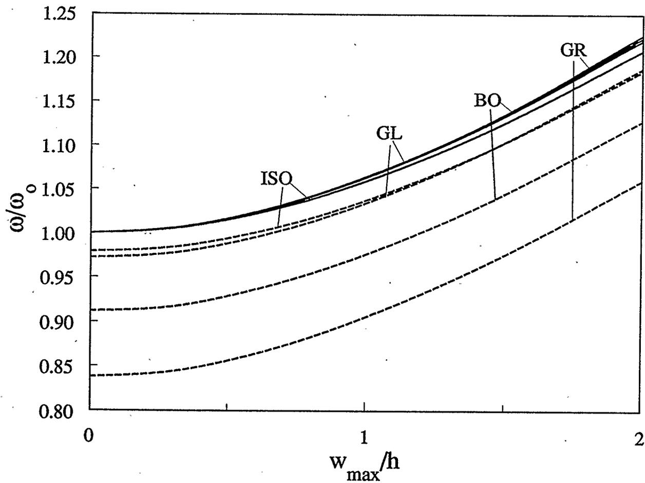
Figure 4.38: Effect of material properties on the frequency-amplitude response of an elastically supported six-layer circular plate (  $a/h=10$  )
