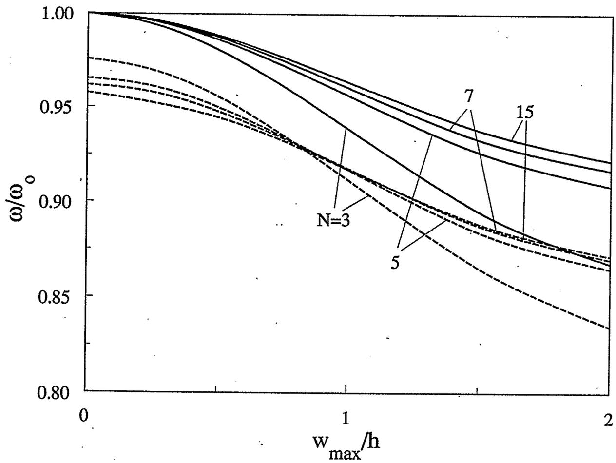
Figure 4.13: Effect of the number of layers on the frequency-amplitude response of an elastically supported boron-epoxy shallow spherical shell ( $K_p=5$ ,  $K_t=0$ ,  $a/h=12$ ,  $H/a=0.15$ )
