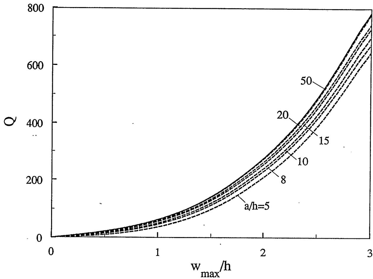
Figure 4.60: Effect of the base radius-to-thickness ratio on the static large-deflection response of an immovable clamped five-layer graphite-epoxy circular plate
