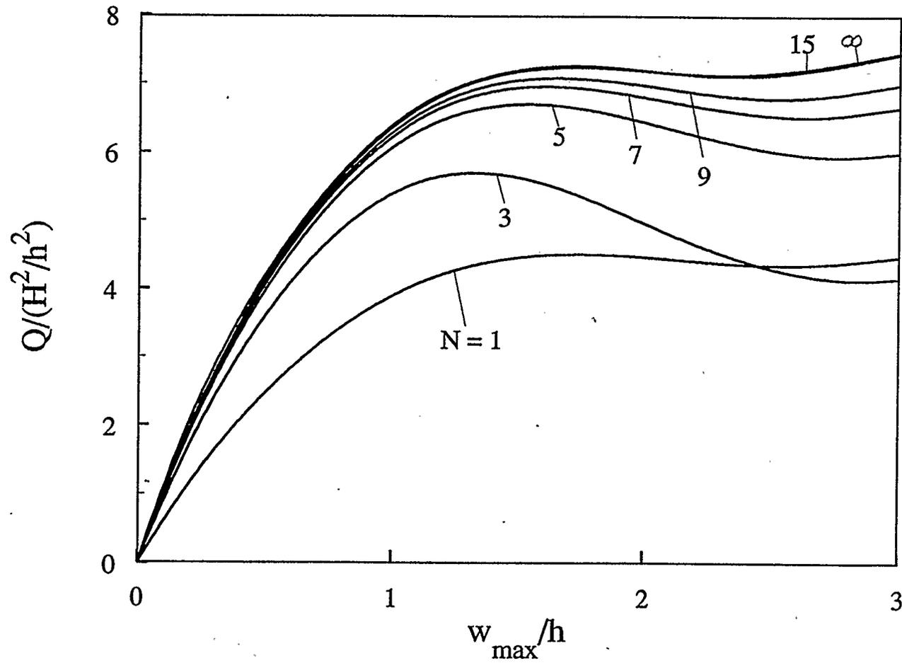
Figure 4.47: Effect of the number of layers on the postbuckling response of a movable clamped boron-epoxy shallow spherical shell (  $a/h=30$ ,  $H/a=0.1$  )
