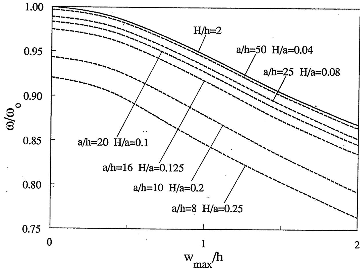
Figure 4.36: Effect of the base radius-to-thickness ratio on the frequency-amplitude response of a movable clamped two-layer graphite-epoxy shallow spherical shell
