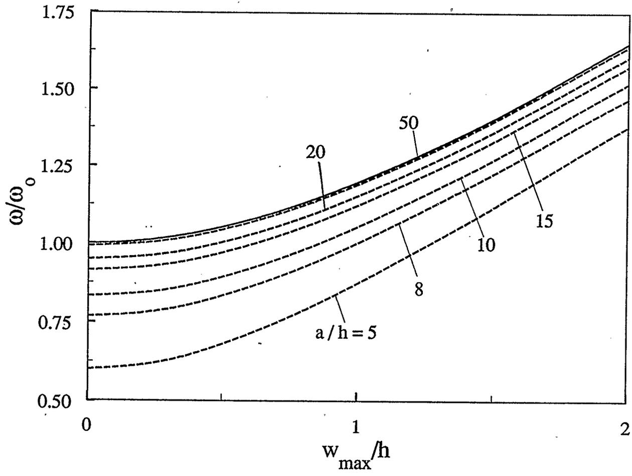
Figure 4.27: Effect of the base radius-to-thickness ratio on the frequency-amplitude response of an immovable clamped five-layer graphite-epoxy circular plate
