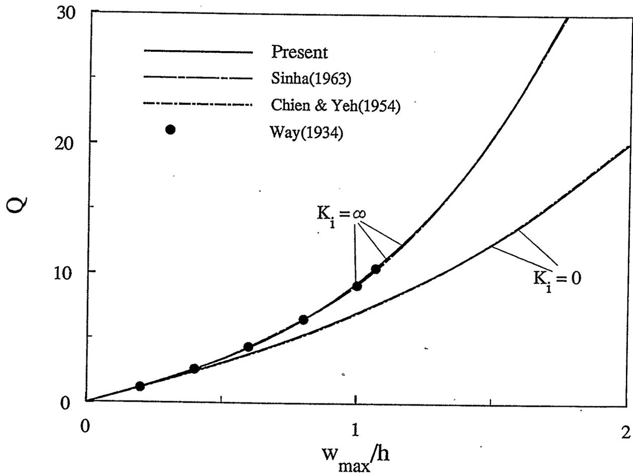
Figure 4.9: Comparison of the static large deflection of immovable and movable clamped isotropic circular plates ( $\nu_{\theta r} = 0.3$ )
