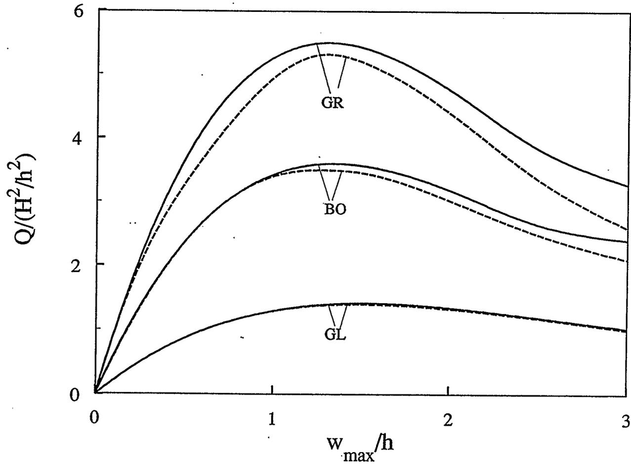
Figure 4.50: Effect of material properties on the postbuckling response of a movable simply-supported five-layer shallow spherical shell (  $a/h=20$ ,  $H/a=0.15$  )
