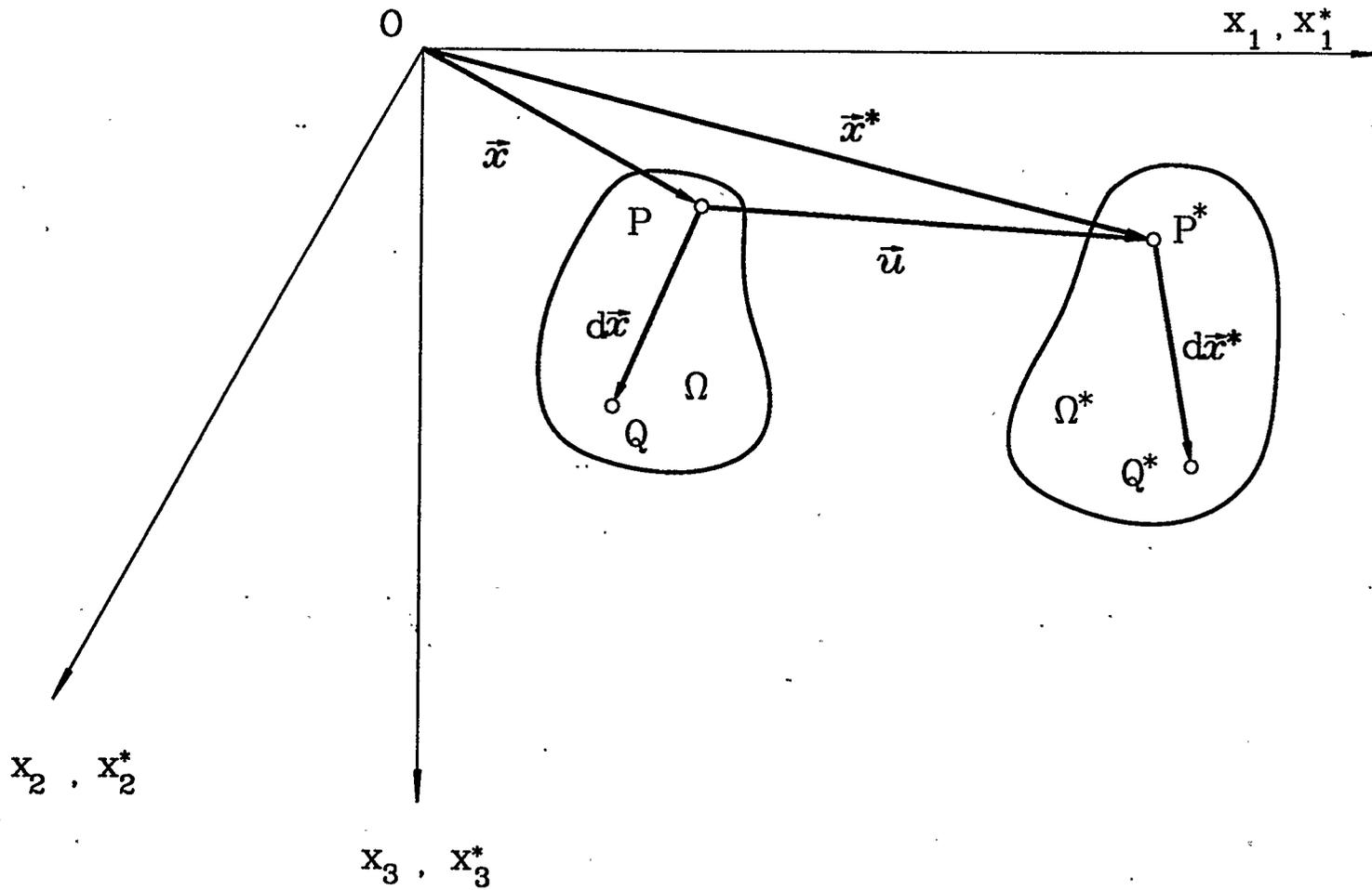
Figure 2.2: Deformation of a line element
