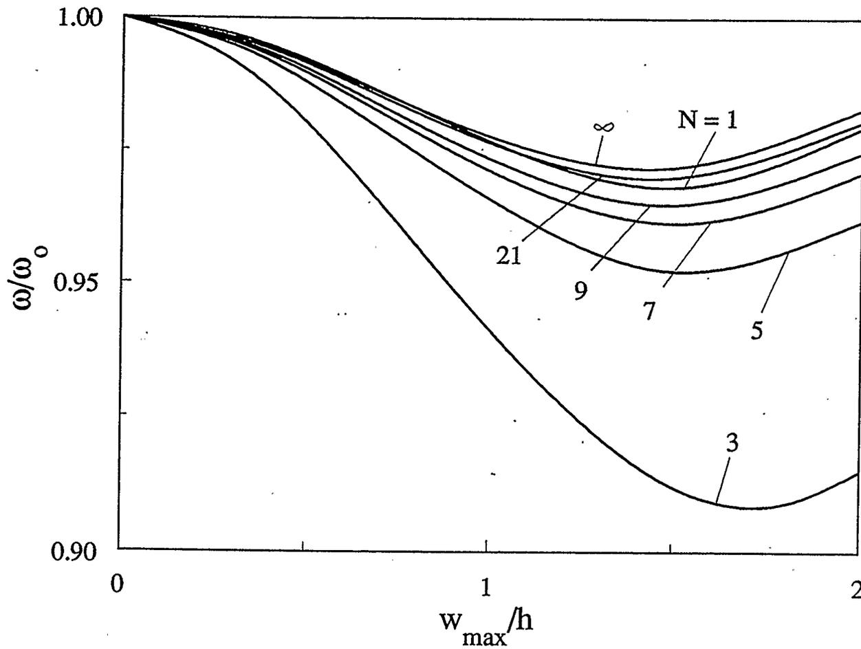
Figure 4.14: Effect of the number of layers on the frequency-amplitude response of a movable clamped graphite-epoxy shallow spherical shell ( $a/h=15$ ,  $H/a=0.1$ )
