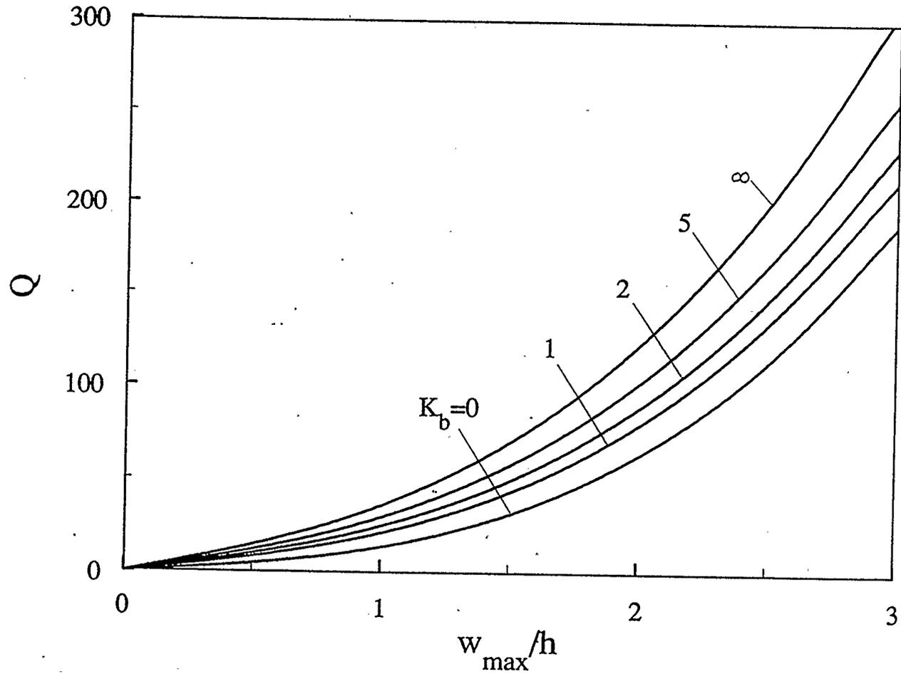
Figure 4.63: Effect of rotational edge stiffness on the static large-deflection response of an elastically supported seven-layer boron-epoxy circular plate ( $K_1=2$ ,  $a/h=10$ )
