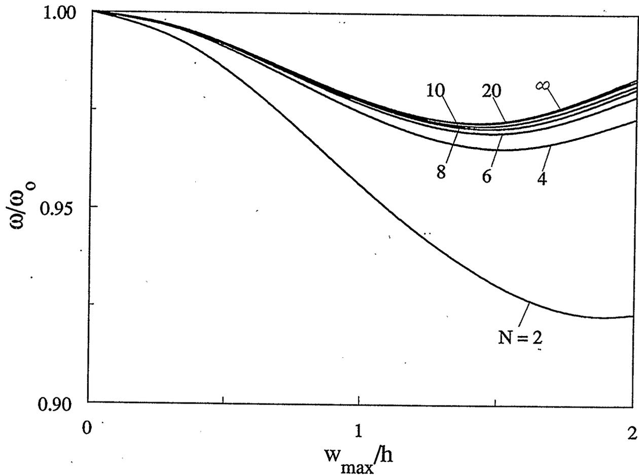
Figure 4.37: Effect of the number of layers on the frequency-amplitude response of a movable clamped glass-epoxy shallow spherical shell (  $a/h=15, H/a=0.1$  )
