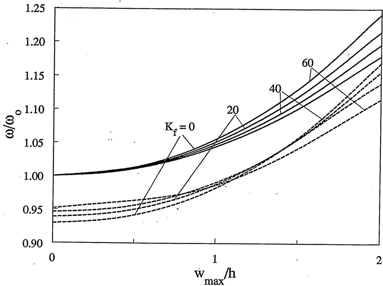
Figure 4.24: Effect of Winkler foundation parameter on the frequency-amplitude response of an immovable clamped five-layer graphite-epoxy shallow spherical shell ( $K_n=5$ ,  $G_f=10$ ,  $a/h=10$ ,  $H/a=0.05$ )
