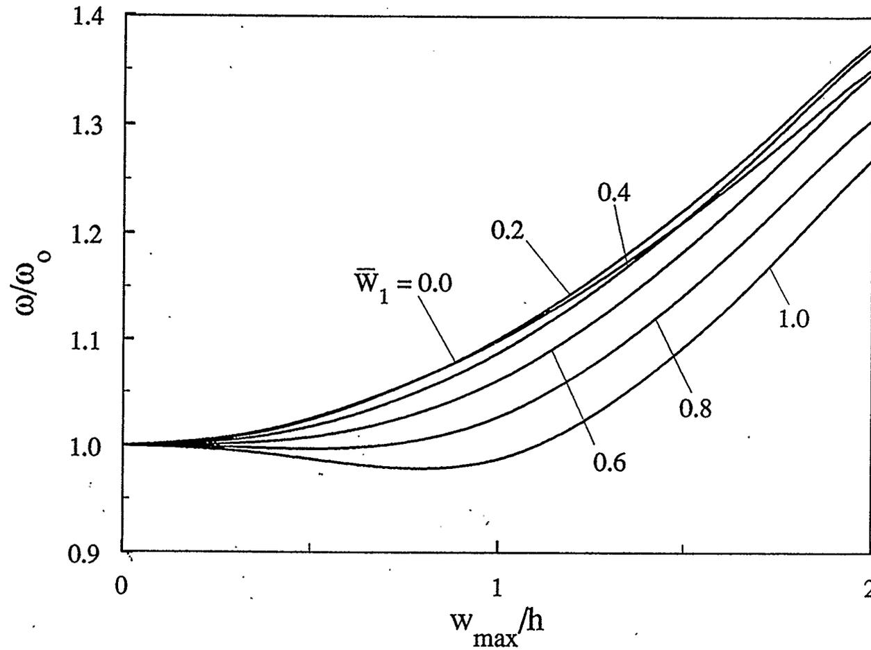
Figure 4.32: Effect of geometrically initial imperfections on the frequency-amplitude response of a movable simply-supported five-layer glass-epoxy circular plate (  $a/h=15$  )
