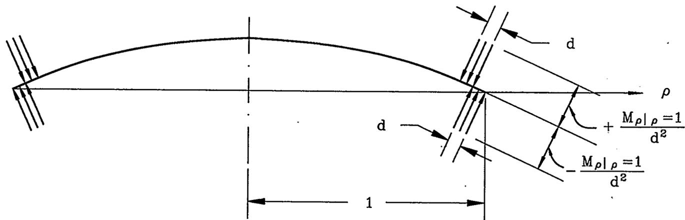
Figure 3.1: Equivalent pressure distribution (  $d \rightarrow 0$  ) for edge moment
