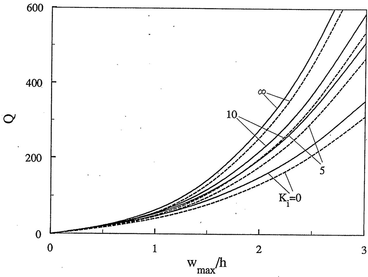
Figure 4.64: Effect of inplane edge stiffness on the static large-deflection response of a five-layer graphite-epoxy circular plate with a clamped edge (  $a/h=15$  )
