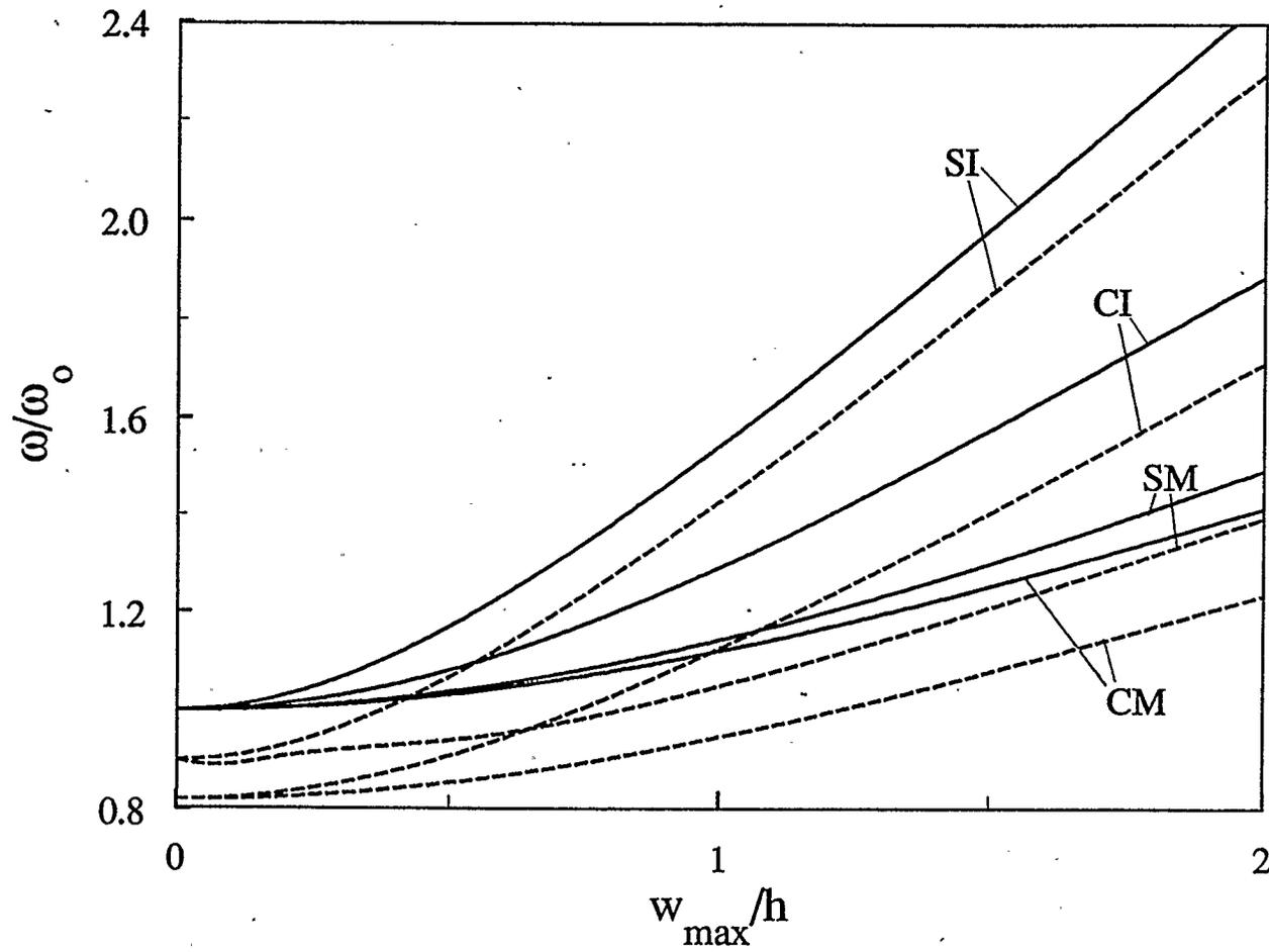
Figure 4.31: Effect of boundary conditions on the frequency-amplitude response of a three-layer graphite-epoxy circular plate (  $a/h=8$  )
