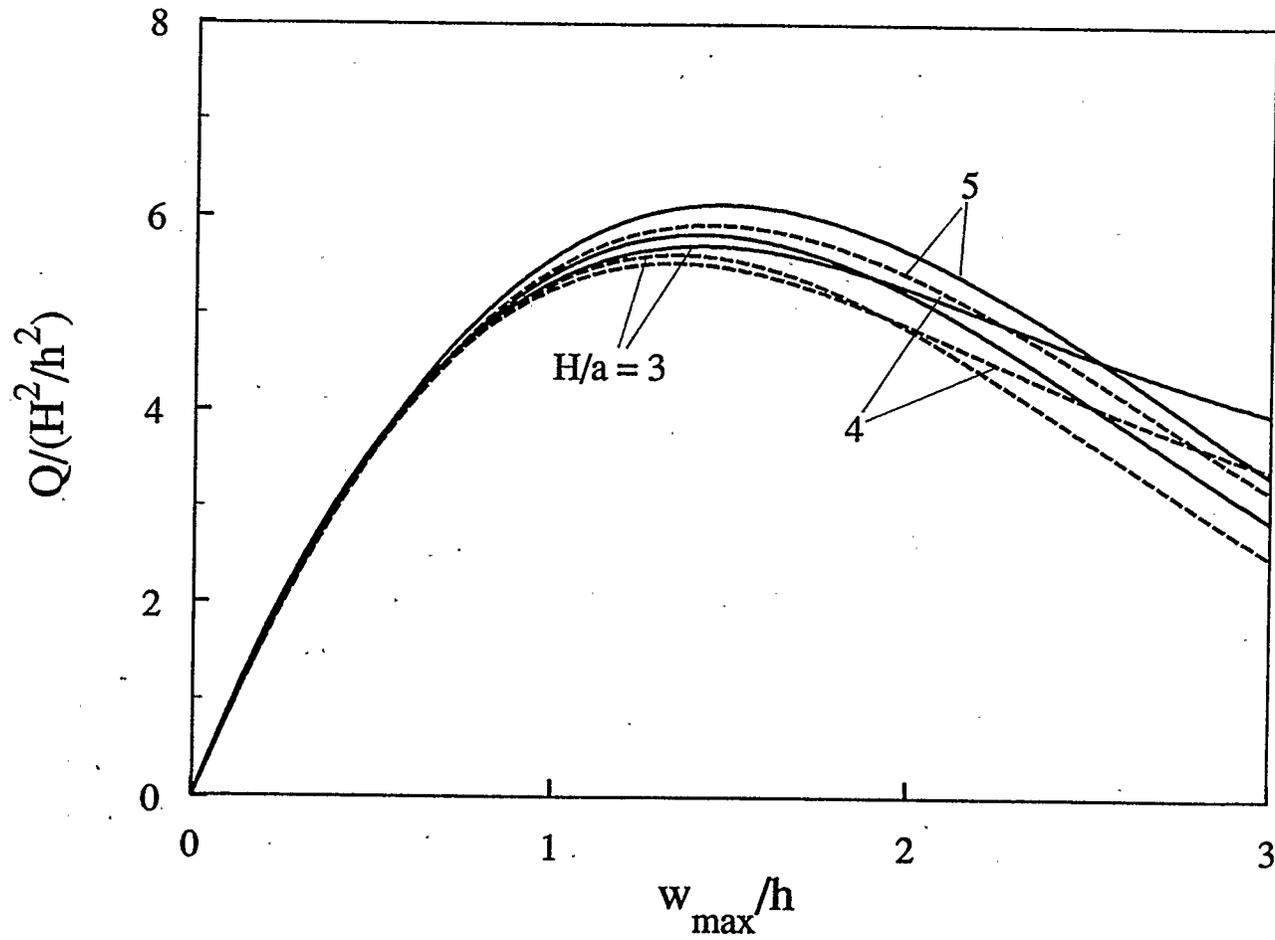
Figure 4.55: Effect of the shell rise on the postbuckling response of a movable simply-supported seven-layer graphite-epoxy shallow spherical shell (  $a/h=20$  )
