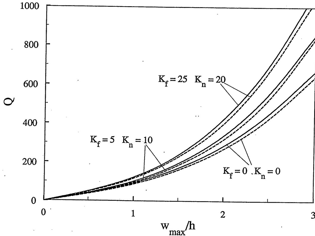
Figure 4.66: Effect of elastic foundations on the static large-deflection response of an immovable clamped five-layer glass-epoxy imperfect circular plate ( $\bar{W}_1=0.1, G_f=10, a/h=10$ )
