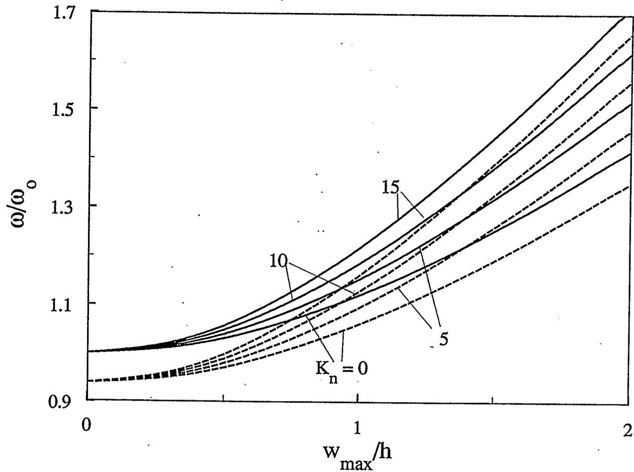
Figure 4.35: Effect of nonlinear Winkler foundation parameter on the frequency-amplitude response of an elastically supported three-layer boron-epoxy circular plate
