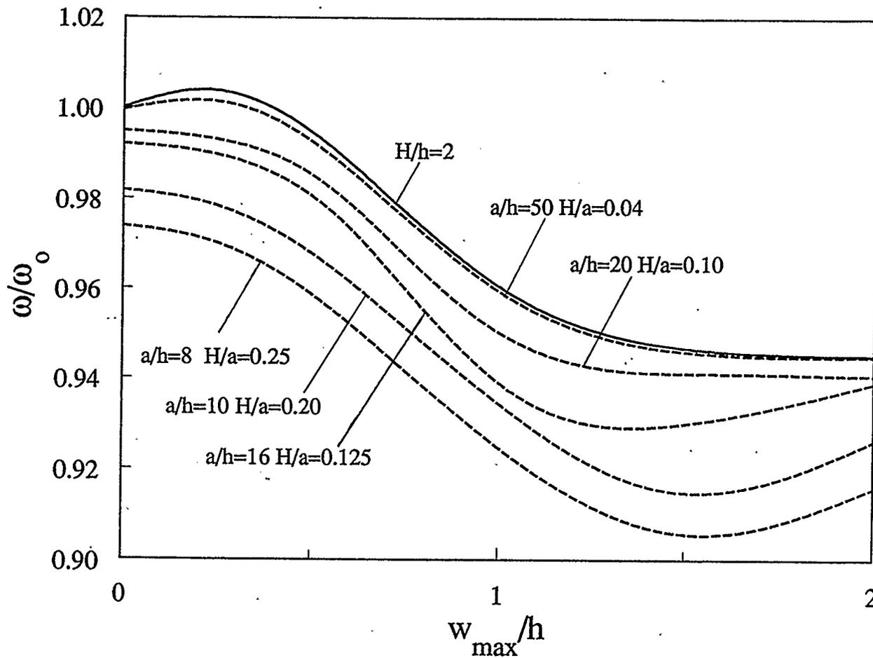
Figure 4.12: Effect of the base radius-to-thickness ratio on the frequency-amplitude response of an immovable clamped five-layer boron-epoxy shallow spherical shell resting on elastic foundation ( $\bar{W}_1=0.2$ ,  $K_f=10$ ,  $K_n=10$ ,  $G_f=5$ )
