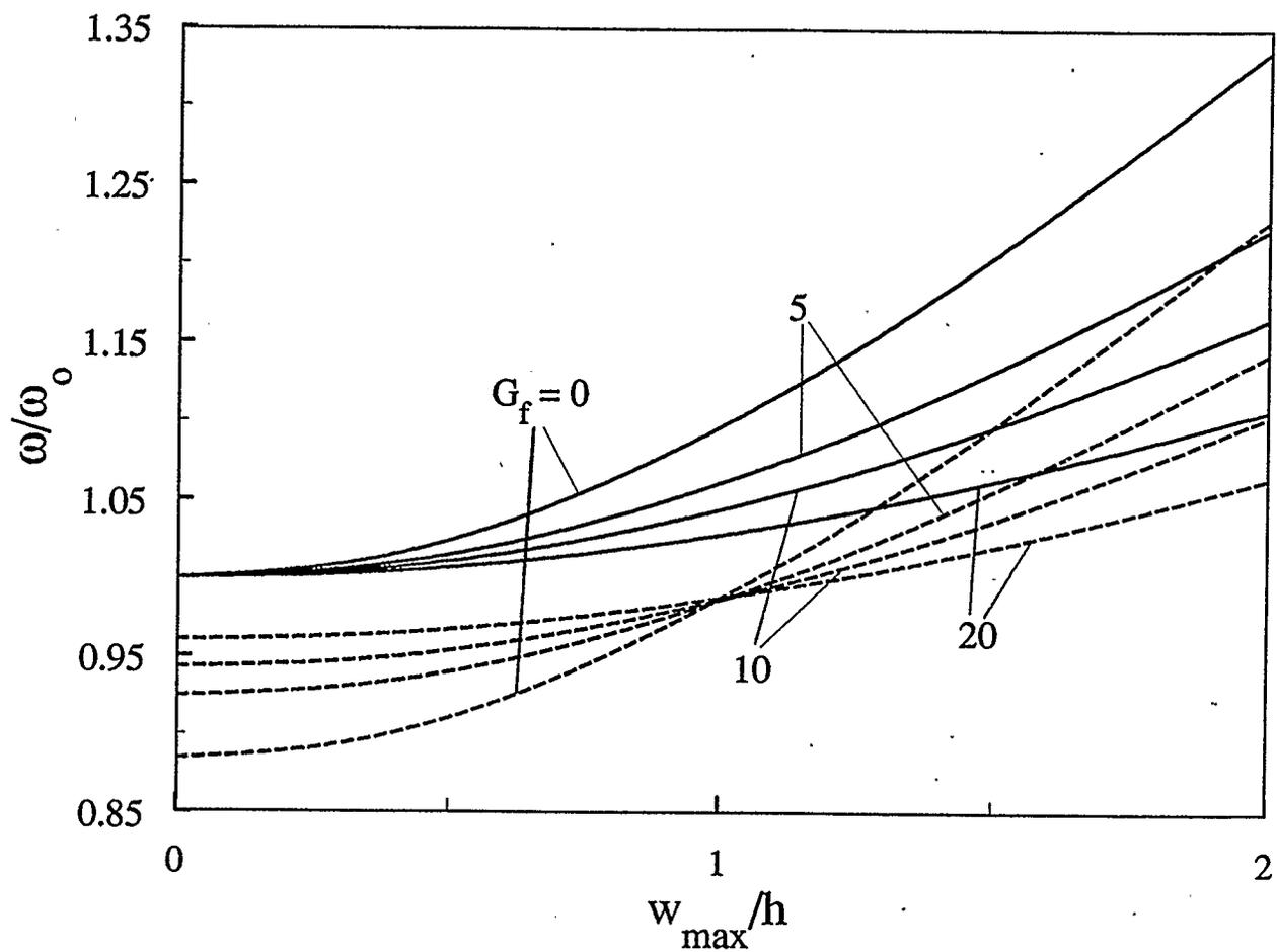
Figure 4.34: Effect of Pasternak foundation parameter on the frequency-amplitude response of a movable clamped five-layer graphite-epoxy imperfect circular plate shell
