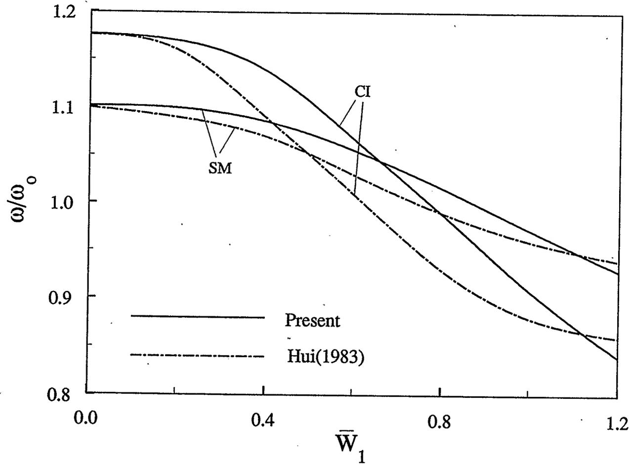
Figure 4.4: Comparison of the effect of geometric imperfections on the frequency ratio at  $w_{\max}/h=1$  of immovable clamped and movable simply-supported isotropic circular plates ( $\nu_{\theta r}=0.3$ )
