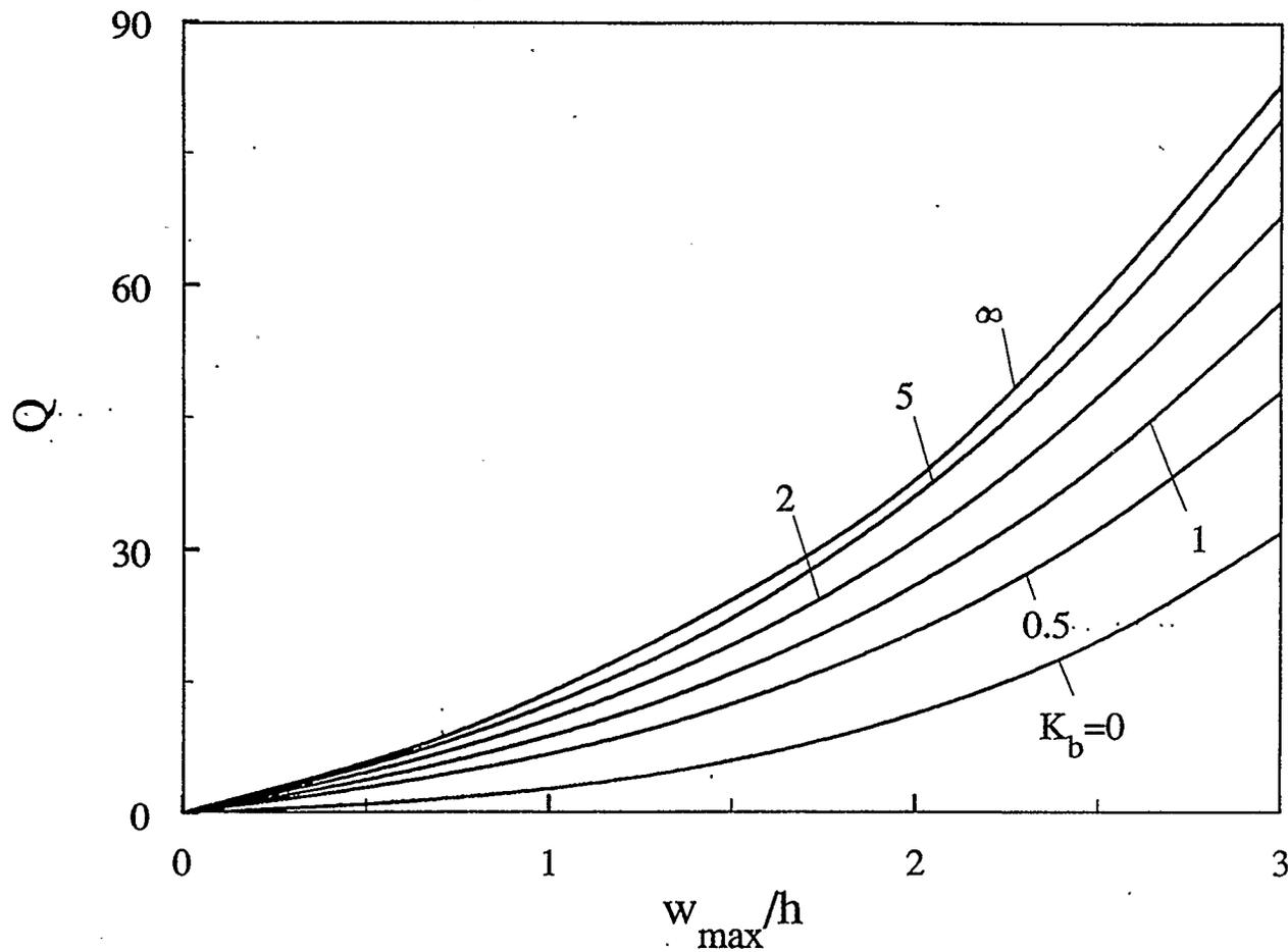
Figure 4.71: Effect of rotational edge stiffness on the static large-deflection response of a two-layer glass-epoxy circular plate with a movable edge (  $a/h=20$  )
