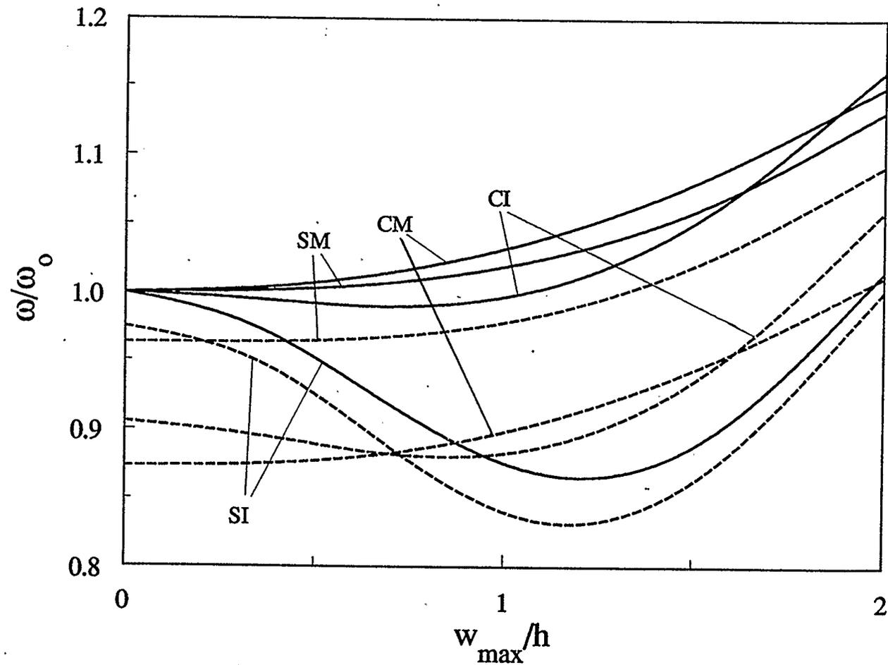
Figure 4.19: Effect of boundary conditions on the frequency-amplitude response of a five-layer graphite-epoxy imperfect shallow spherical shell resting on elastic foundations ( $\bar{W}_1=0.3, K_f=2, K_n=2, G_f=1, a/h=10, H/a=0.1$ )
