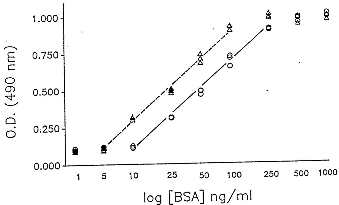
Figure 3. The effect of changing buffer composition on sample optical density. Samples diluted in the assay buffer ( $\Delta$ -- $\Delta$ ) are compared with samples diluted in Ussing chamber buffer ( $O$ — $O$ ).
