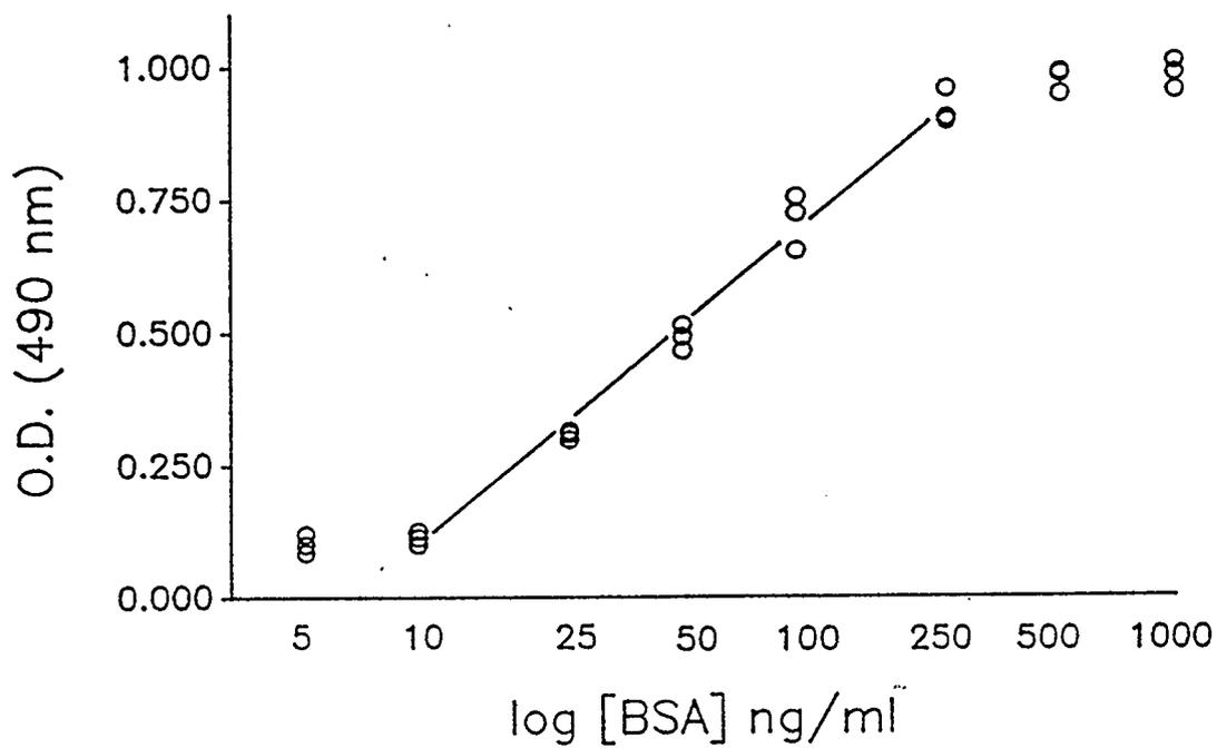
Figure 2. A representative BSA ELISA standard curve. The log of BSA concentration is plotted against optical density for triplicate BSA standards. The linear regression has been plotted for the linear portion of the curve.
