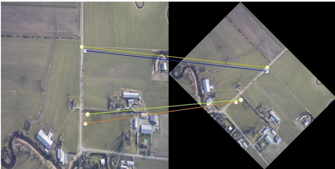
Figure A 14: Descriptor length 36 with scale variation = 0.8 and rotation = 45 and number of sample points 5x5
