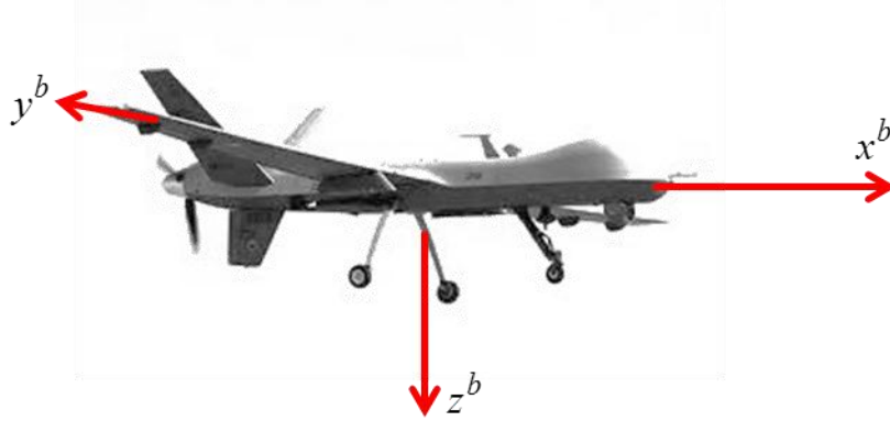
Figure 2.3: UAV body frame.
