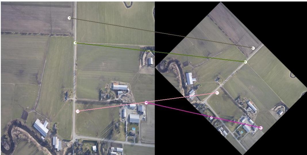
Figure A 10: Descriptor length 64 with scale variation = 1 and rotation = 45 and number of sample points 5x5
