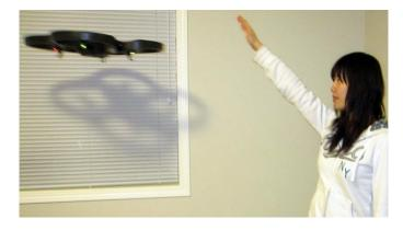
Figure 1. Using a gesture to tell the A.R. Drone to fly higher.
