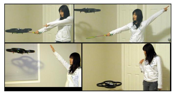
Figure 3. (Top) A user doing the *takeoff* gesture with a badminton racquet as the takeoff pad. (Bottom left) Making a raising gesture. (Bottom right) Making a *come* gesture.
