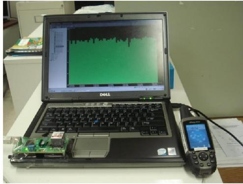
**Figure 6-5 Wi-Fi+GPS+IMU prototype system**
