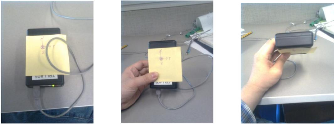
(a) Orientation 1: horizontal    (b) Orientation 2: 45° pitch    (c) Orientation 3: -45° pitch
