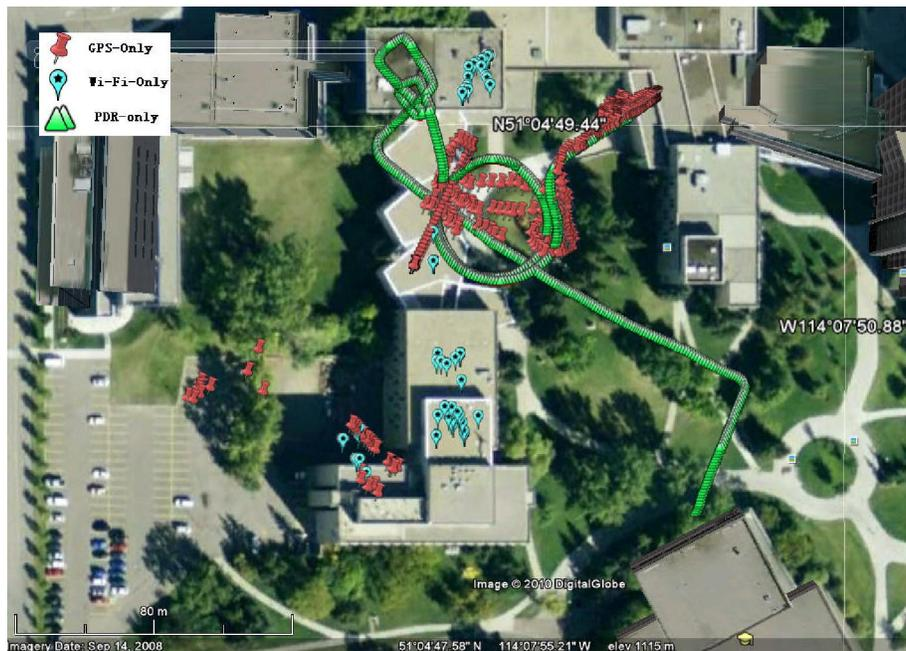
**Figure 6-6 Comparison of GPS/Wi-Fi/PDR stand-alone solutions**
