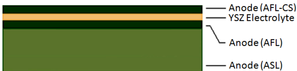
Figure 3.2. Schematic diagram of ASC-2 samples that contain an ASL, AFL, YSZ electrolyte and another AFL on the counter electrode side of the cell.
