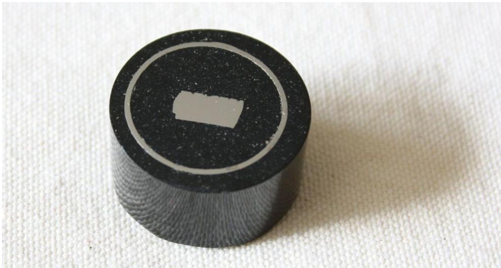
**Figure 4-3 Mounted Metallurgical Sample of SCC Affected Pipeline, 32 mm Diameter**
