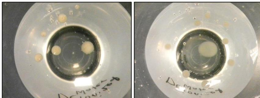
Figure 3.8 Dilution test for emulsions where rev dust initially was added to Neodrill oil (left) water with pH 12.5 (right) and. The test indicated that emulsions are still invert even though 5 ml of deionized water was added.
