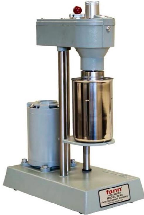
Figure 2.3 Fann Model 35 viscometer is a direct reading instrument used to measure rheological properties in six-speed designs. The sample is added to the steel cup and placed under the sleeve.
