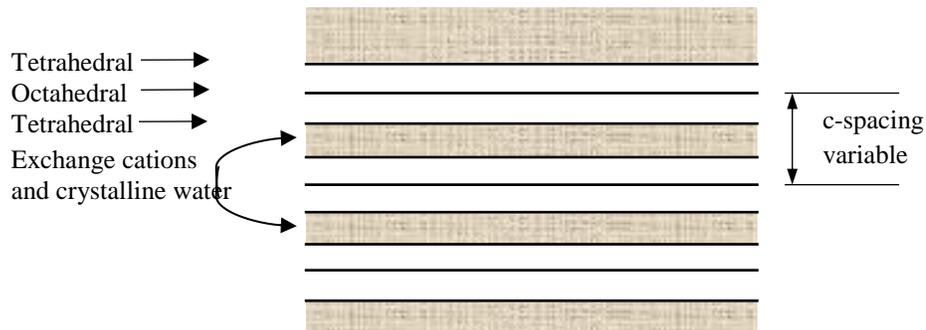
Figure 1.3 Diagrammatic representation of 3-layer expanding clay lattice [34]. The absorption of water molecules on crystal surface greatly increases c-spacing, the distance between a plane in one layer and the corresponding layer in the next layer.
