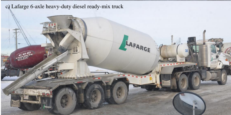
Figure 5-6 Typical HDDVs used to deliver ready-mix concrete
