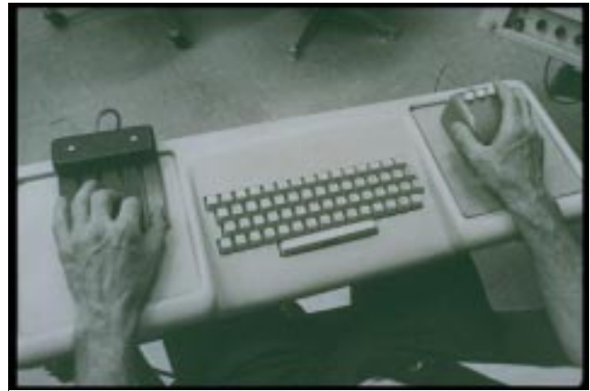
Figure 8. Engelbart's mouse-keyset combination, including a one-handed chorded keyboard (from www.bootstrap.org )
