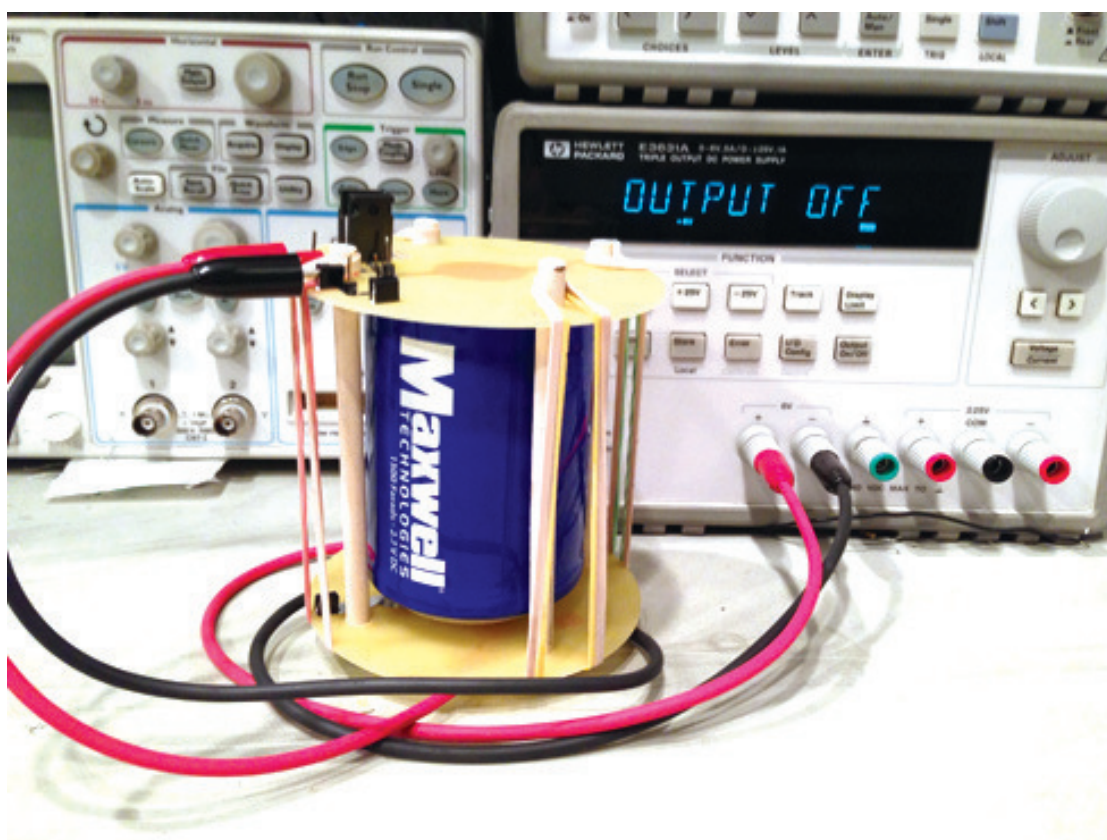
Figure D.2: BCAP1500-P270-K05 supercapacitor from Maxwell Technologies Inc. installed between the high capacity supercapacitor test PCBs.
