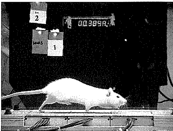
Fig. 3. Rats broke an infrared beam of light to trigger the data acquisition system and LED timer just prior to crossing the force platforms. All rats used a symmetrical trotting gait where diagonal limb pairs alternate.
