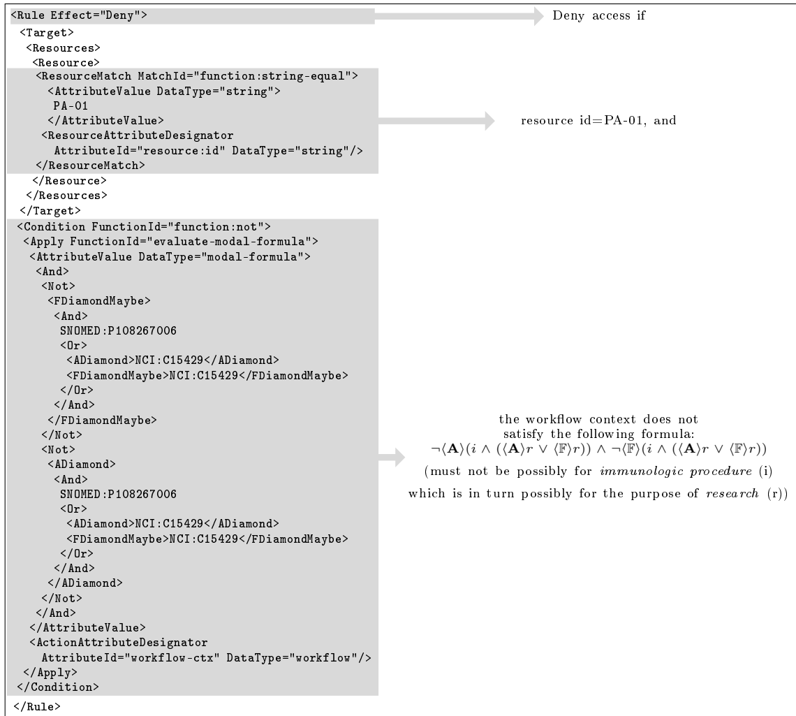
Figure 9.3: A sample consent directive formulated in XACML 2.0; the policy says that access to the specific record data is denied if it is possibly for immunologic procedure which is in turn possibly for the purpose of research activity . Note that the XACML namespaces are removed/summarized for better readability.
