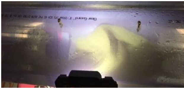
Figure 7. Sand bank after 1.2[kg] of frac sand was injected into the desander.
